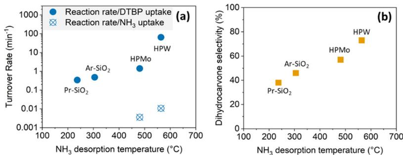
Fig. 3 Correlation of NH<sub>3</sub> desorption temperature to turnover rate (a) and dihydrocarvone selectivity (b) for solid acids (conditions: 5 °C, conversion 13–15%, reaction time 15 min, limonene oxide 225  $\mu\text{mol}$ , dimethyl carbonate 3 mL, turnover rate calculated using the DTBP uptake (●) and NH<sub>3</sub> uptake (⊗)).
