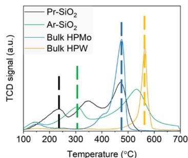
**Fig. 1** NH<sub>3</sub> TPD of solid acids (chemisorption 100 °C, NH<sub>3</sub> desorption temperatures (marked in dashed lines) were obtained considering catalyst decomposition and water removal).
