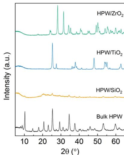
Fig. 4 XRD spectra of the heteropoly acid catalysts.
