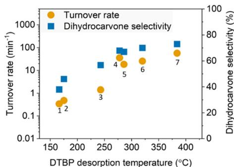
Fig. 7 Correlation of DTBP desorption temperature to the turnover rate and dihydrocarvone selectivity for solid acid catalysts: (1) Pr-SiO<sub>2</sub>, (2) Ar-SiO<sub>2</sub>, (3) bulk HPMO, (4) HPW/ZrO<sub>2</sub>, (5) HPW/TiO<sub>2</sub>, (6) HPW/SiO<sub>2</sub>, and (7) bulk HPW (Conditions: 5 °C conversion 13–15%, reaction time 15 min, limonene oxide 225  $\mu\text{mol}$ , dimethyl carbonate 3 mL, DTBP uptake used for turnover rate calculation).
