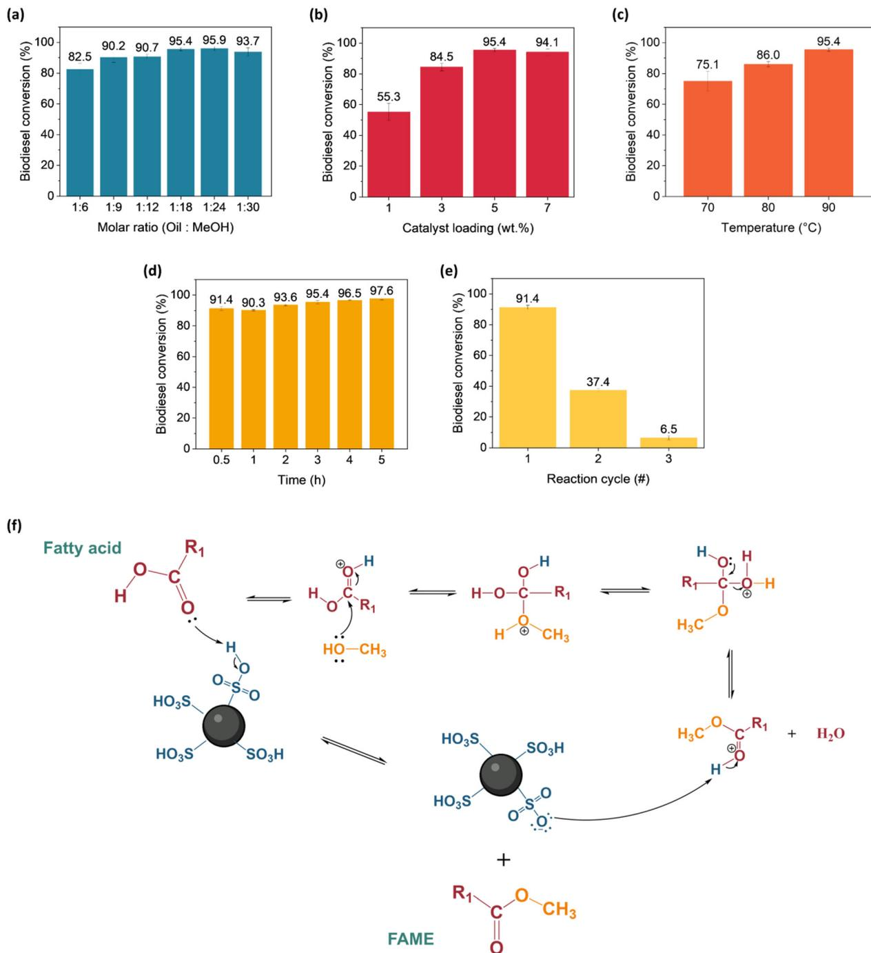
Fig. 4 (a) Reaction optimization of oil : methanol molar ratio, (b) catalyst loading (wt%), (c) temperature (°C), and (d) reaction time. (e) Reusability test of SSO<sub>3</sub>H<sub>1</sub>:1.5\_180\_20 for the esterification reaction. (f) Proposed esterification mechanism using SSO<sub>3</sub>H<sub>1</sub>:1.5\_180\_20 as a catalyst.
