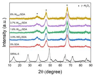
Fig. 1 XRD patterns of the SIRAL-5, 5 wt% SDA support, 3.5 wt% WO $_3$ / SDA nanoparticle catalyst prepared without the templating Zn-BTC MOF, and the various (1.6 wt%, 3.7 wt%, and 6 wt%) W $_{SAC}$ /SDA catalysts prepared using the templating Zn-BTC MOF via high-temperature pyrolysis at 1000 °C under Ar flow, followed by annealing in static air at 700 °C
