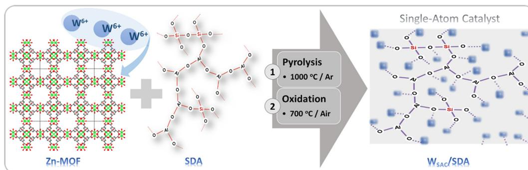
**Scheme 1** MOF-confinement of  $W^{6+}$  ions and mixing with SDA followed by pyrolysis at 1000 °C to vaporize the Zn framework and oxidation in air at 700 °C to incorporate W atoms within the SDA support.
