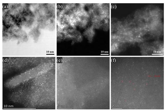
Fig. 3 (a) Dark-field and (b and c) bright-field low-resolution STEM images and (d-f) HAADF-STEM images of the 3.7 wt% W<sub>SAC</sub>/SDA catalyst.
