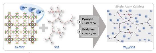
Scheme 1 MOF-confinement of W<sup>6+</sup> ions and mixing with SDA followed by pyrolysis at 1000 °C to vaporize the Zn framework and oxidation in air at 700 °C to incorporate W atoms within the SDA support.
