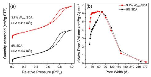
Fig. 6 (a) Nitrogen (N<sub>2</sub>) adsorption/desorption isothermal plots and (b) BJH adsorption dV/dD pore size distribution plots of the 5% SDA support and the 3.7% W<sub>SAC</sub>/SDA catalyst.
