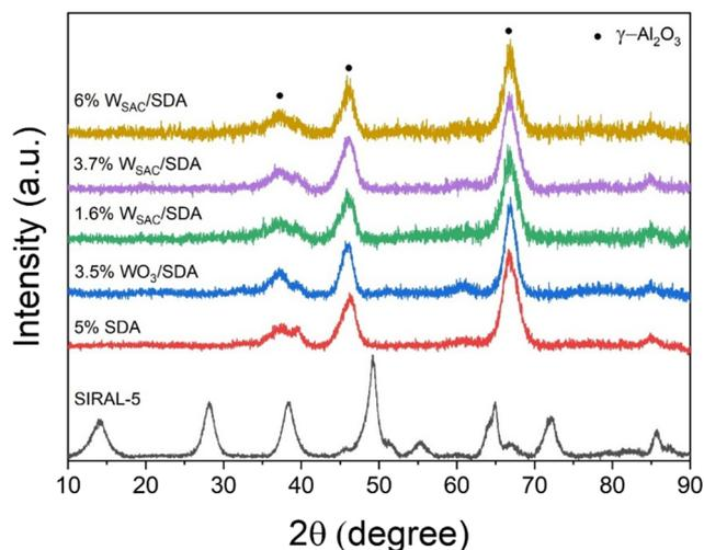
**Fig. 1** XRD patterns of the SIRAL-5, 5 wt% SDA support, 3.5 wt%  $\text{WO}_3$ /SDA nanoparticle catalyst prepared without the templating Zn-BTC MOF, and the various (1.6 wt%, 3.7 wt%, and 6 wt%)  $\text{W}_{\text{SAC}}/\text{SDA}$  catalysts prepared using the templating Zn-BTC MOF *via* high-temperature pyrolysis at 1000 °C under Ar flow, followed by annealing in static air at 700 °C.
