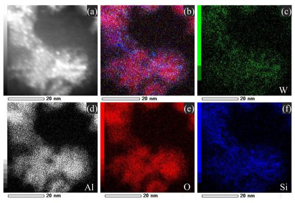
Fig. 4 (a) EDS mapping SEM image, (b) EDS layer image, and (c-f) EDS elemental mapping images of (c) tungsten, (d) aluminum, (e) oxygen, and (f) silicon of the 3.7 wt%  $W_{SAC}/SDA$  catalyst.
