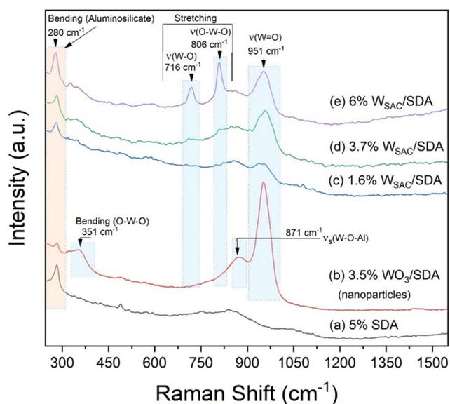
**Fig. 2** Raman spectra of (a) the SDA support prepared from SIRAL-5 at 700 °C in air for 5 h, (b) 3.5%  $\text{WO}_3$ /SDA nanoparticle catalyst prepared by a sol-gel method without using the templating Zn-MOF, and (c) 1.6 wt%, (d) 3.7 wt%, and (e) 6 wt%  $\text{W}_{\text{SAC}}/\text{SDA}$  catalysts prepared using templating Zn-BTC to confine the  $\text{W}^{6+}$  ions and incorporate the isolated  $\text{W}_1\text{-O}_3$  moieties within the SDA support.
