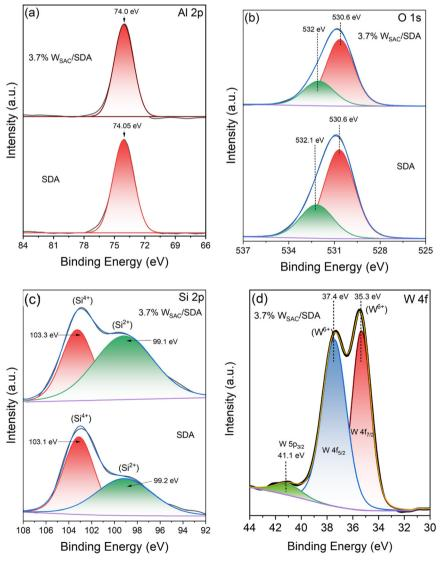
Fig. 7 High-resolution XPS spectra of (a) Al 2p, (b) O 1s, and (c) Si 2p elements of the 5% SDA support and the 3.7% W<sub>SAC</sub>/SDA catalyst, and (d) W 4f element of the 3.7%  $W_{SAC}/SDA$  catalyst.
