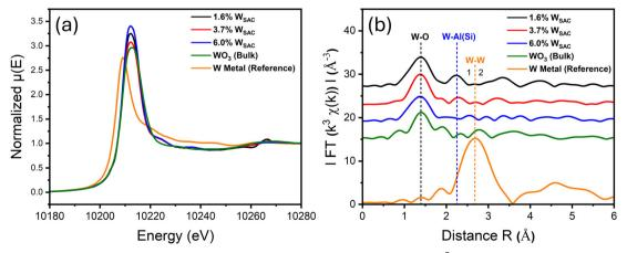
Fig. 5 (a) Normalized W L<sub>3</sub>-edge X-ray absorption near-edge structure (XANES) spectra and (b)  $k^3$ -weighted Fourier transform (FT) of the EXAFS spectra of 1.6–6.0% W<sub>SAC</sub>/SDA, bulk WO<sub>3</sub>, and reference W metal samples.
