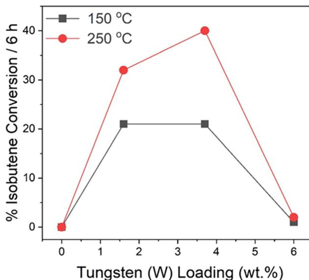
Fig. 8 Plots of % average isobutene conversion as a function of tungsten loading after 6 h at 150 °C and 250 °C under fixed GHSV and WHSV of 3000  $h^{-1}$  and 12 000  $cm^3 g^{-1} h^{-1}$ , respectively.
