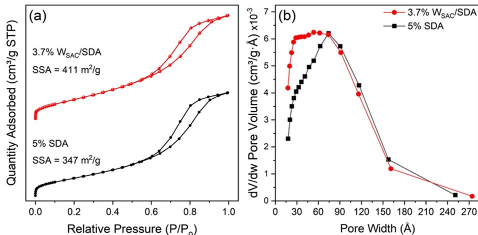
Fig. 6 (a) Nitrogen (N<sub>2</sub>) adsorption/desorption isothermal plots and (b) BJH adsorption dV/dD pore size distribution plots of the 5% SDA support and the 3.7% W<sub>SAC</sub>/SDA catalyst.
