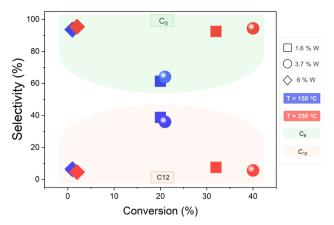
**Fig. 9** Plots of average isobutene conversion (%) *versus* selectivity (%) toward  $C_8$  and  $C_{12}$  olefins produced using  $W_{SAC}/SDA$  catalysts (1.6%, 3.7%, and 6% W) following 6 h of isobutene oligomerization at 150 °C and 250 °C under fixed GHSV and WHSV of 3000 h<sup>-1</sup> and 12000 cm<sup>3</sup> g<sup>-1</sup> h<sup>-1</sup>, respectively.
