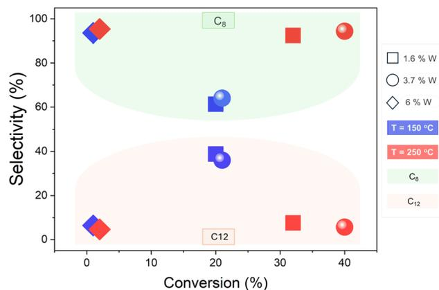
Fig. 9 Plots of average isobutene conversion (%) versus selectivity (%) toward  $C_8$  and  $C_{12}$  olefins produced using  $W_{SAC}/SDA$  catalysts (1.6%, 3.7%, and 6% W) following 6 h of isobutene oligomerization at 150 °C and 250 °C under fixed GHSV and WHSV of 3000  $h^{-1}$  and 12000  $cm^3 g^{-1} h^{-1}$ , respectively.
