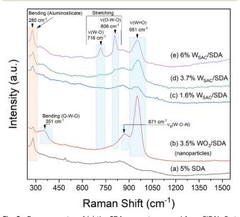
Fig. 2 Raman spectra of (a) the SDA support prepared from SIRAL-5 at 700  $^{\circ}\text{C}$  in air for 5 h, (b) 3.5% WO<sub>3</sub>/SDA nanoparticle catalyst prepared by a sol–gel method without using the templating Zn-MOF, and (c) 1.6 wt%, (d) 3.7 wt%, and (e) 6 wt% W<sub>SAC</sub>/SDA catalysts prepared using templating Zn-BTC to confine the W<sup>6+</sup> ions and incorporate the isolated W<sub>1</sub>–O<sub>3</sub> moieties within the SDA support.
