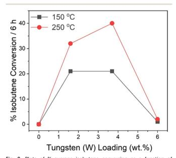
Fig. 8 Plots of % average isobutene conversion as a function of tungsten loading after 6 h at 150 °C and 250 °C under fixed GHSV and WHSV of 3000  $h^{-1}$  and 12 000 cm<sup>3</sup> g<sup>-1</sup>  $h^{-1}$ , respectively.
