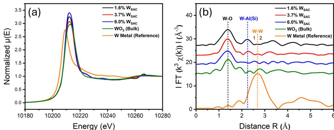
Fig. 5 (a) Normalized W  $L_3$ -edge X-ray absorption near-edge structure (XANES) spectra and (b)  $k^3$ -weighted Fourier transform (FT) of the EXAFS spectra of 1.6–6.0%  $W_{SAC}/SDA$ , bulk  $WO_3$ , and reference W metal samples.
