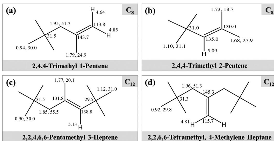
Fig. 10 Structures and chemical shifts of  $\text{C}_8$  and  $\text{C}_{12}$  olefin products as determined by NMR for (a) 2,4,4-trimethyl-1-pentene, (b) 2,4,4-trimethyl-2-pentene, (c) 2,2,4,6,6-pentamethyl-3-heptene, and (d) 2,2,6,6-tetramethyl-4-methylene heptane obtained from isobutene conversion over  $W_{\text{SAC}}/\text{SDA}$  catalysts.
