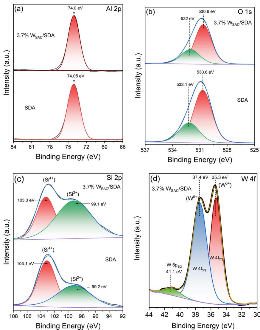
Fig. 7 High-resolution XPS spectra of (a) Al 2p, (b) O 1s, and (c) Si 2p elements of the 5% SDA support and the 3.7% W<sub>SAC</sub>/SDA catalyst, and (d) W 4f element of the 3.7% W<sub>SAC</sub>/SDA catalyst.
