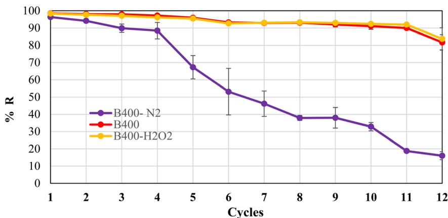
**Fig. 12** Long-term removal stability (24 hours) in the removal efficiency of B400, B400- $H_2O_2$  and B400- $N_2$  (non-activated biochar). 10 mL MB solution was recycled for 2 hours-cycles for a total of 12 cycles (MB  $2.5 \times 10^{-5}\ mol\ L^{-1}$ ).
