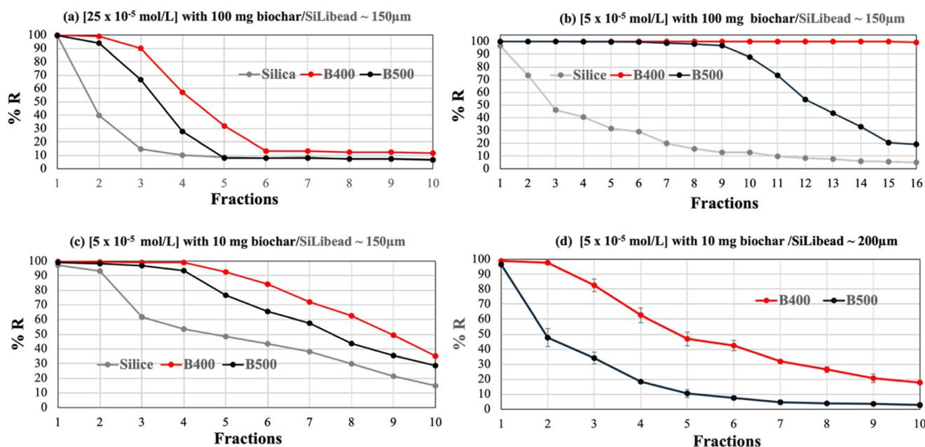
**Fig. 11** Percentage removal (% R) of MB in different experimental conditions as reported in Table 1: type and mass of biochar, granulometry of SiLibeads® as supports, concentration and volume of MB solution are indicated in each panel.
