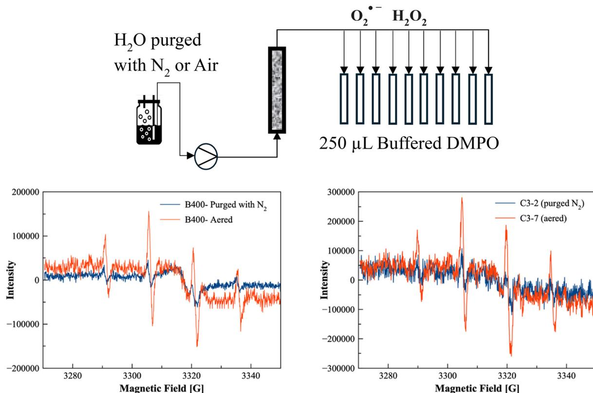
Fig. 14 (Left) EPR spectra of  $\text{DMPO}^{\bullet}\text{-OH}$  generated into B400 suspensions aerated and not, batch mode. (Right) EPR spectra of  $\text{DMPO}^{\bullet}\text{-OH}$  generated in the vial containing DMPO solution and the purged water percolated through a B400-based bed-packed column dropped into it.
