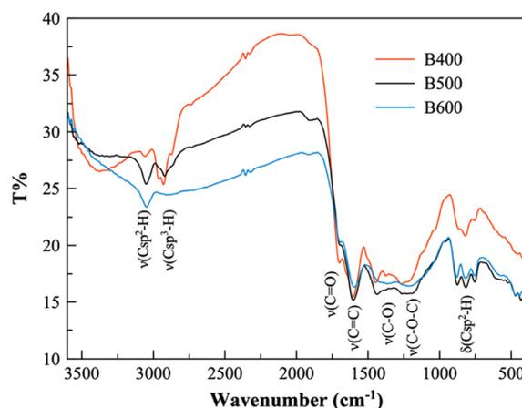
**Fig. 2** DRIFTS analysis of pyrolyzed samples B400–B600.
