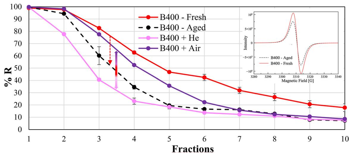
**Fig. 13** % removal of MB in continuous flow (100 mL,  $5 \times 10^{-5}$  mol L $^{-1}$ ) of three column-packed systems with different concentrations of dissolved oxygen in contact with B400: B400-fresh (red line); B400-aged (black dashed line); B400-insufflated He (pink line) and B400-insufflated with air (O $_2$ ) (purple line). The insert reports the EPR spectra of B400-fresh and B400-aged samples.
