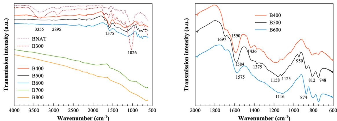
**Fig. 1** ATR-FT-IR analysis of natural bamboo (BNAT) and pyrolyzed samples B300–B800 (left panel). Magnification of ATR-FT-IR spectra of B400, B500 and B600 (right panel) in the 600–2000  $\text{cm}^{-1}$  region. In the images only the most representative bands are indicated.
