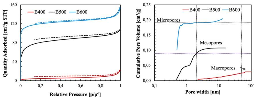
**Fig. 9** (Left) N<sub>2</sub> adsorption (full lines) and desorption (dashed lines) isotherm for BAC (B400, B500 and B600). (Right) DFT analysis for cumulative pore volume of BAC.
