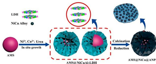
Fig. 8 Synthetic procedure for AMS@NiCu@ANPs through transformation of the AMS@NiCuAl-LDH precursor [panel has been reproduced with permission from ref. 126, Copyright 2019, American Chemical Society].
