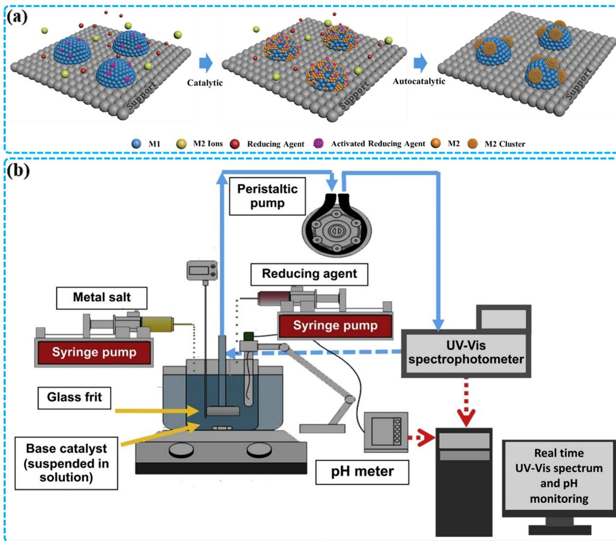
Fig. 11 (a) Electroless deposition method for supported-bimetallic catalyst synthesis with the catalytic process and autocatalytic process; (b) schematic illustration of the continuous ED procedure [panel (b) has been reproduced with permission from ref. 153, Copyright 2019, Elsevier].
