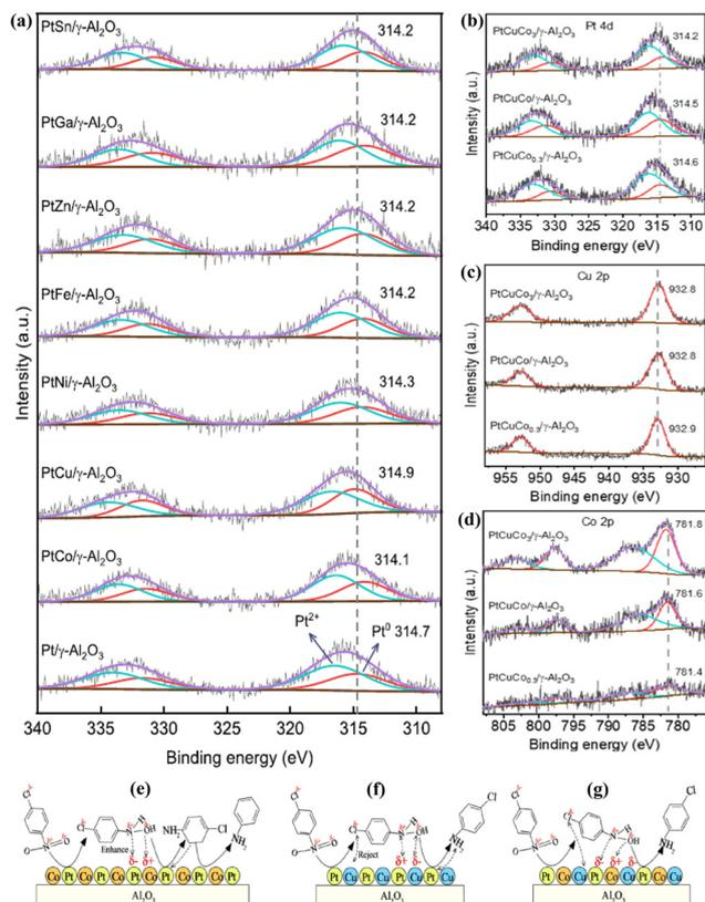
**Fig. 3** (a) Pt 4d XPS spectra for PtM/γ-Al<sub>2</sub>O<sub>3</sub> catalysts; XPS spectra of (b) Pt 4d, (c) Cu 2p, and (d) Co 2p for PtCuCo<sub>x</sub>/γ-Al<sub>2</sub>O<sub>3</sub> catalysts; proposed mechanism for the selective hydrogenation of *p*-CNB on (e) PtCo/γ-Al<sub>2</sub>O<sub>3</sub>, (f) PtCu/γ-Al<sub>2</sub>O<sub>3</sub>, and (g) PtCuCo<sub>x</sub>/γ-Al<sub>2</sub>O<sub>3</sub> catalysts [panels (a–g) have been reproduced with permission from ref. 64, Copyright 2023, Elsevier].
