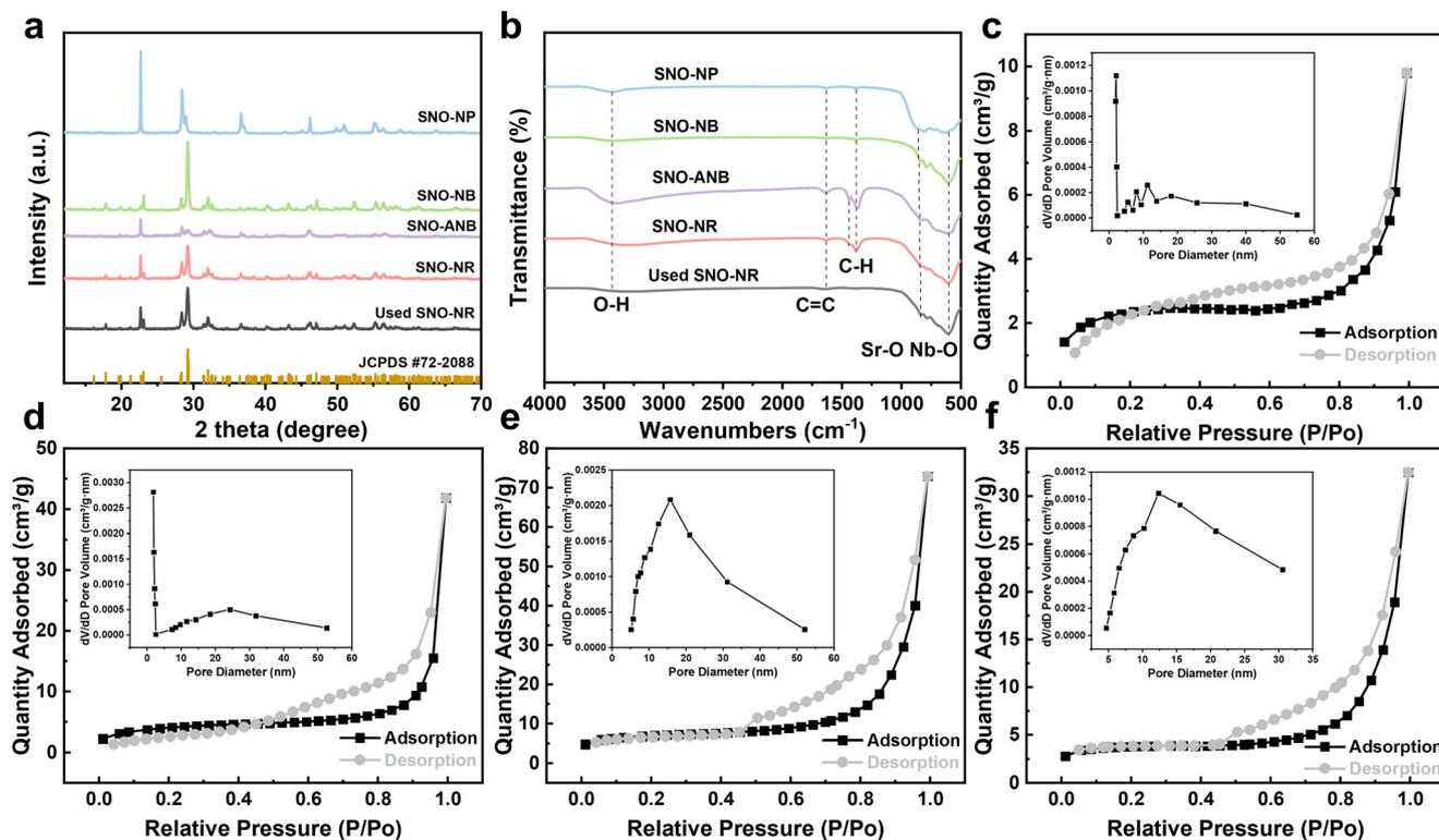
Fig. 2 (a) XRD patterns and (b) FT-IR profiles of all the SNO catalysts including the spent SNO-NR. The N<sub>2</sub> adsorption-desorption isotherms of (c) SNO-NP, (d) SNO-NB, (e) SNO-ANB, and (f) SNO-NR, respectively.
