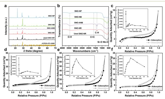
Fig. 2 (a) XRD patterns and (b) FT-IR profiles of all the SNO catalysts including the spent SNO-NR. The  $N_2$  adsorption-desorption isotherms of (c) SNO-NP, (d) SNO-NB, (e) SNO-ANB, and (f) SNO-NR, respectively.
