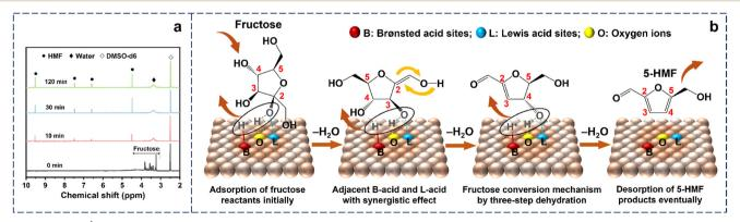
Fig. 6 (a) In situ <sup>1</sup>H NMR spectra as a function of time for the dehydration of 4 wt% fructose catalyzed by SNO-NR in DMSO-d<sub>6</sub> at 120 °C. (b) Proposed reaction mechanism for the SNO-catalyzed dehydration of fructose to HMF.
