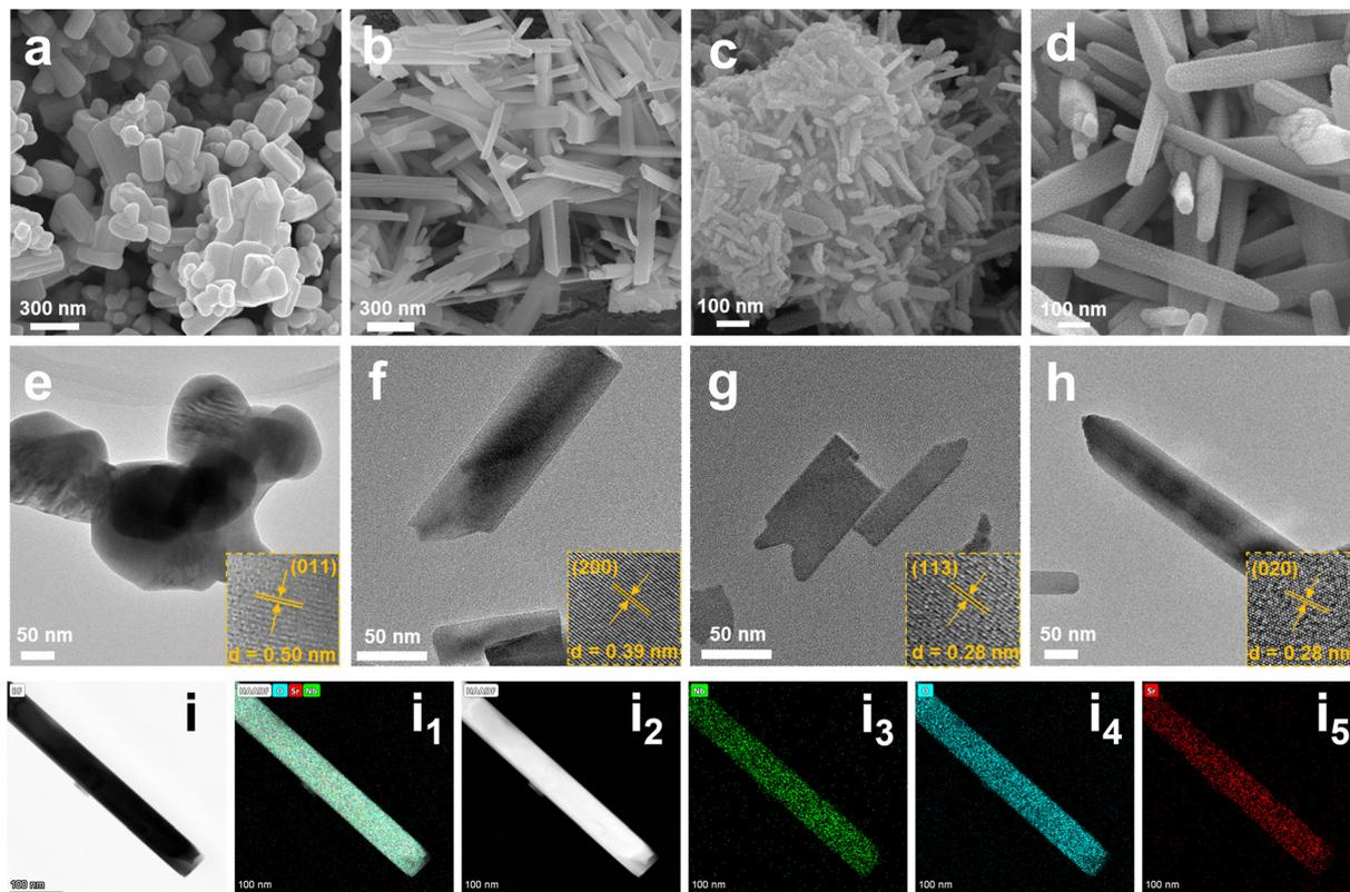
**Fig. 3** FESEM images of (a) SNO-NP, (b) SNO-NB, (c) SNO-ANB, and (d) SNO-NR, respectively. (e–h) TEM images of these SNO nanomaterials accordingly as well as their magnification. (i–i5) TEM mapping images of SNO-NR.
