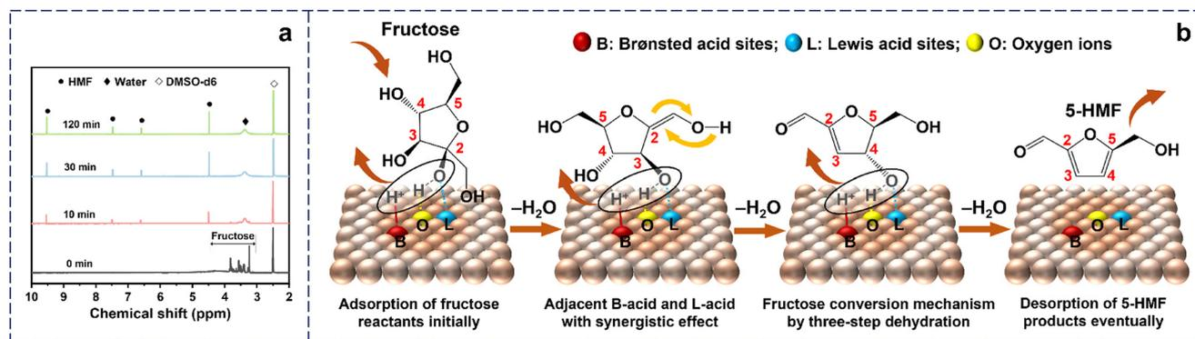
Fig. 6 (a) *In situ*  $^1\text{H}$  NMR spectra as a function of time for the dehydration of 4 wt% fructose catalyzed by SNO-NR in  $\text{DMSO-}d_6$  at  $120\text{ }^\circ\text{C}$ . (b) Proposed reaction mechanism for the SNO-catalyzed dehydration of fructose to HMF.
