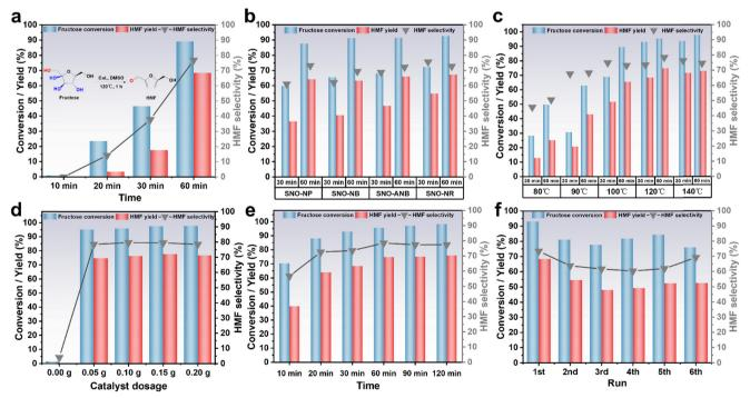
Fig. 5 Catalytic performance of various catalysts: (a)  $Nb_2O_5$  and (b) SNO catalysts with various morphologies. Effects of (c) reaction temperature, (d) catalyst dosage, and (e) reaction time on the dehydration of fructose to HMF over SNO-NR. (f) Recycle tests over SNO-NR. Reaction conditions: 4 wt% fructose solution (5 mL DMSO), 120 °C, 60 min, 0.05 g catalyst except for (b) 110 °C, (c) 80-140 °C, (d) 0.00-0.20 g catalyst, (e) 10-120 min, and (f) 30 min.
