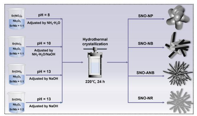
Fig. 1 Schematic illustration for the synthetic process of various SrNb<sub>2</sub>O<sub>6</sub> nanocatalysts
