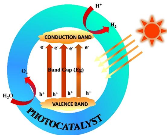
Scheme 2 Schematic representation of photocatalytic hydrogen evolution.
