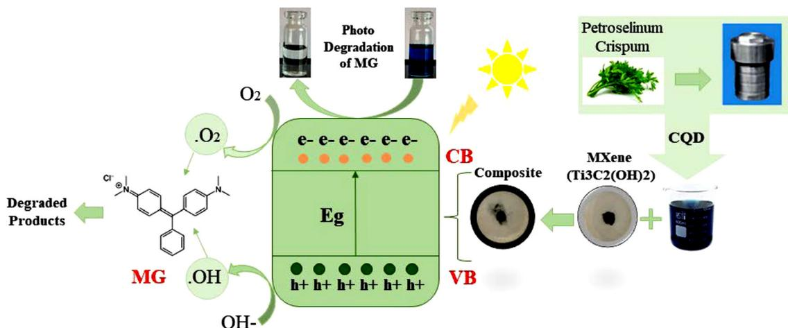
Fig. 13 An illustration of the photocatalytic pathway for MG degradation by the CQDs/MXene nanocomposite. Reproduced from ref. 104 with permission from Elsevier, copyright 2024.
