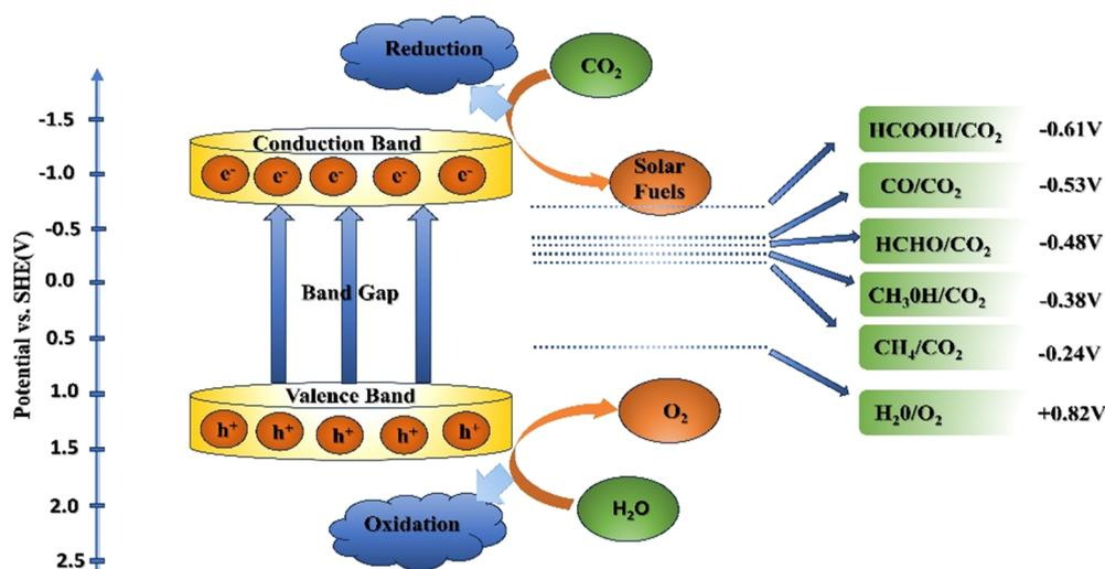
Scheme 3 Schematic representation of carbon dioxide reduction.
