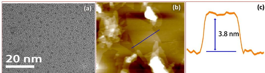
Fig. 3 (a) TEM image of  $\text{TiO}_2$  QDs, (b) height profile characterized by AFM, and (c) the corresponding height distribution. Reproduced from ref. 73 with permission from Elsevier, copyright 2021.
