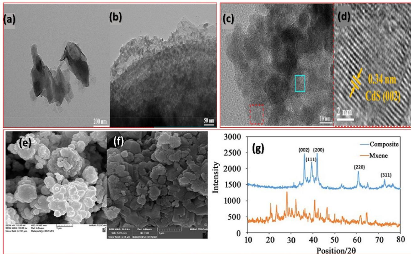
Fig. 8 TEM images of (a)  $\text{Ti}_3\text{C}_2\text{T}_x$  and (b) CT-9 and (c and d) HRTEM images of CT-9.<sup>103</sup> SEM images of (e) MXene (left) and (f) nanocomposite (right); (g) XRD patterns. Reproduced from ref. 104 with permission from American Chemical Society, copyright 2023.
