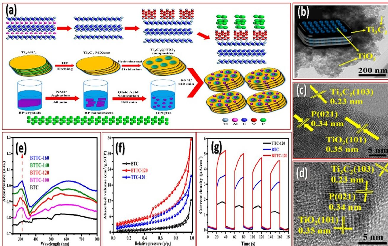
Fig. 1 (a) Schematic illustration of the preparation of BPQDs/Ti<sub>3</sub>C<sub>2</sub>@TiO<sub>2</sub> composites, (b–d) HRTEM images of the BTTC-120 sample, (e) UV-vis diffuse reflectance spectra (DRS) of as-synthesized BTC and BTTC-*x* (*x* = 100, 120, 140, and 160 °C, respectively), (f) N<sub>2</sub> adsorption–desorption isotherms of the as-prepared BTC, TTC-120, and BTTC-120 powders, and (g) photocurrent response. Reproduced from ref. 77 with permission from MDPI, copyright 2020.
