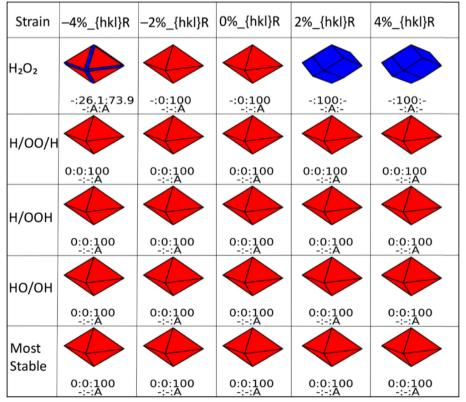
Fig. 5 CeO<sub>2</sub> nanoparticle shapes of dissociatively and associatively adsorbed hydrogen peroxide on CeO<sub>2</sub> (100), (110) and (111) surfaces. Red, blue and green represent the (111), (110) and (100) CeO<sub>2</sub> surfaces, respectively. The nanoparticle shapes are generated at 1 bar and 298 K. Each shape is characterized by a ratio of surfaces defined in numerical percentage ((100): (110): (111)). The label B defines a bare surface and A means adsorbed.
