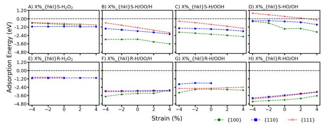
Fig. 2 Adsorption energy of H<sub>2</sub>O<sub>2</sub> on stoichiometric/reduced CeO<sub>2</sub> {100}, {110}, and {111} surfaces as a function of strain: molecular (A and E) H<sub>2</sub>O<sub>2</sub> and dissociative (B and F) H/OO/H, (C and G) H/OOH, and (D and H) HO/OH adsorption hydrogen peroxide.
