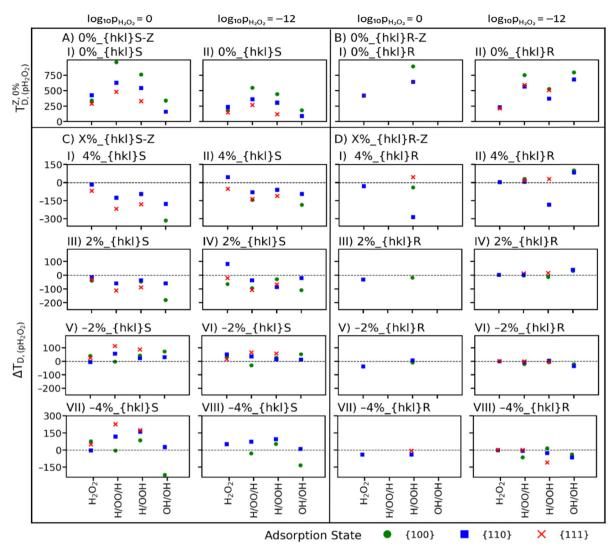
Fig. 3 Desorption temperature of molecularly and dissociatively adsorbed hydrogen peroxide on stoichiometric and oxygen-deficient CeO<sub>2</sub>.  $T_{D,(\rho_{12}O_2)}^{N,0\%}$  of adsorbed hydrogen peroxide species on unstrained stoichiometric (A) and oxygen-deficient (B) CeO<sub>2</sub> surfaces.  $\Delta T_{D,(\rho_{12}O_2)}$  of adsorbed hydrogen peroxide species on strained stoichiometric (C) and oxygen-deficient (D) CeO<sub>2</sub> surfaces.
