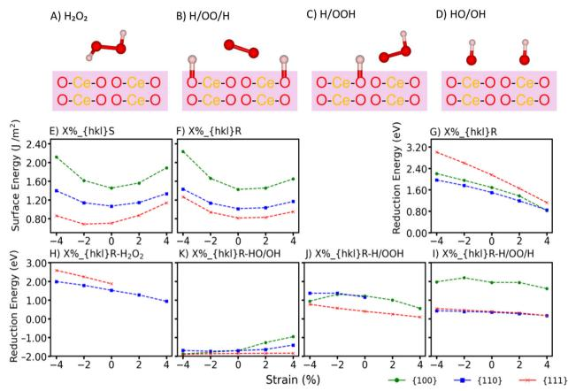
Fig. 1 Schematics of (A) molecular H<sub>2</sub>O<sub>2</sub> and dissociative (B) H/OO/H, (C) H/OOH, and (D) HO/OH adsorption states on ceria surfaces. Surface energies of (E) stoichiometric and (F) reduced CeO2 under compression (negative) and tensile (positive) strain. Reduction energies of reduced CeO2 surfaces as a function of strain: (G) bare; (H) molecular H<sub>2</sub>O<sub>2</sub>; and dissociative (I) H/OO/H, (J) H/OOH and (K) HO/OH hydrogen peroxide.
