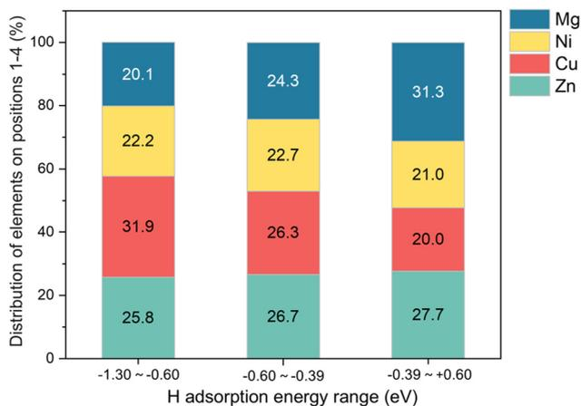
**Fig. 8** Percent distribution among the four metal elements at positions 1-4 for different HAE ranges. Positions 1-4 refer to the four nearest metal neighbors of the O site on the surface (see Fig. 1c).
