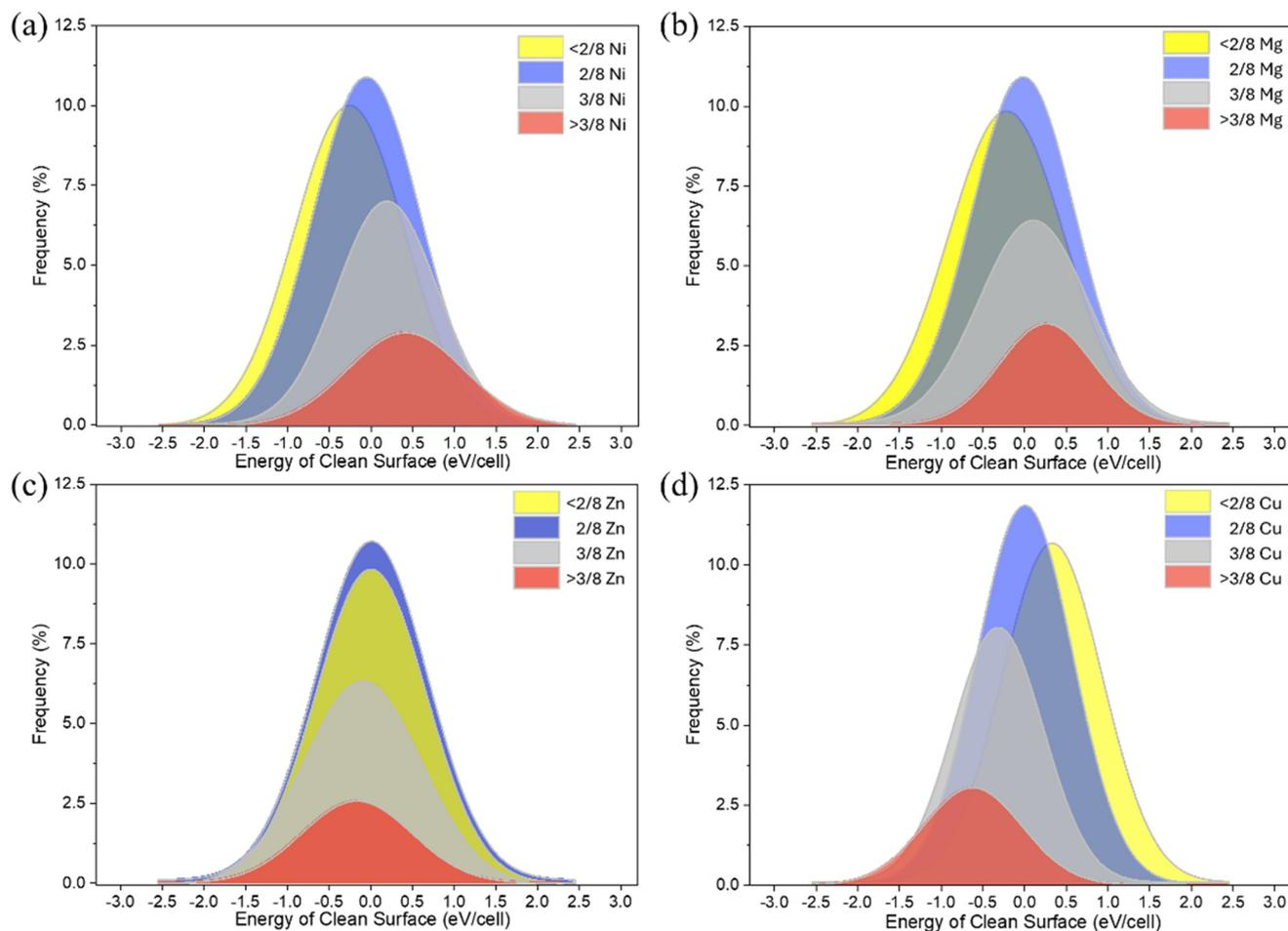
Fig. 3 Distributions of the relative energies (eV per cell) of the 2000 clean (100) surfaces of  $\text{Mg}_{0.25}\text{Ni}_{0.25}\text{Cu}_{0.25}\text{Zn}_{0.25}\text{O}$  for different surface concentrations of metal cations: (a) Ni; (b) Mg; (c) Zn; (d) Cu.
