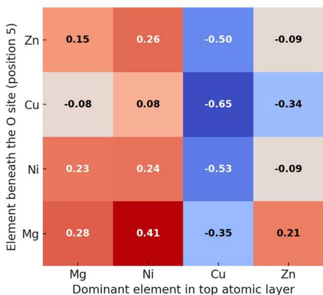
Fig. 6 Average relative energies (in eV per cell) of the 2000 H-adsorbed surfaces of  $\text{Mg}_{0.25}\text{Ni}_{0.25}\text{Cu}_{0.25}\text{Zn}_{0.25}\text{O}$  as a function of the position-5 element (y-axis) and the dominant surface element (x-axis). Position-5 refers to the metal element directly beneath the O site where H adsorbs (see Fig. 1c).
