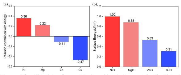
Fig. 4 (a) Pearson correlation coefficients between the energy of the surface and the surface-layer concentration of a metal atom for the 2000  $Mg_{0.25}Ni_{0.25}Cu_{0.25}Cn_{0.25}C$  (100) surfaces; (b) computed (100) surface energies (J m $^{-2}$ ) of different rock-salt metal oxides.
