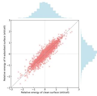
Fig. 5 Correlation between the relative energies of clean surfaces and H-adsorbed surfaces for the 2000 (100) surfaces of Mg<sub>0.25</sub>Ni<sub>0.25</sub>Cu<sub>0.25</sub>- $Zn_{0.25}O. R^2 = 0.85.$
