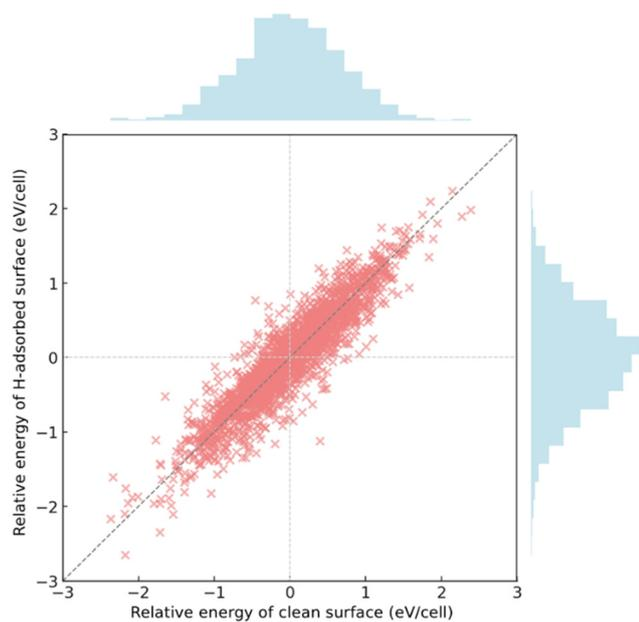
Fig. 5 Correlation between the relative energies of clean surfaces and H-adsorbed surfaces for the 2000 (100) surfaces of  $\text{Mg}_{0.25}\text{Ni}_{0.25}\text{Cu}_{0.25}\text{Zn}_{0.25}\text{O}$ .  $R^2 = 0.85$ .
