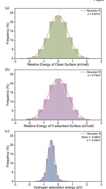
Fig. 2 Distributions of DFT-computed energies of the 2000 Mg<sub>0.25</sub>- $Ni_{0.25}Cu_{0.25}Zn_{0.25}O$  (100) surfaces: (a) energy of the clean surface relative to the mean (eV per cell; each cell has 80 atoms); (b) energy of the H-adsorbed surface relative to the mean (eV per cell; each cell has 80 atoms plus 1 H atom); (c) hydrogen adsorption energy (eV, in reference to  $\frac{1}{2}$  H<sub>2</sub>; H coverage: 1.4 nm<sup>-2</sup>).
