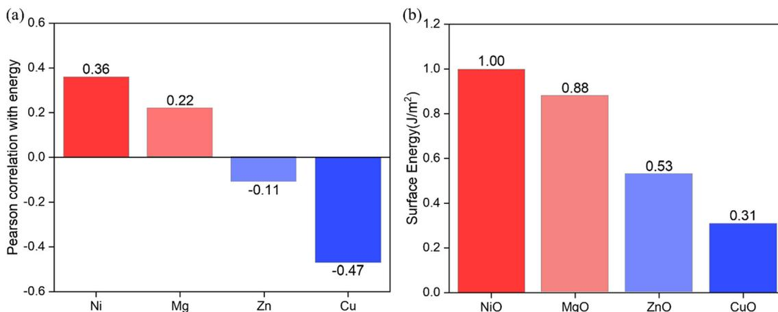
Fig. 4 (a) Pearson correlation coefficients between the energy of the surface and the surface-layer concentration of a metal atom for the 2000  $\text{Mg}_{0.25}\text{Ni}_{0.25}\text{Cu}_{0.25}\text{Zn}_{0.25}\text{O}$  (100) surfaces; (b) computed (100) surface energies ( $\text{J m}^{-2}$ ) of different rock-salt metal oxides.
