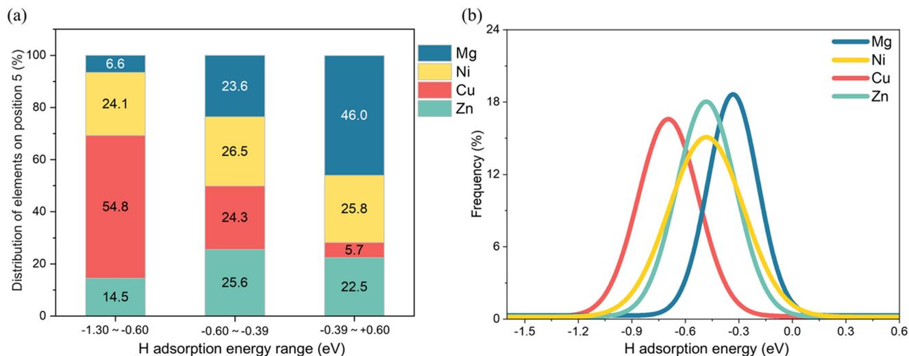
**Fig. 7** Relationship between the H adsorption strength and the metal element: (a) Percent distribution among the four metal elements at position 5 for different HAE ranges; (b) distribution of HAEs for a given metal element at position 5 which refers to the metal site directly beneath the O site where H adsorbs (see Fig. 1c).
