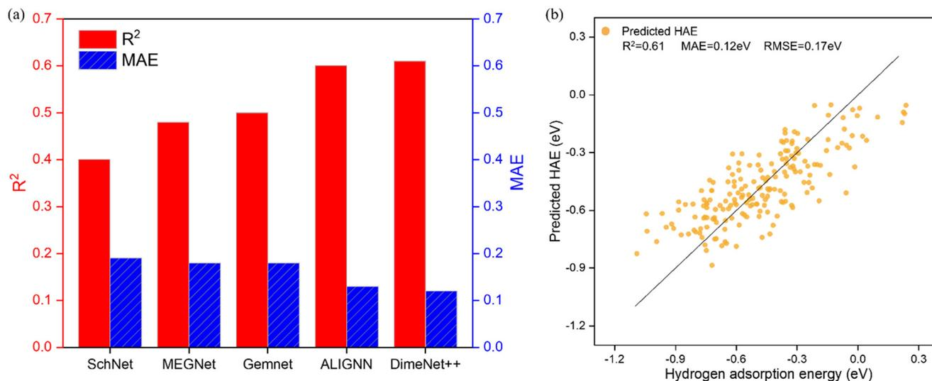
Fig. 9 (a) Comparison of different machine-learning models trained on DFT-computed HAEs on 2000  $\text{Mg}_{0.25}\text{Ni}_{0.25}\text{Cu}_{0.25}\text{Zn}_{0.25}\text{O}$  (100) surfaces: left axis, coefficient of determination; right axis, mean absolute error (MAE). (b) Parity plot for the DimeNet++ based on the 10% held-out test set.
