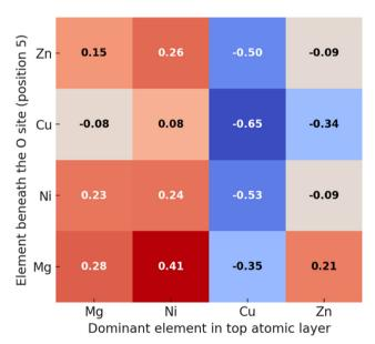
Fig. 6 Average relative energies (in eV per cell) of the 2000 H-adsorbed surfaces of Mg<sub>0,25</sub>Ni<sub>0,25</sub>Cu<sub>0,25</sub>Zn<sub>0,25</sub>O as a function of the position-5 element (y-axis) and the dominant surface element (x-axis). Position-5 refers to the metal element directly beneath the O site where H adsorbs (see Fig. 1c).
