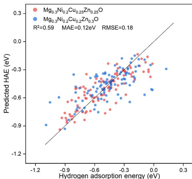
Fig. 10 Performance of DimeNet++ for predicting the hydrogen adsorption energy (HAE) on the (100) surfaces of two different compositions,  $\text{Mg}_{0.3}\text{Ni}_{0.2}\text{Cu}_{0.25}\text{Zn}_{0.25}\text{O}$  and  $\text{Mg}_{0.3}\text{Ni}_{0.2}\text{Cu}_{0.2}\text{Zn}_{0.3}\text{O}$ , from  $\text{Mg}_{0.25}\text{Ni}_{0.25}\text{Cu}_{0.25}\text{Zn}_{0.25}\text{O}$  used for training.
