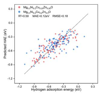
Fig. 10 Performance of DimeNet++ for predicting the hydrogen adsorption energy (HAE) on the (100) surfaces of two different compositions,  $Mg_{0.3}Ni_{0.2}Cu_{0.25}Zn_{0.25}O$  and  $Mg_{0.3}Ni_{0.2}Cu_{0.2}Zn_{0.3}O$ , from Mg<sub>0.25</sub>Ni<sub>0.25</sub>Cu<sub>0.25</sub>Zn<sub>0.25</sub>O used for training.
