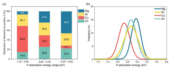
Fig. 7 Relationship between the H adsorption strength and the metal element: (a) Percent distribution among the four metal elements at position 5 for different HAE ranges; (b) distribution of HAEs for a given metal element at position 5 which refers to the metal site directly beneath the O site where H adsorbs (see Fig. 1c).
