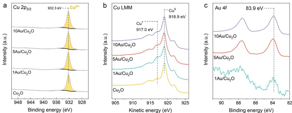
Fig. 7 Quasi-*in situ* XPS spectra of the (a) Cu 2p<sub>3/2</sub>, (b) Cu LMM and (c) Au 4f regions (spectra recorded after 1 h CO<sub>2</sub>RR at -0.9 V vs. RHE, transfer through vacuum system without air exposure).
