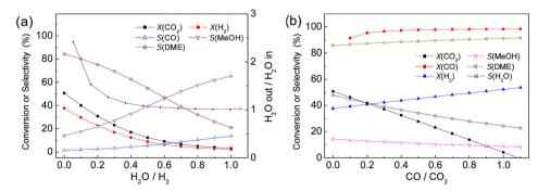
Fig. 5 Effect of a) H<sub>2</sub>O or b) CO addition to feed on equilibrium product distribution in CO<sub>2</sub> hydrogenation to DME. Reaction conditions: 473 K, 3 MPa,  $H_2/CO_2 = 4$ . Copyright<sup>29</sup> 2017 Earth and Environmental Science.
