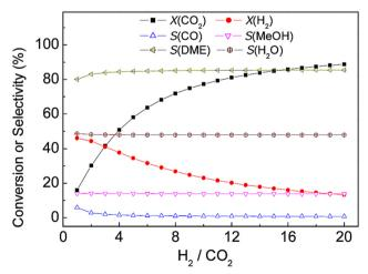
Fig. 4 Effect of H<sub>2</sub>/CO<sub>2</sub> molar ratio on equilibrium product distribution in CO<sub>2</sub> hydrogenation to DME. Reaction conditions: 473 K, 3.0 MPa copyright<sup>29</sup> 2017 Earth and Environmental Science.
