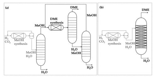
Fig. 11 Simplified flowsheet for (a) the conventional DME production process and (b) the approach by reactive distillation. Copyright<sup>169</sup> ChemEngineering 2022.
