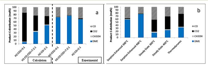
Fig. 10 a) Conventional (calculation, left) versus sorption enhanced (experimental, right, regeneration at 400 °C) direct DME synthesis at 25 bar(a) and 275 °C; b) carbon distribution in steady state SEDMES at 25 bar(a) and 275 °C. Copyright<sup>149</sup> 2020 25th International Symposium on Chemical Reaction Engineering, Florence.
