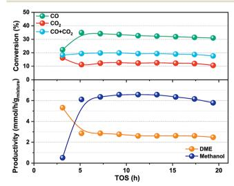
Fig. 9 Evolution of conversions and productivities obtained with the mixture 50:50 CZA: $\gamma$ -Al<sub>2</sub>O<sub>3</sub> combined with the zeolite 3A at 290 °C, 50 bar, and 5000 h<sup>-1</sup>. Copyright<sup>33</sup> 2020 Chemical Engineering Journal Advances.
