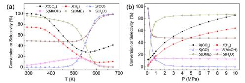
Fig. 3 Effects of (a) temperature at 3.0 MPa and H<sub>2</sub>/CO<sub>2</sub> = 4 and (b) pressure at 473 K and H<sub>2</sub>/CO<sub>2</sub> = 4 on the equilibrium product distribution in  $CO_2$  hydrogenation to DME (X = conversion;  $S_i$  = selectivity to product) copyright<sup>29</sup> 2017 Earth and Environmental Science.
