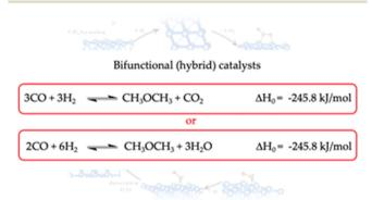
Fig. 2 Alternative (direct) one-step process DME synthesis.
