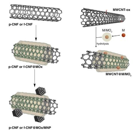
Fig. 7 Synthetic pathways for the preparation of CNF-based hybrid materials.
