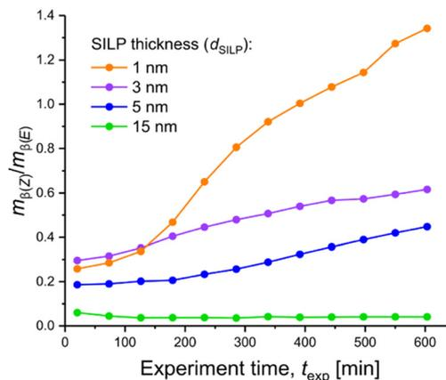
Fig. 6 Comparison of *Z/E*-selectivities via eqn (2) over the course of the four continuous-flow experiments with varied SILP thickness (cf. Fig. 5). Reaction time,  $t_{\text{rct}} = 20$  min; reaction temperature,  $T = 50$  °C.
