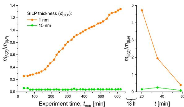
**Fig. 9** Continuous-flow experiments with thin SILP ( $d_{\text{SILP}} = 1$  nm) and thick SILP ( $d_{\text{SILP}} = 15$  nm), followed by a flushing step of the microreactor with pure MTBE and a rest period (stopped flow) of 18 hours. Afterwards, the MTBE solution was flushed out and the effluent analysed for *Z/E*-selectivity using the second dimension of the setup depicted in Fig. 3.
