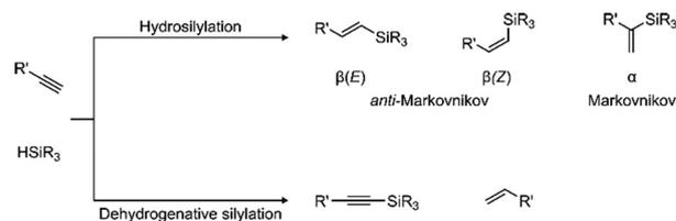
**Scheme 1** Hydrosilylation and dehydrogenative silylation of terminal alkynes.
