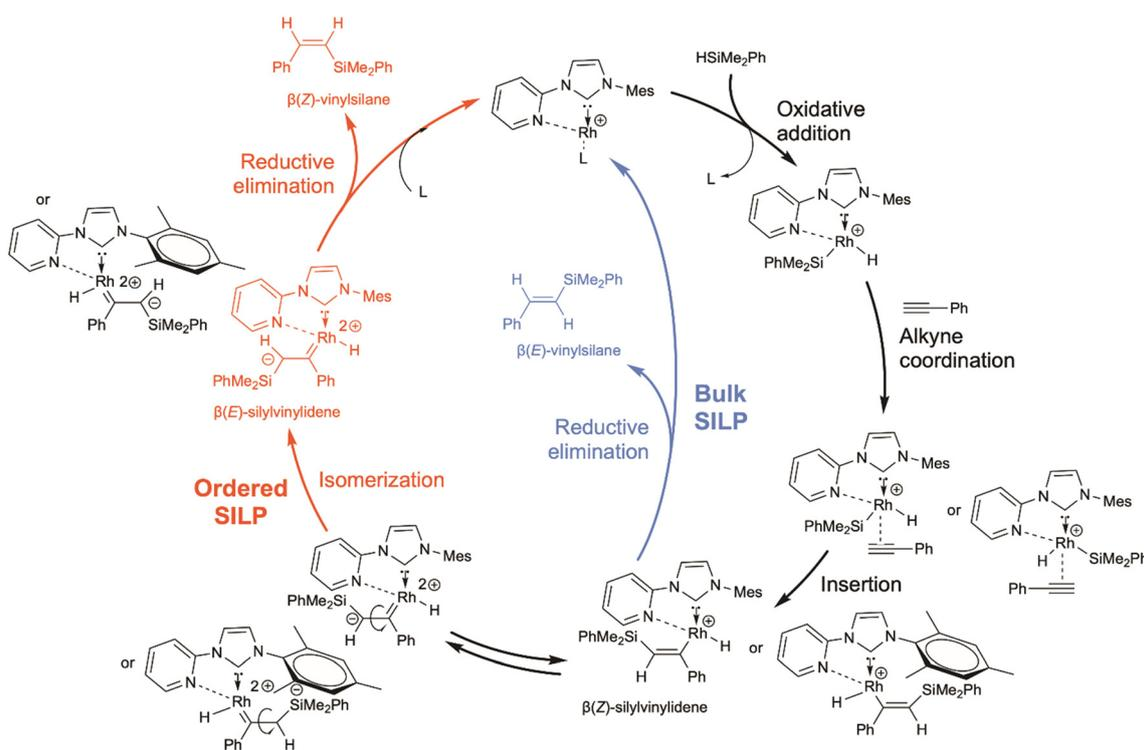
**Scheme 3** Modified Chalk-Harrod mechanism for the preferential formation of  $\beta(Z)$ - or  $\beta(E)$ -vinylsilane isomer in the continuous-flow hydrosilylation reaction between PA and DMPS with Rh-1 in the SILP formed by [BMIM][BF<sub>4</sub>] on a macro-mesoporous silica monolith.
