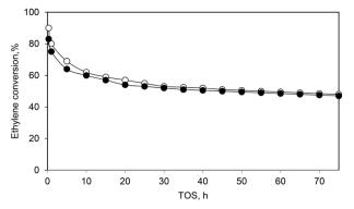
Fig. 12 Ethylene conversion vs. time on stream, over (0) fresh and (1) regenerated Ni-AlSiO<sub>2</sub> catalyst; reaction conditions: C<sub>2</sub>H<sub>4</sub>/N<sub>2</sub> = 1/5 (vol), T = 250 °C, P = 15 bar, WHSV = 1.1 h<sup>-1</sup>. This scheme has been reproduced from ref. 39.
