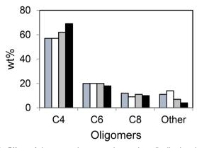
Fig. 8 Effect of the contaminants on the product distribution; blue =  $C_2H_4 + N_2$ , white =  $C_2H_4 + N_2 + H_2$ , grey =  $C_2H_2 + N_2 + CO$ , black =  $C_2H_2 + N_2 + H_2O$ ; TOS = 30 h, T = 250 °C, catalyst: Ni-AlSBA-15. This scheme has been reproduced from ref. 39.
