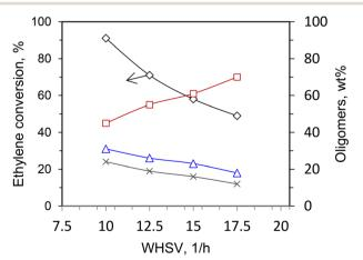
Fig. 5 Ethylene conversion and oligomer distribution at various WHSV; Ni-SBA-15 catalyst; ( $\lozenge$ ) % ethylene conversion, ( $\square$ ) % C<sub>4</sub>, ( $\Delta$ ) % C6, (x)  $C_{8+}$ ; conditions: 3.0 MPa of ethylene, T = 150 °C, TOS = 1 h. This scheme has been reproduced from ref. 40.
