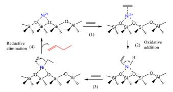
Scheme 6 Simplified catalytic cycle proposed for the activation and dimerization of ethylene on the active Ni<sup>2+</sup> centers of Ni-Beta catalysts: (1) ethylene adsorption on Ni site; (2) oxidative adition; (3) ethylene insertion; (4) reductive elimination of butene. This scheme has been adapted from ref. 7 with permission from American Chemical Society, copyright 2025.
