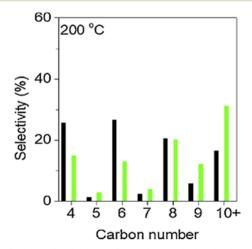
Fig. 15 Carbon distribution of products obtained after ethylene reaction for 16 h on stream over Ni/Siral-30 (black) and Ni/Siral-30 + H-7SM-5 (green) in the continuous fixed-bed reactor. This figure has been reproduced from ref. 75 with permission from Elsevier, copyright
