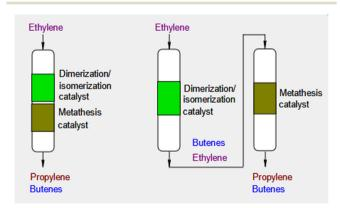
Fig. 13 ETP processes with one or two reactors.
