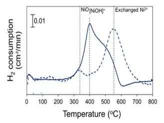
Fig. 2 H<sub>2</sub> TPR profiles of Ni-Beta catalysts after in situ pretreatment at 300 °C (solid lines) and 500 °C (dashed lines). This figure has been reproduced from ref. 14.
