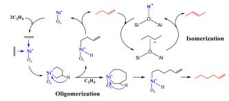
**Scheme 11** Proposed catalytic cycles for linear ethylene oligomerization involving Ni<sup>+</sup> and H<sup>+</sup> as active sites on the Ni-AlSBA-15 catalyst  $(O_s^{2^-} = \text{surface oxide ions})$ . This scheme has been adapted from ref. 40.
