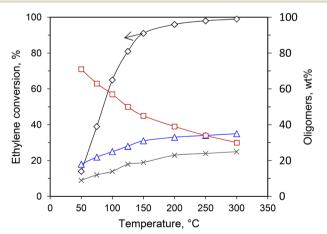
Fig. 4 Ethylene conversion and oligomer distribution at various temperatures; Ni-SBA-15 catalyst; (◊) % ethylene conversion, (□) % C4, ( $\Delta$ ) % C6, (x) C8; conditions: 3.0 MPa, WHSV = 10 h<sup>-1</sup>. This scheme has been reproduced from ref. 40.
