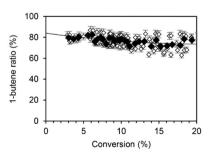
Fig. 3 Butene selectivity (left) and 1-C4 isomer ratio (right) vs. ethylene conversion. Catalyst: 0.1 g of Ni-AlKIT-6, T = 40-80 °C, Pethylene = 0.4-2 MPa,  $P_{\text{total}} = 3.0$  MPa, contact time = 15–98 s. This scheme has been reproduced from ref. 46.
