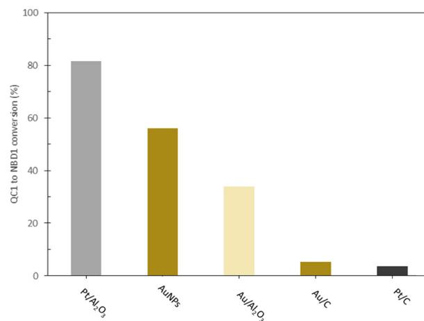
Fig. 7 QC1 back conversion measured in Duratherm-HTO22 after 1 hour with the four 5 wt% catalysts and the industry standard.
