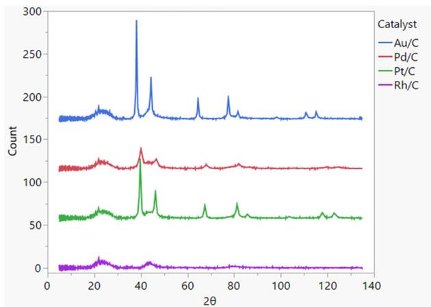
Fig. 2 XRD spectra for the carbon-supported catalysts.
