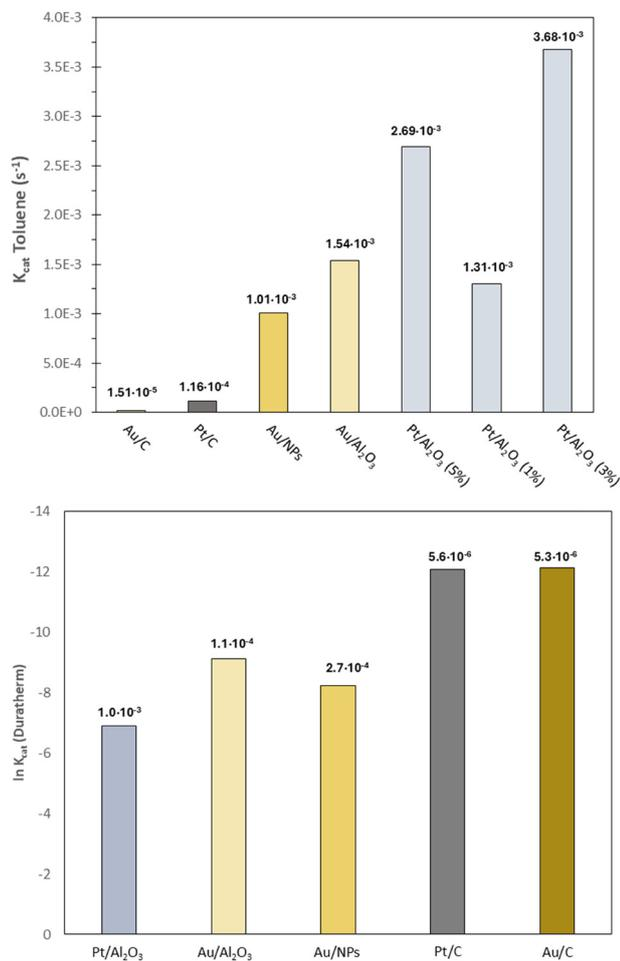
**Fig. 8** Top) Catalytic rate constants of the different catalysts measured in toluene by method 1. Indicated values correspond to the  $k_{\text{cat}}$ . Bottom) Logarithmic representation of the rate constants of the different catalysts in Duratherm-HTO22. Indicated values correspond to the  $k_{\text{cat}}$ .
