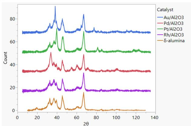
Fig. 3 XRD spectra for the alumina-supported catalysts.
