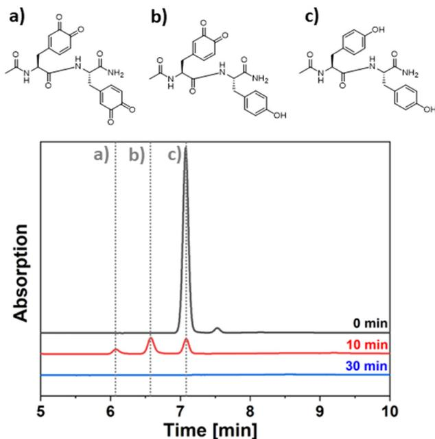
**Fig. 2** HPLC chromatograms for samples extracted from the reaction mixture for the conversion of Ac-YY-NH<sub>2</sub> by immobilized SinATyr in batch mode. The chromatogram was recorded using a reversed phase column (C18) running a gradient of water/acetonitrile (+0.05%(v/v) formic acid) from 95/5 v/v to 5/95 v/v over the course of 17 min. Detection was done via UV absorption at 270 nm.
