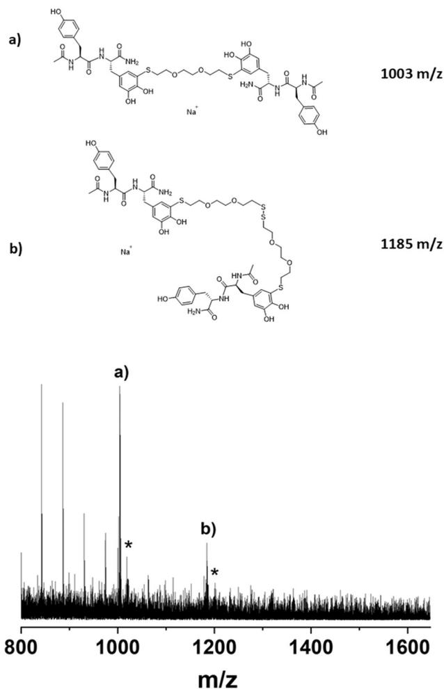
Fig. 4 MALDI-ToF analysis after enzymatic activation of Ac-YY-NH<sub>2</sub> in flow mode and subsequent exposure to 2,2'-(ethylenedioxy) diethanedithiol. The Ac-YY-NH<sub>2</sub>/dithiol ratio had been set to 3.3. The matrix for the MALDI-ToF measurement was dithranol.
