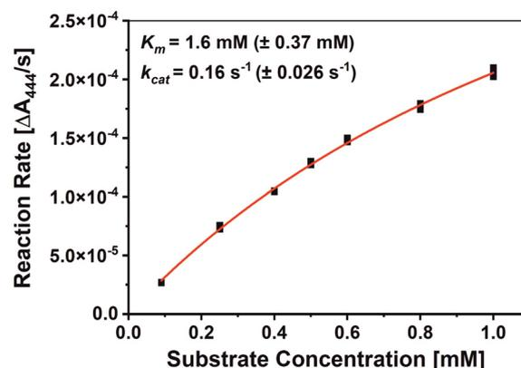
**Fig. 1** Michaelis–Menten plot of *SinATyr* on Ac-YY-NH<sub>2</sub>. Different Ac-YY-NH<sub>2</sub> molarities were oxidized by *SinATyr* and the corresponding absorption values have been measured in triplicates in 50 mM sodium citrate buffer (pH 6.8).
