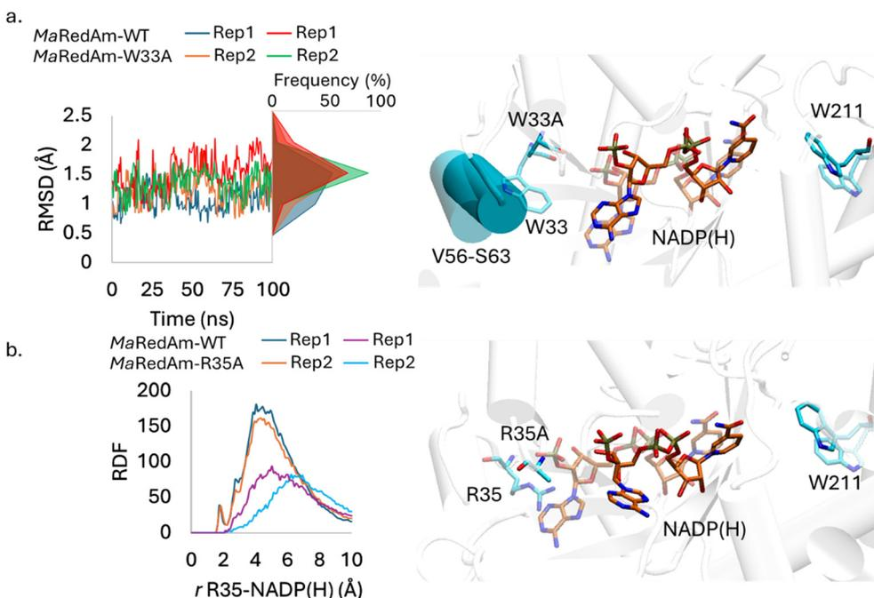
**Fig. 2** RMSD of V56-S63  $\alpha$ -helix obtained from molecular dynamics (MD) simulations of *MaRedAm*-WT and *MaRedAm*-W33A systems (a). RDFs of R35-NADP(H) pair calculated from MD simulations of *MaRedAm*-WT and *MaRedAm*-R35A systems (b). For clarity, hydrogens were omitted, and only relevant species were reported. In the figures, atoms in transparent-background representation are for the wild-type enzyme.
