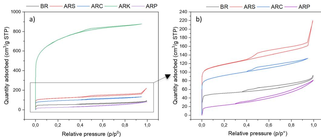
**Fig. 1** N<sub>2</sub> adsorption-desorption isotherms of the non-activated and activated biochar samples. a) All samples. b) Magnification between 0 and 240 cm<sup>3</sup> g<sup>-1</sup>.
