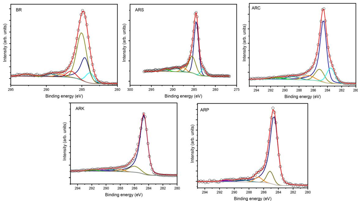
Fig. 4 XPS spectra of non-activated and activated biochar samples.
