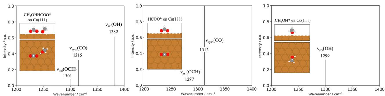
**Fig. 10** Computed infrared spectra for HCOO\*, CH<sub>3</sub>OH\*, and CH<sub>3</sub>OHHCOO\* on Cu(111). Intensities are normalized with respect to the most intense mode calculated for each species. Peaks within 1200–1400 cm<sup>-1</sup> wavenumber range are considered interesting. The top view and side view of the computed adsorbed structures are shown, Copper atoms are in orange, carbon in grey, oxygen in red, and hydrogen in white.
