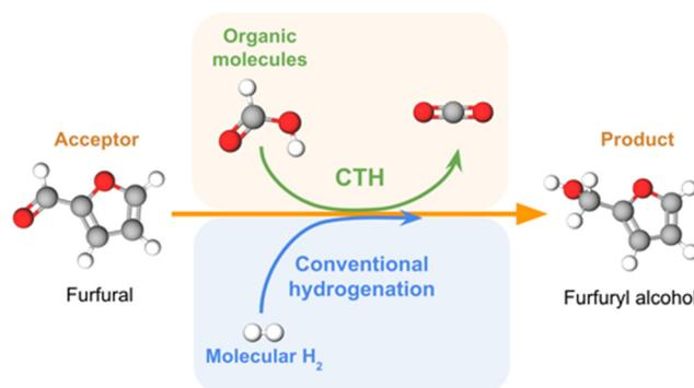
Fig. 1 A schematic comparison between catalytic transfer hydrogenation/hydrogenolysis (CTH) using an organic hydrogen donor and conventional hydrogenation using H<sub>2</sub>.
