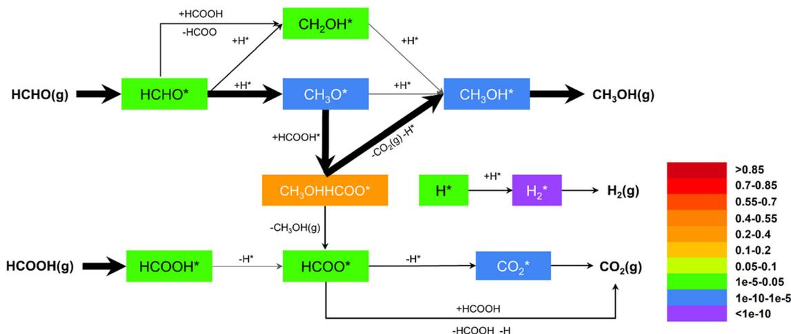
**Fig. 9** Reaction network for the new “HCOOH-cofeed” model based on 2/9th ML HCOO\*<sup>-</sup>-covered surface at 373 K, 1 atm, with partial pressure of HCHO and HCOOH/H<sub>2</sub> being 0.15 and 0.08 respectively (and rest inert). The width of the arrows qualitatively represents the magnitude of the reaction flux, and the coverages of surface intermediate were color coded by different level.
