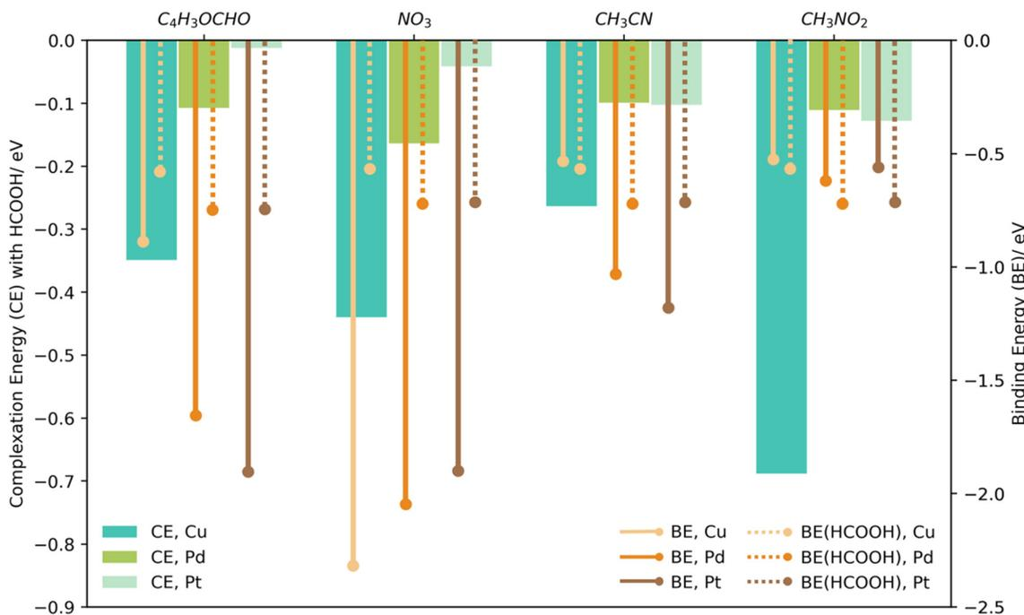
**Fig. 12** Complexation energies with HCOOH (CE) and binding energies (BE) of furfural, nitrate, acetonitrile and nitromethane (from left to right), and binding energies of HCOOH on Cu(111), Pd(111) and Pt(111) respectively. Complexation energies (CE) are represented by bar, while binding energies (BE) of hydrogen acceptors are represented by solid line, and binding energies (BE) of HCOOH are represented by dashed line.
