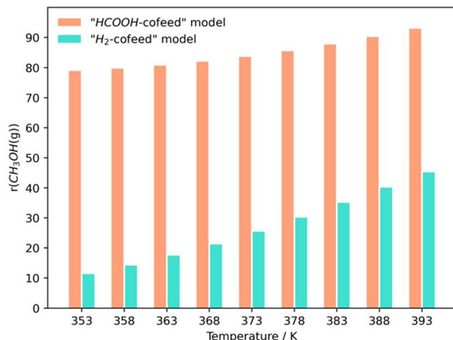
**Fig. 8** Comparison of the hydrogenation rate of the final “HCOOH-cofeed” model based on 2/9th ML HCOO\*<sup>-</sup>-covered surface and “H<sub>2</sub>-cofeed” model based on 3/9th ML CH<sub>3</sub>O\*<sup>-</sup>-covered surface under various temperature, total pressure of 1 atm, with partial pressure of HCHO and HCOOH/H<sub>2</sub> being 0.15 and 0.08 respectively (and rest inert). Hydrogenation rate is indicated by the flow rate of CH<sub>3</sub>OH(g) generated.
