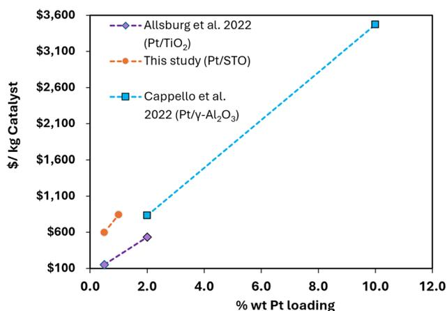
Fig. 4 The catalyst cost depends on the percentage weight of Pt loading in all studies. This study shows the cost of catalyst Pt/STO for 0.5 to 1 wt% Pt loading. Van Allsburg *et al.* showed the Pt/TiO<sub>2</sub> catalyst purchase cost for 0.5 to 2 wt% Pt loading and Cappello *et al.* presented the Pt/ $\gamma$ -Al<sub>2</sub>O<sub>3</sub> catalyst purchase cost for 2 to 10 wt% Pt loading.
