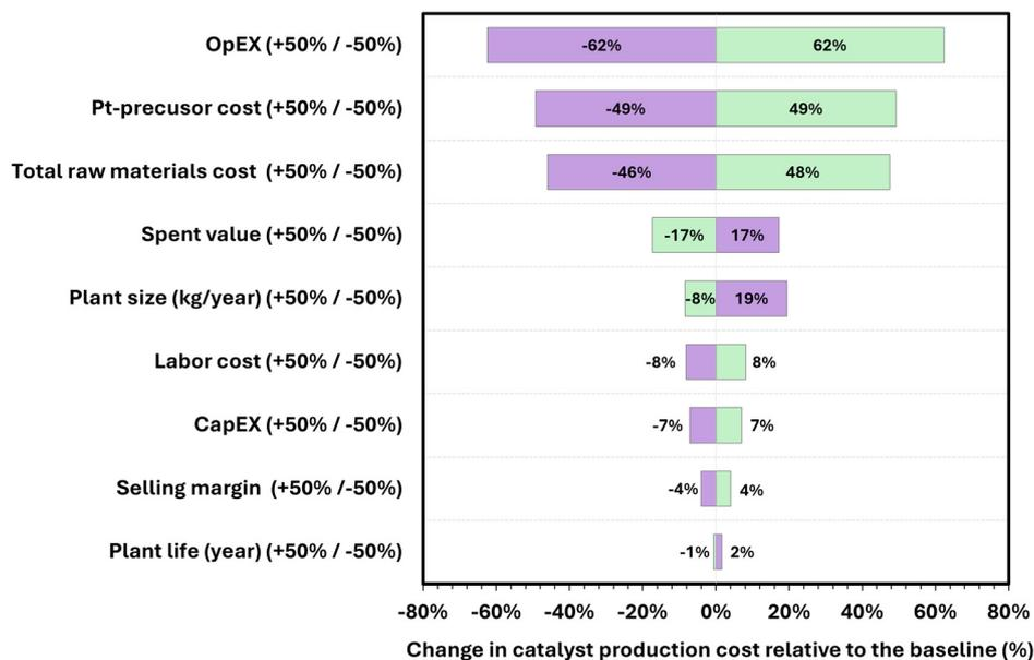
Fig. 5 Sensitivity analyses for the synthesis catalyst production cost. The production cost variation is due to the variation of different factors. Baseline catalyst cost = \$842 per kg catalyst. The dark green color and the lavender color represent the high value and the low value, respectively.
