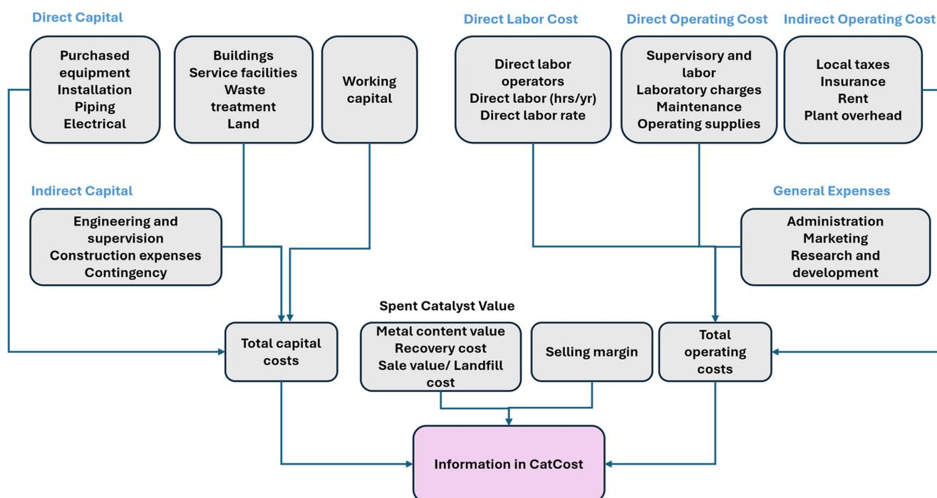
Fig. 2 Estimation of the Pt/STO catalyst cost including the cost components in the CatCost.
