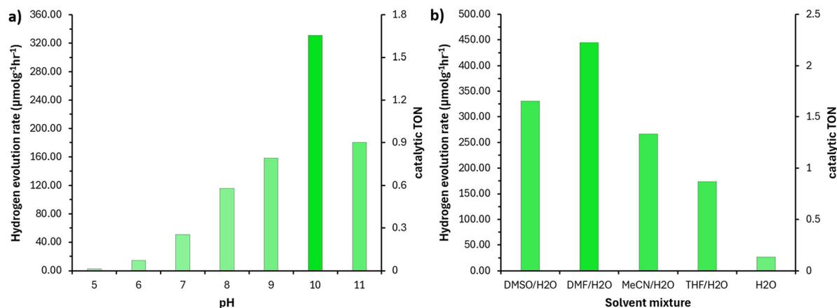
**Fig. 4** a) Rate of hydrogen evolution determined from volume of hydrogen generated over a 5-hour period, all conditions were kept consistent with initial screen parameters (see ESI,† S7) while pH was varied as specified. b) Rate of hydrogen evolution determined from volume of hydrogen generated over a 5-hour period, solvent mixture varied while all other conditions were consistent with initial screen.
