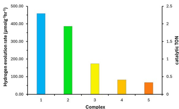
**Fig. 5** Hydrogen generation rate of complexes 1–5 in the optimum conditions informed the screening of complex 2. Reaction conditions: 20  $\mu\text{M}$  iridium complex,  $[\text{Co}(\text{bpy})_3(\text{PF}_6)_2]$  1 mM, DMSO:H<sub>2</sub>O (1:1, 5 mL), 0.35 M NEt<sub>3</sub>, LiCl 0.3 M, and pH 10, samples were irradiated for 5 h under an oriel solar simulator 1.0 sun.
