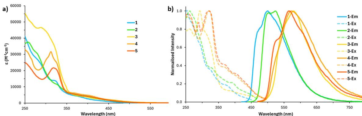
Fig. 2 a) UV-vis spectra of complexes 1–5 in  $\text{CH}_3\text{CN}$  ( $1.0 \times 10^{-5}$  M, 298 K). b) Normalised emission-excitation spectra of complexes 1–5 in  $\text{CH}_3\text{CN}$  ( $1.0 \times 10^{-5}$  M, 298 K), the solid lines represent the emission while the dashed lines represent the absorption. All emission spectra were excited at 300 nm.
