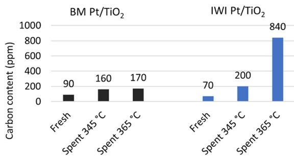
Fig. 7 Carbon content of the fresh and spent BM Pt/TiO<sub>2</sub> and IWI Pt/TiO<sub>2</sub> catalysts.
