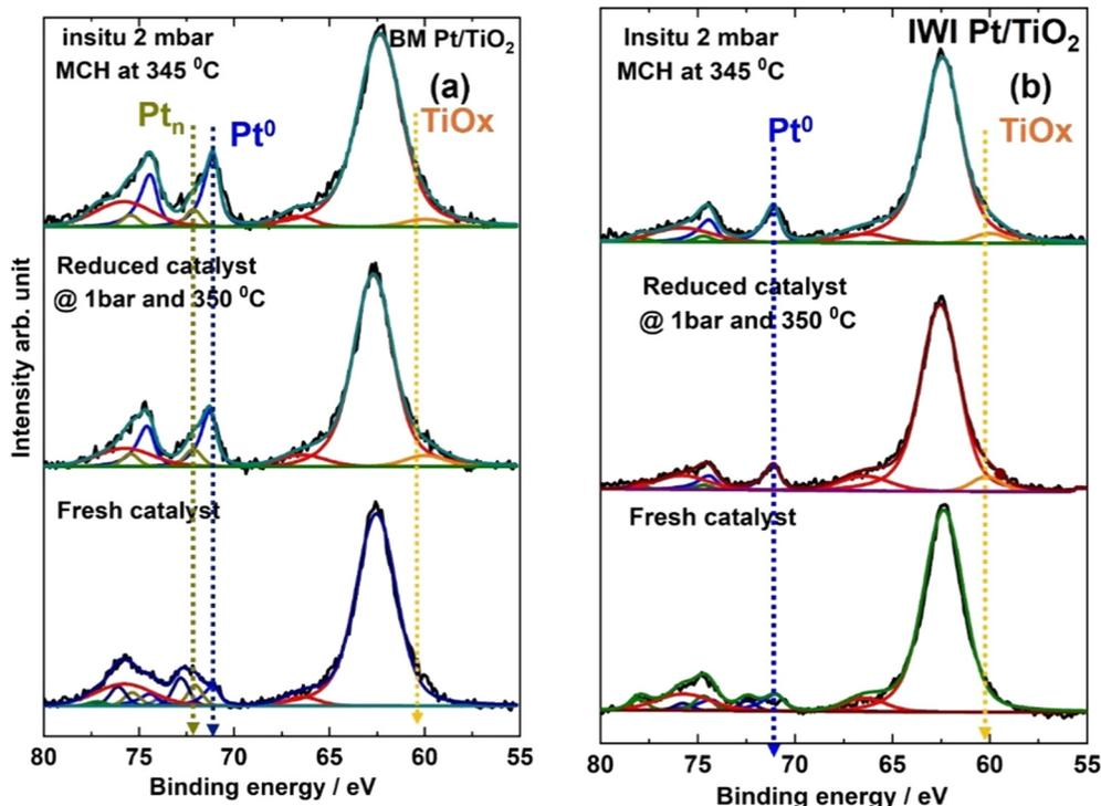
Fig. 6 APXPS Pt 4f and Ti 3s spectra recorded for fresh catalyst (bottom), after reduction (middle) and during the dehydrogenation (top) for (a) BM Pt/TiO<sub>2</sub> and (b) IWI Pt/TiO<sub>2</sub>.
