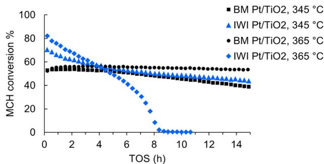
Fig. 1 Catalytic performance of the monometallic Pt/TiO<sub>2</sub> catalysts in terms of MCH conversion at two different temperatures: 345 and 365 °C. Atmospheric pressure, 0.2 g catalyst, MCH feed rate 0.1 ml min<sup>-1</sup>.
