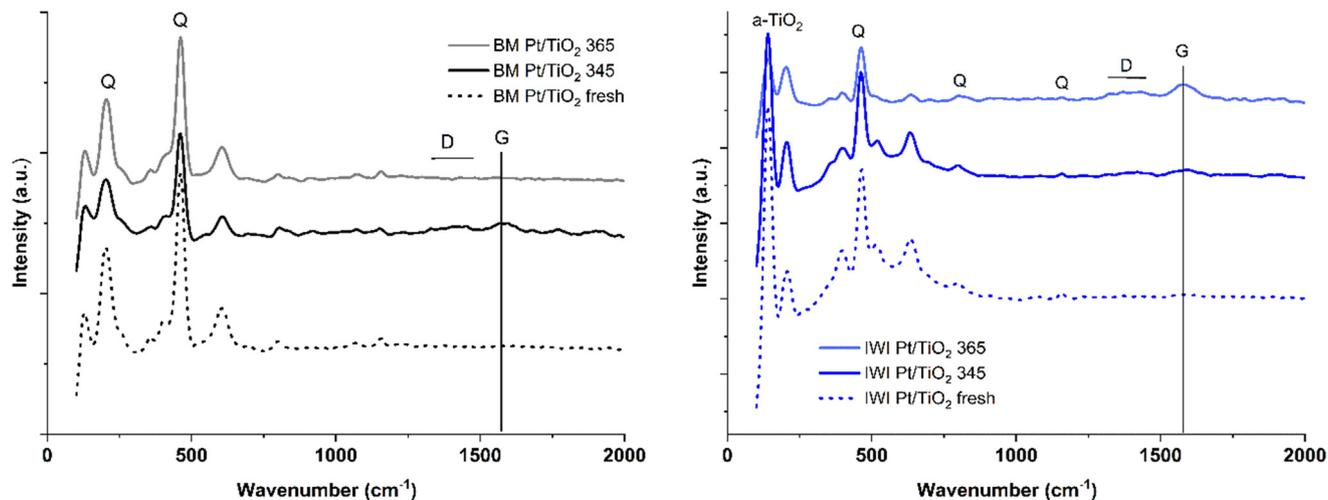
Fig. 8 Raman spectra of fresh and spent BM Pt/TiO<sub>2</sub> (left) and IWI Pt/TiO<sub>2</sub> (right) catalysts. D and G denote carbonaceous species, Q quartz.
