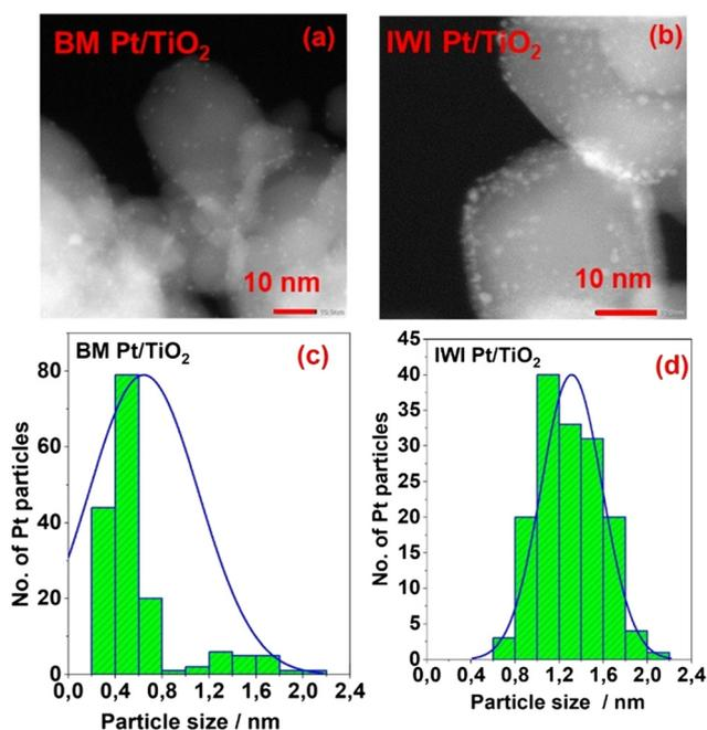
Fig. 3 HAADF-STEM images and Pt particle size distributions of the fresh catalysts (a and c) BM Pt/TiO<sub>2</sub>, (b and d) IWI Pt/TiO<sub>2</sub>.
