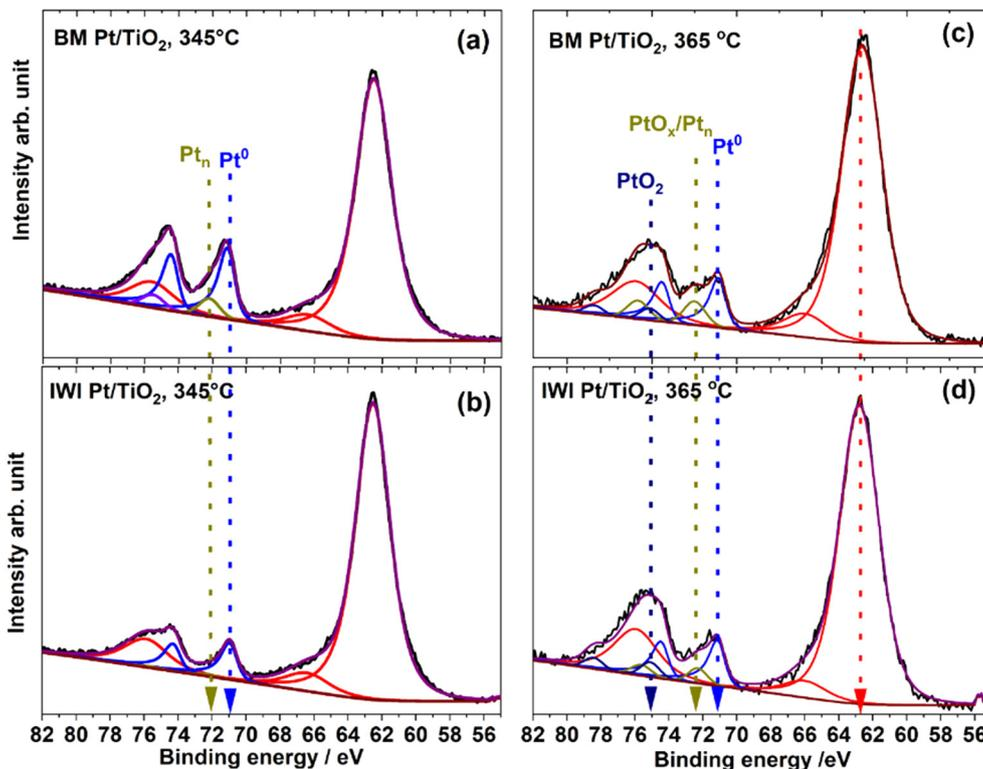
Fig. 5 The Pt 4f and Ti 3s spectra of spent catalysts after dehydrogenation at different temperatures. (a) BM Pt/TiO<sub>2</sub>, 345 °C (b) IWI Pt/TiO<sub>2</sub>, 345 °C (c) BM Pt/TiO<sub>2</sub>, 365 °C and (d) IWI Pt/TiO<sub>2</sub>, 365 °C.
