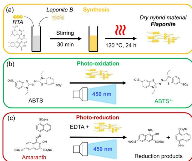
**Fig. 1** (a) Preparation of the flavin-LAPONITE® hybrid (Flaponite). Illustration of the Flaponite-catalysed (b) photo-oxidation of ABTS (b) and photo-reduction of amaranth dye (c) demonstrated within this work.
