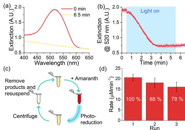
**Fig. 3** (a) Extinction spectra of  $0.5 \text{ mg mL}^{-1}$  Flap<sub>Mix</sub> and  $50 \mu\text{M}$  amaranth before and after light irradiation. (b) Extinction at  $520 \text{ nm}$  over time during the photo-reduction of amaranth with Flap<sub>Mix</sub>. (c) Scheme showing the recycling of the photocatalyst and (d) the rate of amaranth photoreduction during each sequential run ( $n = 3$ ).
