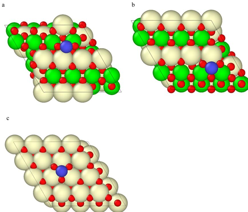
Fig. 4 Nickel binding sites (a)  $\text{Ni}_{\text{CeZr}}/\text{CZO}(111)$ , (b)  $\text{Ni}_{\text{ZrCe}}/\text{CZO}(111)$  and (c)  $\text{Ni}/\text{CeO}_2(111)$  (O, red; Ce, yellow; Zr, green; Ni, blue).
