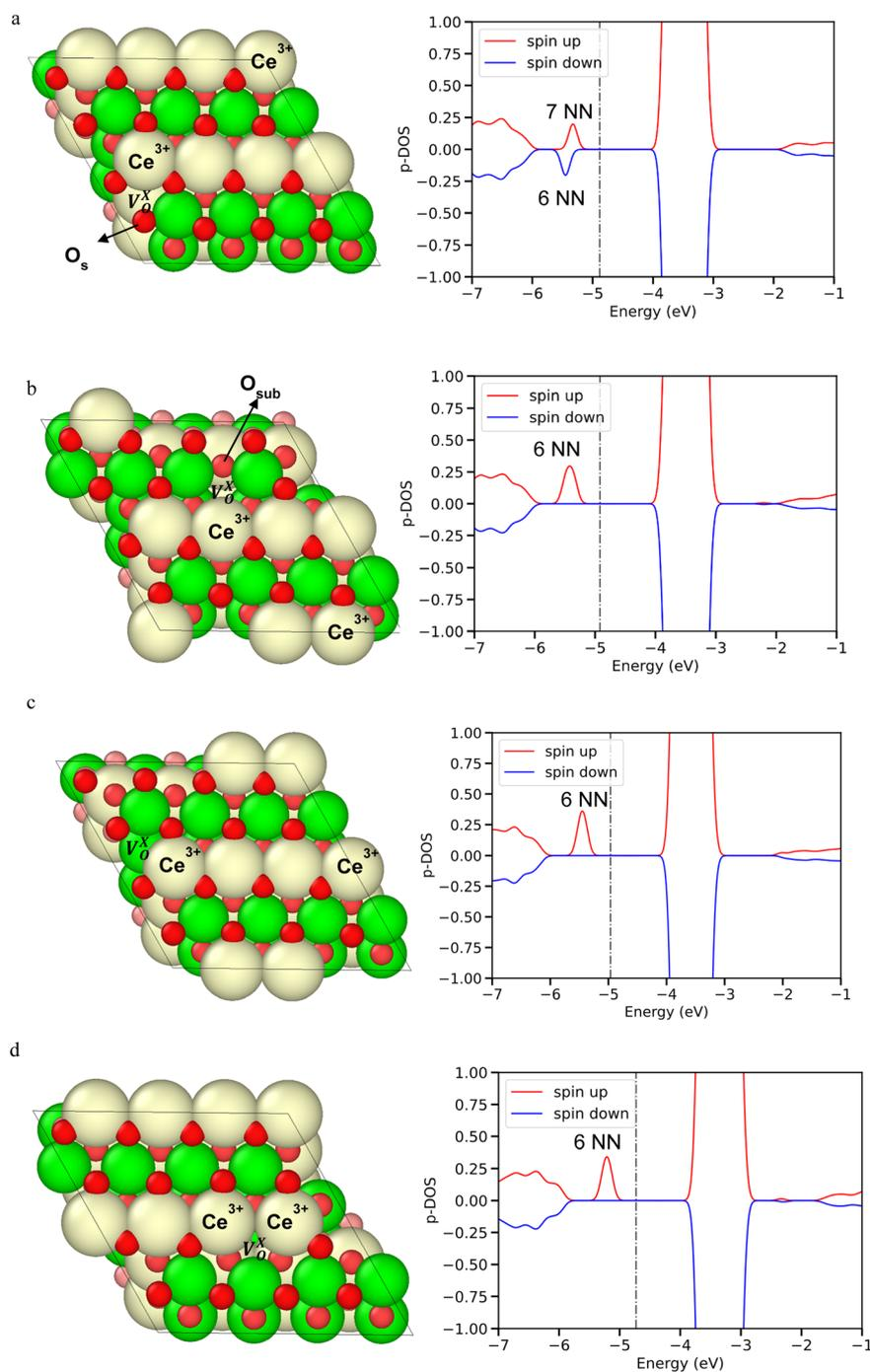
**Fig. 2** Defective CZO(111) surface showing the vacancy and reduced cerium atoms and Ce pDOS on its f states for (a)  $\text{O}_{\text{Zr}}^{\text{sub}}$  vacancy, (b)  $\text{O}_{\text{Zr}}^{\text{s}}$  vacancy, (c)  $\text{O}_{\text{Ce}}^{\text{sub}}$  vacancy, and (d)  $\text{O}_{\text{Ce}}^{\text{s}}$  vacancy. (O, red; Ce, yellow; Zr, green). Left structures; right pDOS. The vertical gray dashed line indicates the Fermi level referenced to the vacuum level.
