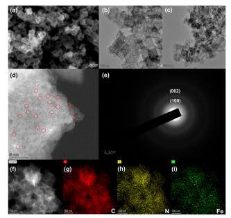
Fig. 2 (a) SEM image of Fe-N-C NH<sub>3</sub>. (b) and (c) TEM images of Fe-N-C NH<sub>3</sub>. (d) Aberration-corrected HAADF-STEM image of Fe-N-C NH<sub>3</sub>. (e) SAED pattern of Fe-N-C NH<sub>3</sub>. (f)-(i) Elemental mapping analysis of C, N, and Fe of Fe-N-C NH<sub>3</sub> by HAADF-STEM.
