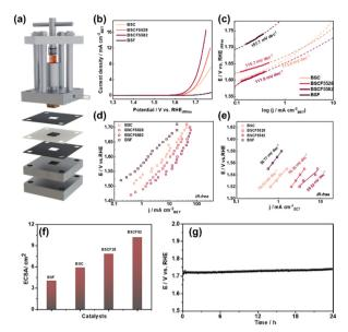
**Fig. 3** (a) Schematic illustration of the forced-flow cell. (b) LSVs curves and (c) tafel slope of BSC, BSF, BSCF5582 and BSCF5528 by RDE method. (d) i-e curves and (e) tafel slope of BSC, BSF, BSCF5582 and BSCF5528 using the forced-flow cell method and time zero analysis. (f) ECSA, (g) stability of BSCF5582 with forced flow cell at 100 mA cm $^{-2}$  for 24 h.
