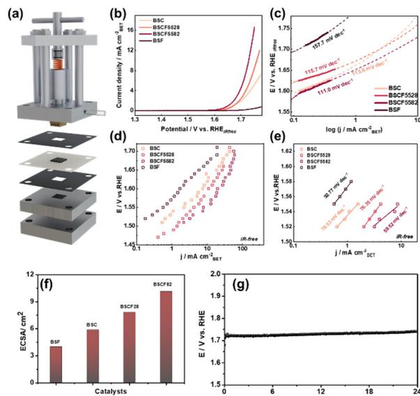
**Fig. 3** (a) Schematic illustration of the forced-flow cell. (b) LSVs curves and (c) tafel slope of BSC, BSF, BSCF5582 and BSCF5528 by RDE method. (d) *i*-*e* curves and (e) tafel slope of BSC, BSF, BSCF5582 and BSCF5528 using the forced-flow cell method and time zero analysis. (f) ECSA, (g) stability of BSCF5582 with forced flow cell at 100 mA cm<sup>-2</sup> for 24 h.
