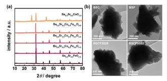
Fig. 1 (a) XRD patterns and (b) TEM images of Ba $_{0.5}$ Sr $_{0.5}$ Co $_x$ Fe $_{1-x}$ O $_{3-\delta}$  (x=0,0.2,0.5,0.8,1).
