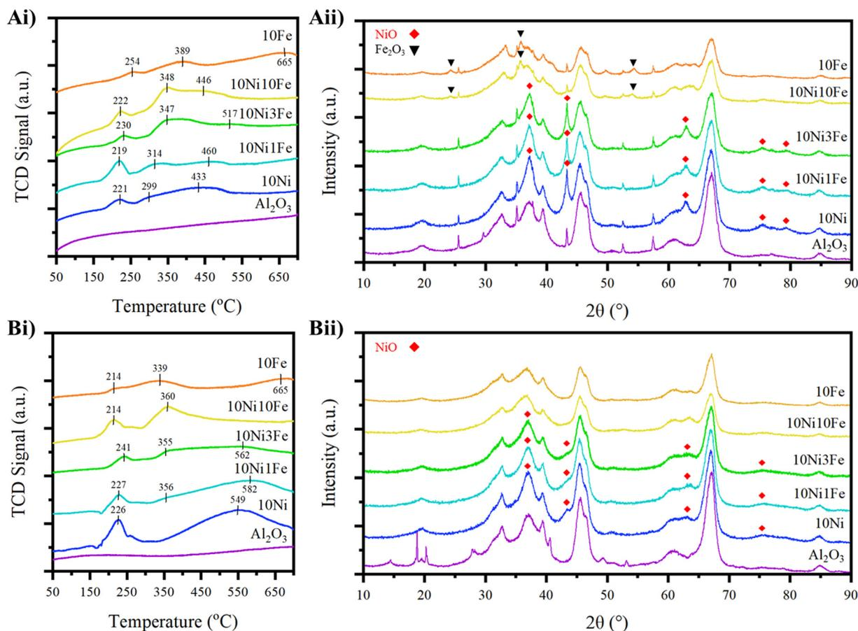
Fig. 1 H<sub>2</sub>-TPR and XRD analysis of the as-prepared WI and DP catalysts. A) WI catalysts, B) DP catalysts, i) H<sub>2</sub>-TPRs profiles, ii) XRD profiles.
