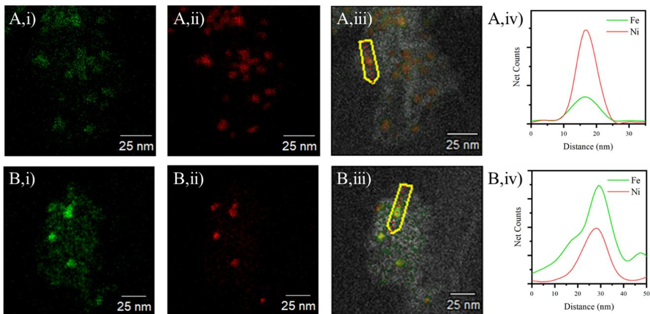
Fig. 3 EDS mapping and line scans of 10Ni10Fe WI and DP catalysts. A) 10Ni10Fe WI, B) 10Ni10Fe DP; i) Ni mapping, ii) Fe mapping, iii) Ni-Fe mapping overlay, iv) Ni-Fe line scans.
