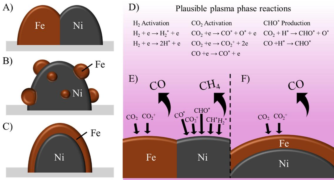
**Fig. 9** Postulated influence of different bimetallic Ni-Fe configurations on the CO<sub>2</sub> methanation pathways. A) Janus-like segregated Ni and Fe structure, B) Fe-decorated Ni structure C) Ni-core/Fe-shell structure, D) plausible plasma phase reactions, E) influence of bimetallic interactions in structures A and B on plasma methanation, and F) influence of structure C on CO production.
