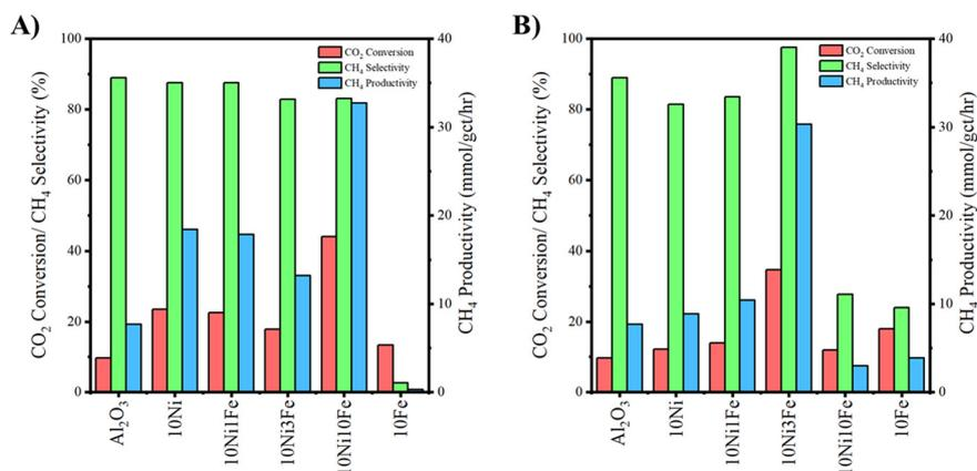
Fig. 7 CO<sub>2</sub> conversion and CH<sub>4</sub> selectivity during plasma-catalytic CO<sub>2</sub> methanation at 150 °C by 10Ni, 10Fe and 10NixFe (where x = 1, 3, 10) Al<sub>2</sub>O<sub>3</sub>-supported catalysts. Neat Al<sub>2</sub>O<sub>3</sub> is included as a control. Where: A) WI; B) DP. Operating conditions: voltage = 150 V, discharge frequency = 850 Hz, resonance frequency = 60 kHz, duty cycle = 66 μs, power = ~28 W.
