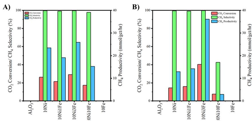
Fig. 6 CO<sub>2</sub> conversion and CH<sub>4</sub> selectivity during thermal-catalytic CO<sub>2</sub> methanation at 300 °C by 10Ni, 10Fe and 10NixFe (where x = 1, 3, 10) Al<sub>2</sub>O<sub>3</sub>-supported catalysts. Neat Al<sub>2</sub>O<sub>3</sub> is included as a control. Where: A) WI; B) DP.
