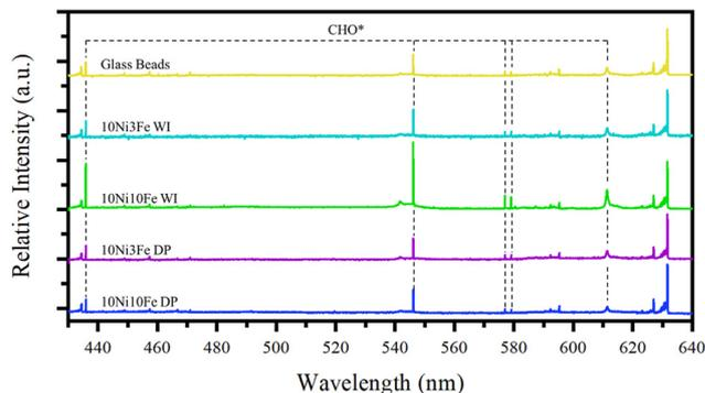
Fig. 8 *In situ* OES spectra of selected WI and DP catalysts over the spectral range of 430 nm to 640 nm during plasma-catalytic CO<sub>2</sub> methanation. The *in situ* OES spectrum for glass beads only is provided as a control.
