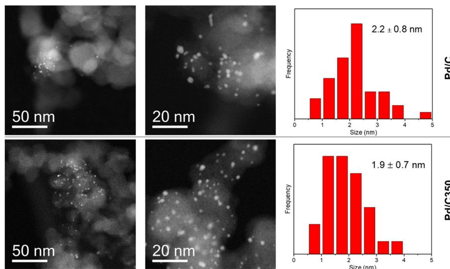
**Fig. 2** STEM-HAADF images and corresponding particle size distribution of (top) Pd/C and (bottom) Pd/C350 catalysts.
