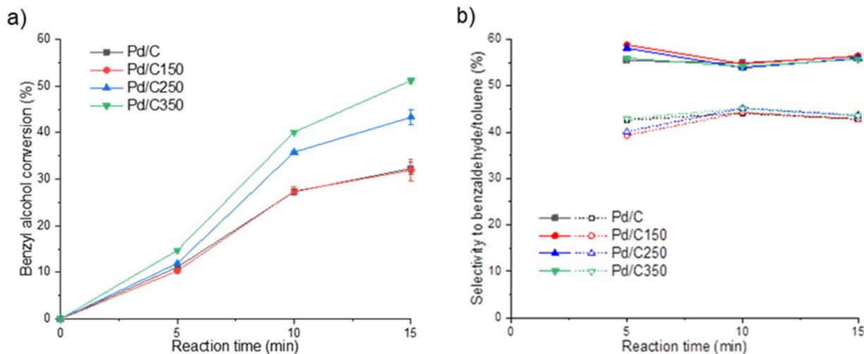
**Fig. 3** Catalytic performance for solvent-free benzyl alcohol oxidation. a) Benzyl alcohol conversion and b) product selectivity toward benzaldehyde (solid line) and toluene (dashed line) as a function of time over Pd/C, Pd/C150, Pd/C250, and Pd/C350. Reaction conditions: 16 mL of benzyl alcohol, 72 mg of catalyst, 3 bar O<sub>2</sub>, reaction temperature 120 °C, stirring rate 1000 rpm. Associated error bars were generated by performing each test in triplicate.
