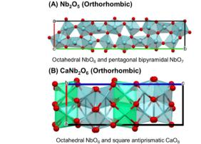
Fig. 1 Crystalline structures of (A) Nb<sub>2</sub>O<sub>5</sub> and (B) CaNb<sub>2</sub>O<sub>6</sub>. Red balls, blue and green sticks represent O, Nb and Ca, respectively.
