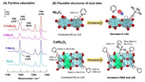
Fig. 2 (A) Difference IR spectra of adsorbed pyridine species on the prepared catalysts at 30 °C. (B) Plausible structures of acid sites on Nb<sub>2</sub>O<sub>5</sub> and CaNb<sub>2</sub>O<sub>6</sub> before and after P-treatment. White circles in (B) indicate oxygen defect sites.
