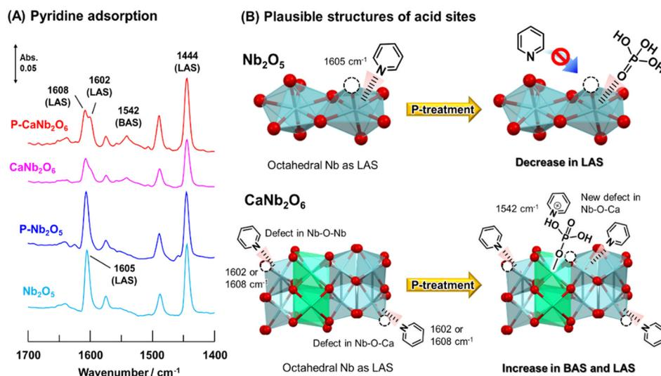
**Fig. 2** (A) Difference IR spectra of adsorbed pyridine species on the prepared catalysts at 30 °C. (B) Plausible structures of acid sites on  $\text{Nb}_2\text{O}_5$  and  $\text{CaNb}_2\text{O}_6$  before and after P-treatment. White circles in (B) indicate oxygen defect sites.
