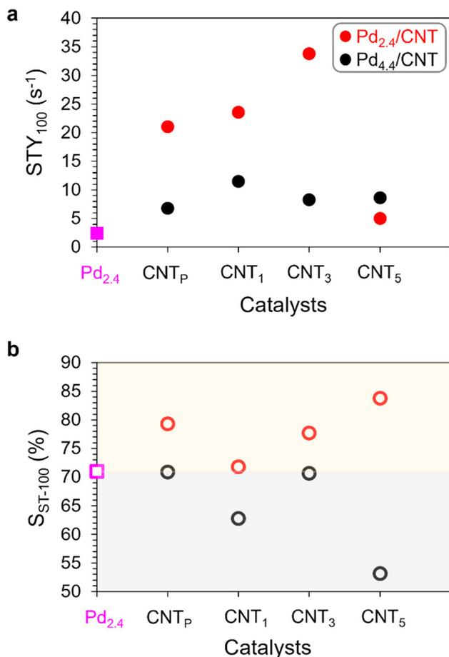
Fig. 5 Evolution of (a) site time yield and (b) styrene selectivity according to the catalyst type (free-standing Pd<sub>2.4</sub> NPs, Pd<sub>2.4</sub>/CNT and Pd<sub>4.4</sub>/CNT series) for phenylacetylene hydrogenation at 100% conversion.
