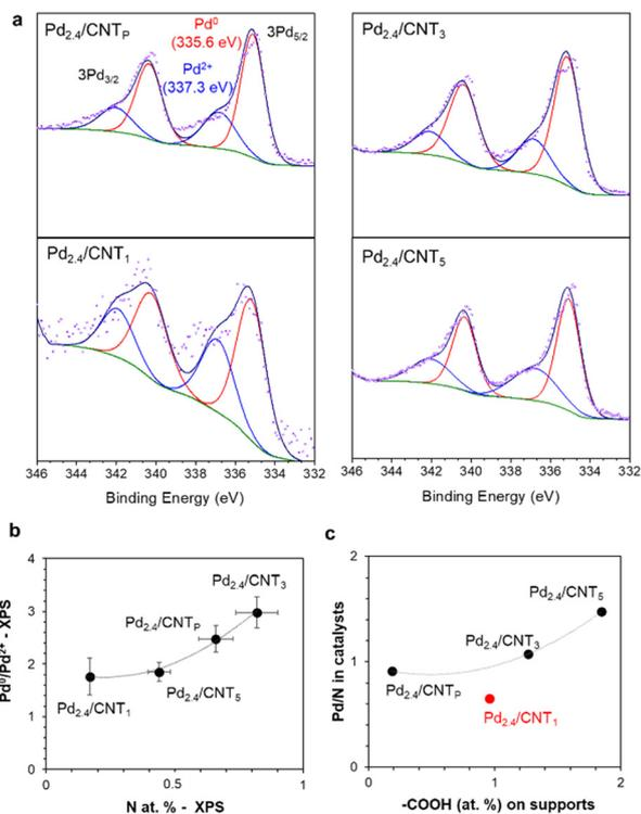
Fig. 4 (a) High-resolution XPS spectra of the Pd 3d region of the CNT-supported Pd<sub>2.4</sub> nanoparticles. (b) Correlation between the at% of nitrogen measured by XPS and the Pd<sup>0</sup>/Pd<sup>2+</sup> ratio for the CNT-supported Pd<sub>2.4</sub> nanoparticle series. (c) Evolution of the Pd/N ratio in the CNT-supported Pd<sub>2.4</sub> nanoparticles with the concentration of carboxylic groups on the bare supports.
