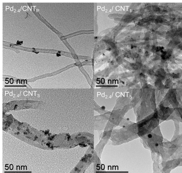
Fig. 3 TEM images of the CNT-supported Pd<sub>2.4</sub> nanoparticles.
