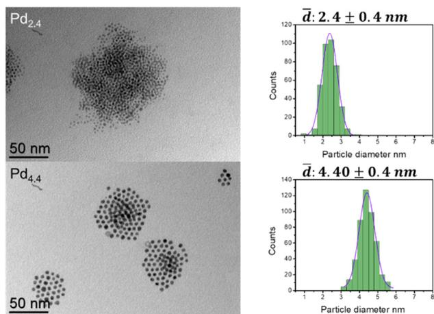
Fig. 2 TEM images of the monodispersed 2.4 ± 0.4 nm and 4.4 ± 0.4 nm Pd<sub>p-NP</sub>.
