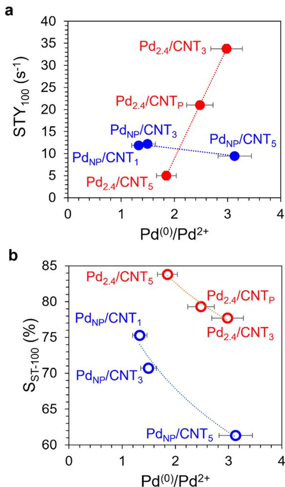
Fig. 6 Evolution of site time yield and styrene selectivity according to  $\text{Pd}^{(0)}/\text{Pd}^{2+}$  ratio in the  $\text{Pd}_{2.4}/\text{CNT}$  (red marks) and  $\text{Pd}_{\text{NP}}/\text{CNT}$  catalyst (blue marks) series.
