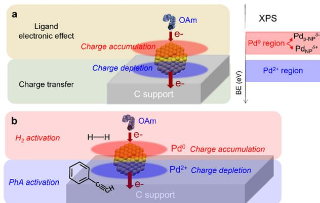
**Scheme 2** (a) Model for charge redistribution in Pd/C catalysts based on charge transfer and electronic ligand effect. (b) Model of dual Pd<sup>(0)</sup> and Pd<sup>2+</sup> site catalyzed mechanism involving H<sub>2</sub> and PhA activation.
