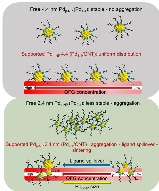
**Scheme 1** Representation of the evolution of Pd<sub>p-NP</sub> distribution on the CNT surface according to the size of the Pd<sub>p-NP</sub> (2.4 or 4.4 nm) and OFGs concentration.
