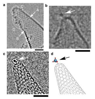
Fig. 3 Representative SMART-EM images of CNH/WO<sub>2</sub>; scale bars: 1 nm. (a) Experimental TEM image after 20 stacks. White arrows and circle indicate single (A and B) and multiple sites (C-E), respectively (Fig. S2†). (b) Out-of-plane WO<sub>2</sub> on CNH. (c and d) TEM simulation and ZC model for out-of-plane model. EDR (electron dose rate) =  $5.7-7.2 \times$  $10^6 e^- nm^{-2} s^{-1}$
