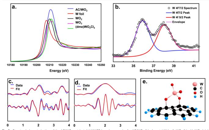
Fig. 2 Structural characterization of the AC/WO<sub>2</sub> catalyst: (a) XANES  $L_{III}$ -edge energies for AC/WO<sub>2</sub> (blue), metal W (red), WO<sub>2</sub> (black), WO<sub>3</sub> (pink) and (dme)WO<sub>2</sub>Cl<sub>2</sub> (green) (b) W 4f XPS spectra for AC/WO<sub>2</sub> (c) EXAFS pRDFs magnitude (top) and real (bottom) for AC/WO<sub>2</sub> (d) EXAFS pRDFs magnitude (top) and real (bottom) for (dme)WO<sub>2</sub>Cl<sub>2</sub> and (e) DFT computed model for AC/WO<sub>2</sub>.
