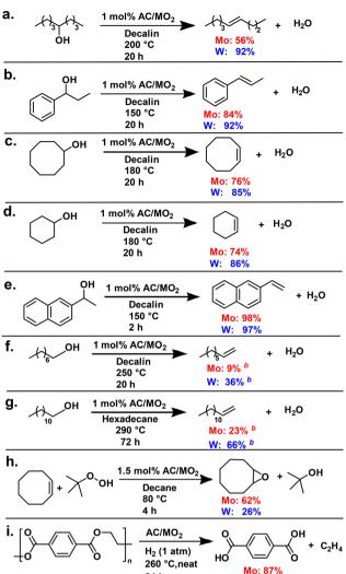
Scheme 2 Activity of AC/WO2 compared to AC/MoO2 for (a)-(g) dehydration (h) alkene epoxidation, and deconstruction.<sup>a</sup> <sup>a</sup>Yields quantified using <sup>1</sup>H HMR with mesitylene as internal standard. bMixture of isomers.
