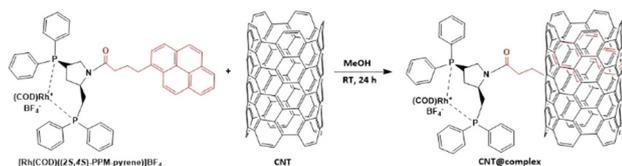
Scheme 2 Immobilization of the [Rh(COD)((2*S*,4*S*)-PPM-pyrene)]BF<sub>4</sub> complex onto CNTs.
