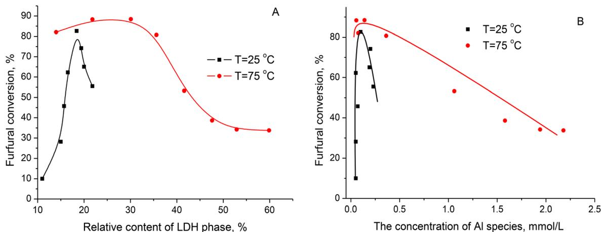
**Fig. 8** Change in furfural conversion observed over catalysts hydrated at  $T = 25\text{ °C}$  or  $75\text{ °C}$  after 60 minutes of aldol condensation depending on the relative content of LDH phase in the samples (A) and concentration of water-soluble Al species (B).
