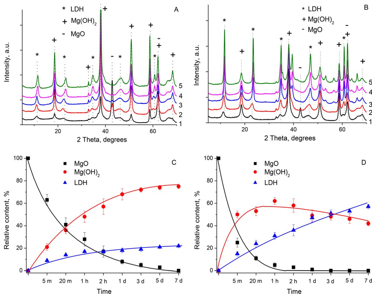
**Fig. 1** XRD patterns of materials prepared by the hydration treatment of pre-calcined MgO + Al<sub>2</sub>O<sub>3</sub> physical mixture at  $T = 25$  °C (A) and 75 °C (B). Hydration time: 1–5 minutes; 2–2 hours; 3–1 day; 4–3 days; and 5–7 days. Relative content of crystalline phases in the samples prepared at  $T = 25$  °C (C) and 75 °C (D).
