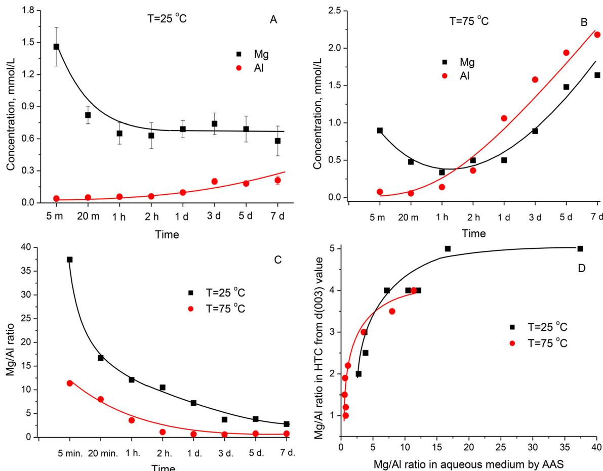
Fig. 3 Concentration of Mg and Al determined by AAS in the aqueous phase during the hydration of MgO + Al<sub>2</sub>O<sub>3</sub> mixture at  $T = 25\text{ }^{\circ}\text{C}$  (A) and  $75\text{ }^{\circ}\text{C}$  (B) as well as change in the Mg/Al ratio in the aqueous phase (C) as a function of hydration time. Dependence of Mg/Al ratio in the LDH phase (evaluated from  $d(003)$  values) on the Mg/Al ratio in the aqueous phase (D).
