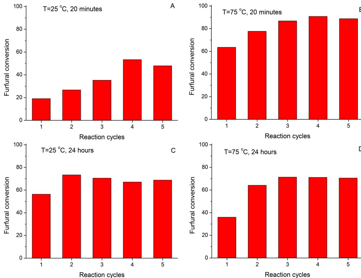
Fig. 9 Furfural conversion after 20 minutes of aldol condensation over different hydrated MgAl catalysts (atomic ratio Mg/Al = 3) in successive reaction cycles at  $T_{\text{reac.}} = 25\text{ }^{\circ}\text{C}$ . Hydration conditions: A – 20 min at 25 °C (S25-20m-*Rm* series), B – 20 min at 75 °C (S75-20m-*Rm* series), C – 24 hours at 25 °C (S25-24h-*Rm* series), and D – 24 hours at 75 °C (S75-24h-*Rm* series).
