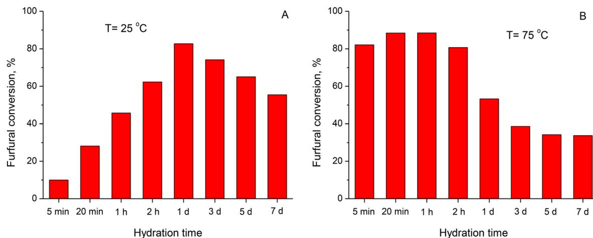
**Fig. 7** Furfural conversion after 60 minutes of aldol condensation over MgAl catalysts (atomic ratio Mg/Al = 3) hydrated at  $T = 25\text{ °C}$  (A) and  $75\text{ °C}$  (B) as a function of hydration time. The mass of the MgAl physical mixture used for the calcination/hydration steps was 1.0 g. Reaction conditions:  $T_{\text{reac.}} = 25\text{ °C}$ , furfural mass = 11.5 g, acetone mass = 35 g, F : Ac = 1 : 5 (mol/mol), and RPM = 250.
