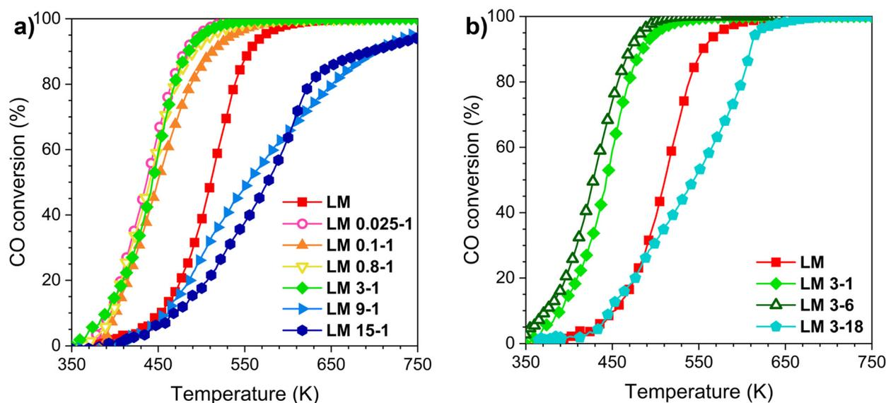
Fig. 6 Catalytic activity during the second cycle of CO oxidation with acid treated  $LaMnO_3$  samples as catalysts: in a) LM samples treated with different acid concentrations; in b) LM samples treated for different times.
