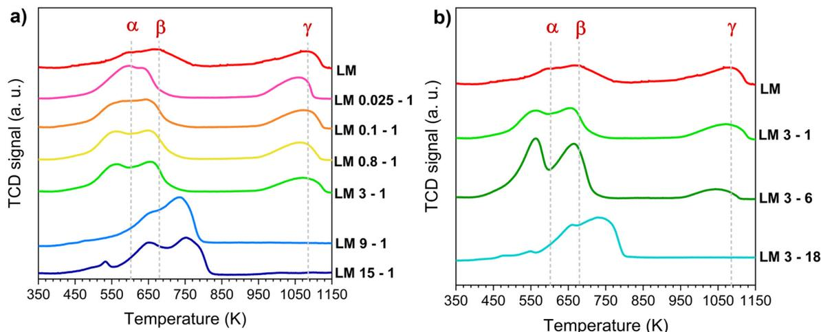
Fig. 4 Temperature-programmed reduction profiles of acid treated  $\text{LaMnO}_3$  samples: in a) LM samples treated with different acid concentrations; in b) LM samples treated for different times. TPR experiments were run on calcined samples.
