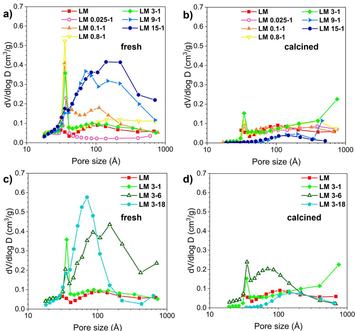
**Fig. 1** Pore distribution of acid treated  $\text{LaMnO}_3$  samples: in a) fresh LM samples (*i.e.*, after the acid treatment) treated with different acid concentrations; in b) the corresponding calcined samples (*i.e.*, after a calcination of 1 hour at 823 K in static air); in c) fresh LM samples treated by variation the duration of the treatment; in d) the corresponding calcined samples.
