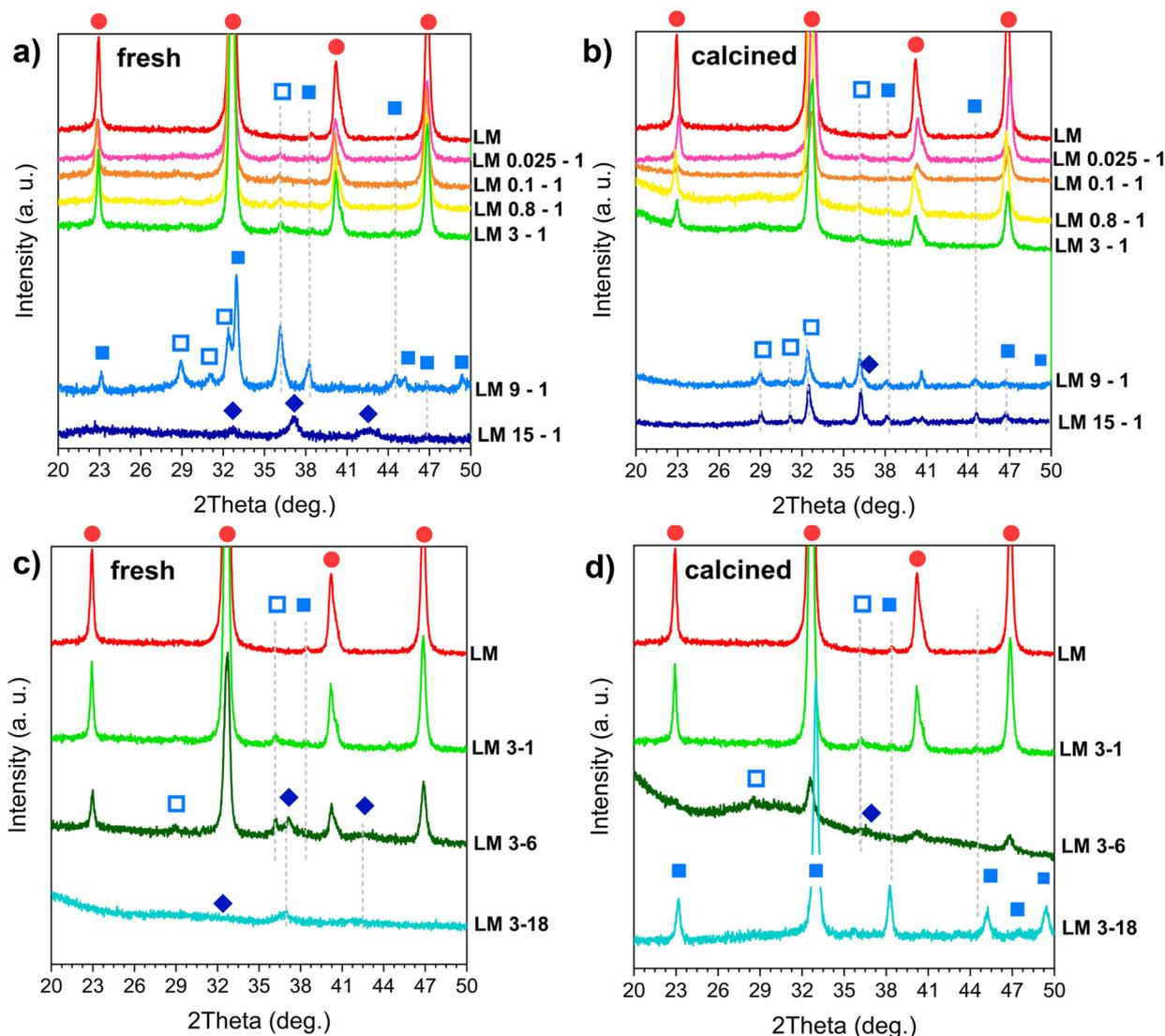
Fig. 2 X-ray diffractograms between 20–50 degrees of acid treated  $\text{LaMnO}_3$  samples: in a) fresh LM samples treated with different acid concentrations; in b) the corresponding calcined samples; in c) fresh LM samples treated by variation the duration of the treatment; in d) the corresponding calcined samples. ●:  $\text{LaMnO}_3$ ; ◆:  $\text{MnO}_2$ ; ■:  $\text{Mn}_2\text{O}_3$ ; □:  $\text{Mn}_3\text{O}_4$ .
