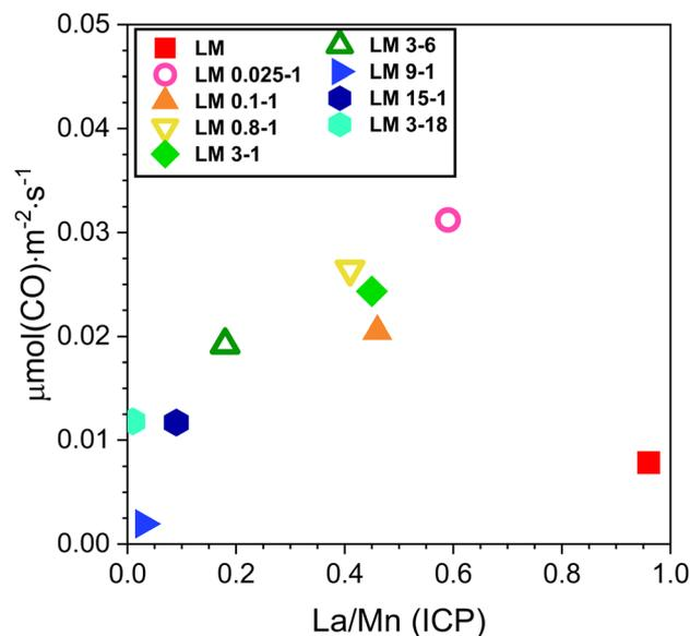
Fig. 8 Specific CO oxidation rate calculated at 390 K as a function of La/Mn molar ratio.
