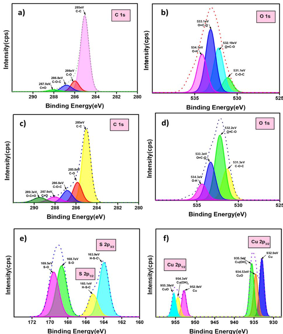
Fig. 3 XPS spectrum: OPL-CNS (a and b) for C 1s and O 1s, respectively, and Cu/TF-CNS (c–f) for C 1s, O 1s, S 2p and Cu 2p, respectively.
