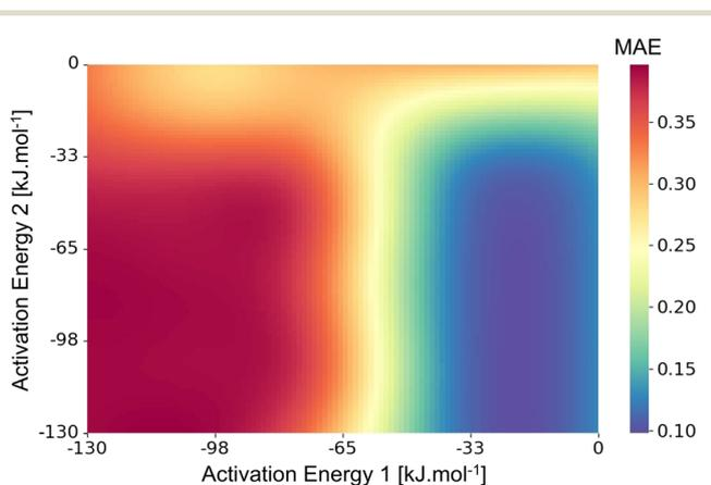
Fig. 4 Illustration of the objective function value (to minimize) along two exemplary dimensions (activation energies of  $\beta$ -scissions) visualizing the plateaus typically occurring when optimizing kinetic parameters.
