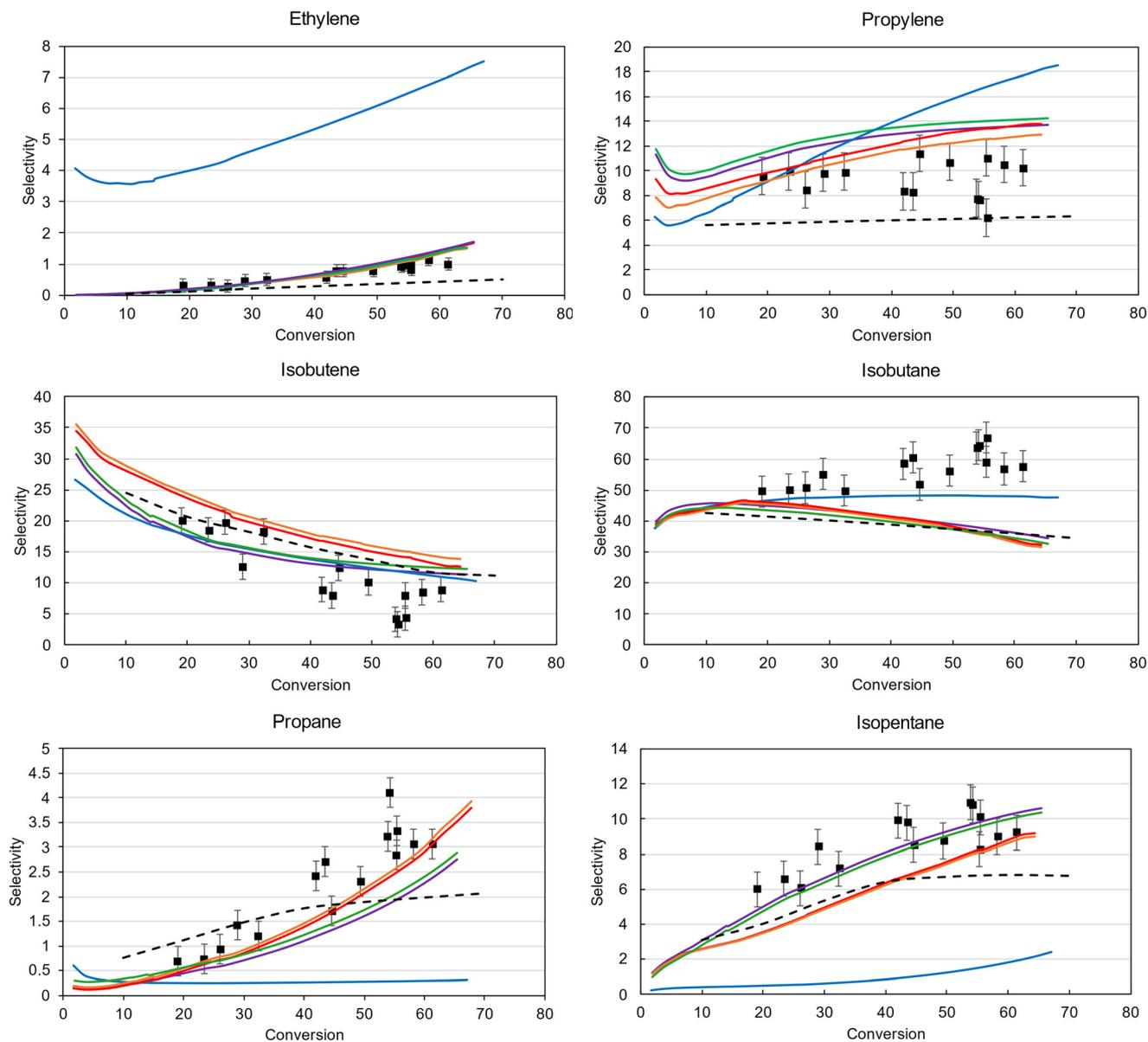
**Fig. 6** Experimental (markers) vs. modeled (lines) selectivities obtained by Levenberg–Marquardt (blue), RBF EI (orange), RQ-Matérn EI (red), RBF exploitative-EI (green), RQ-Matérn exploitative-EI (purple), and the reference kinetic model (dashed) of the main cracking products of ethylene, propylene, isobutene, isobutane, propane and isopentane for iso-octane catalytic cracking in LZ20 as a function of conversion.
