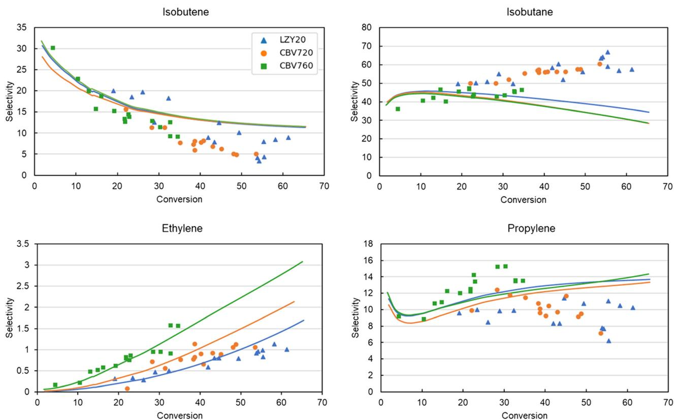
**Fig. 8** Experimental (markers) vs. modeled (lines) selectivities of the main cracking products of iso-octane in LZY20, CBV720, and CBV760 as a function of conversion.
