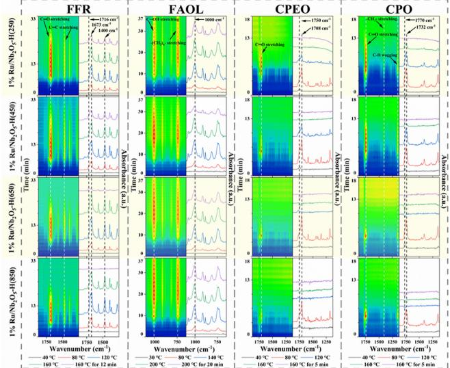
Fig. 4 Time-resolved in situ DRIFT spectra for FFR, FAOL, CPEO, and CPO adsorption over various 1% Ru/Nb<sub>2</sub>O<sub>5</sub> catalysts reduced at varied temperatures. Note: FAOL was subjected to programmed heating to 200 °C, for detailed conditions see Fig. S5-S8.†
