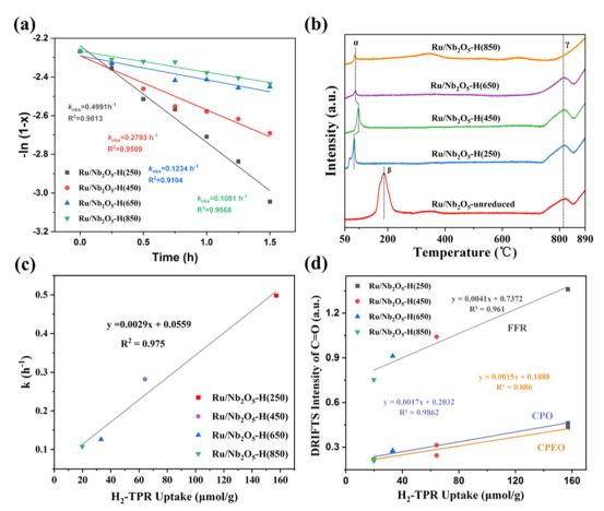
Fig. 3 (a) Kinetic fitting curves of kinetic data of the Ru/Nb<sub>2</sub>O<sub>5</sub> catalyst, x stands for FFR conversion; (b) H<sub>2</sub>-TPR profiles for 1% Ru/Nb<sub>2</sub>O<sub>5</sub> catalysts with varied reduction temperatures; (c) the fitting curves of  $H_2$ -TPR uptake of the  $\alpha$  peak and FFR reaction rate constant; (d) the fitting curves of H<sub>2</sub>-TPR uptake and the intensity of C=O adsorption of furfural.
