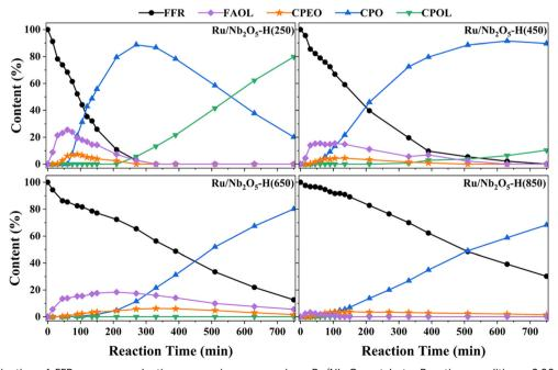
Fig. 2 Catalytic kinetics of FFR aqueous reductive conversion over various Ru/Nb₂O₅ catalysts. Reaction conditions: 2.00 g furfural, 0.40 g catalyst, 200 mL of H<sub>2</sub>O, p (initial, H<sub>2</sub>) = 5.0 MPa, the initial reaction temperature is 25 °C, T = 160 °C, heating rate = 4.5 °C min<sup>-1</sup>, stirring speed = 800 rpm, reaction time = 720 min.
