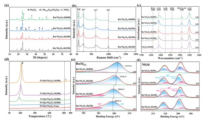
Fig. 1 Material characterization of various 1% Ru/Nb<sub>2</sub>O<sub>5</sub> catalysts reduced at varied temperatures. (a) XRD patterns, (b) Raman spectra, (c) Py-IR spectra at a desorption temperature of 150 °C, (d) H<sub>2</sub>-TPR profile, XPS results and peak fitting curves of (e) Ru3d and (f) Nb3d.
