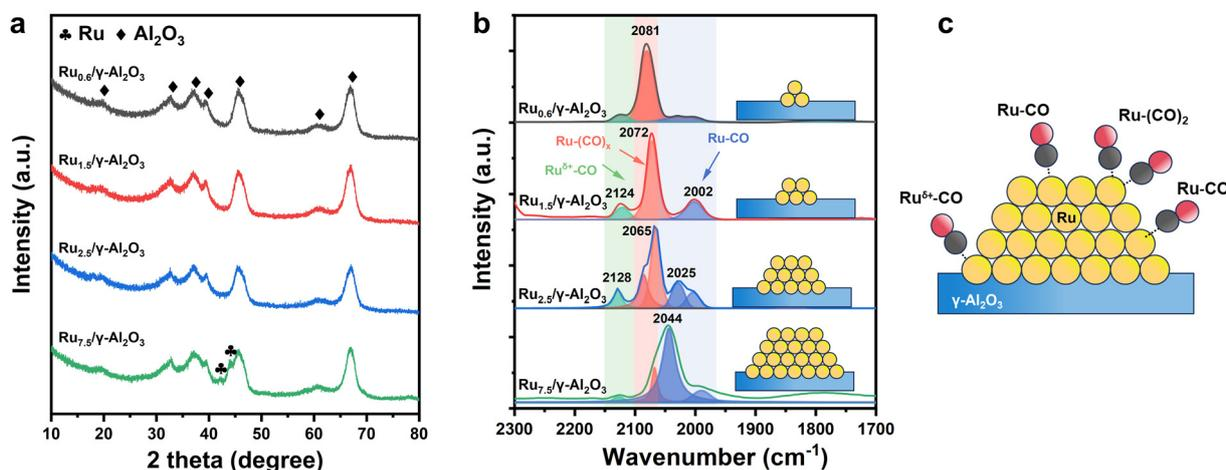
Fig. 2 a. XRD patterns of Ru/γ-Al<sub>2</sub>O<sub>3</sub> catalysts (♣ represents Ru, ♦ represents Al<sub>2</sub>O<sub>3</sub>); b. CO-DRIFTS and fitting result of Ru/γ-Al<sub>2</sub>O<sub>3</sub> catalysts; c. adsorption configurations of CO on Ru/γ-Al<sub>2</sub>O<sub>3</sub> catalysts. All the catalysts are pre-reduced at 200 °C for 2 h.
