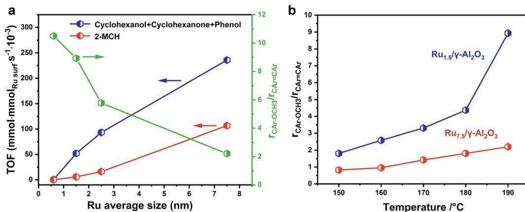
Fig. 5 a. The surface molar<sub>Ru</sub>-specific activity (turnover frequency, TOF) as a function of Ru particle size and the relative ratio of  $r_{\text{CAr-OCH}_3}$  and  $r_{\text{CAr=C}_{\text{Ar}}}$  of guaiacol; b. the  $r_{\text{CAr-OCH}_3}/r_{\text{CAr=C}_{\text{Ar}}}$  of Ru<sub>1.5</sub>/γ-Al<sub>2</sub>O<sub>3</sub> and Ru<sub>7.5</sub>/γ-Al<sub>2</sub>O<sub>3</sub> as a function of temperature.
