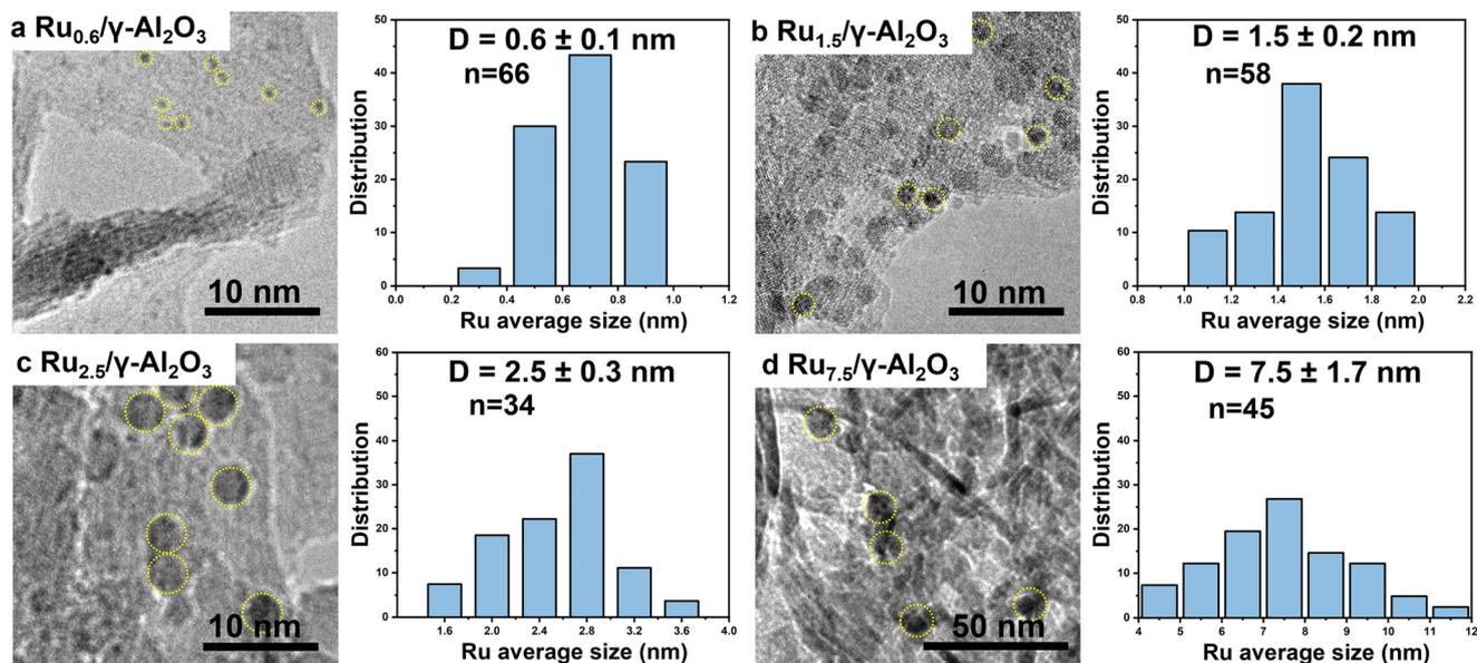
Fig. 1 TEM images and statistics particle size distribution bar charts of Ru/γ-Al<sub>2</sub>O<sub>3</sub> catalysts with different Ru particle sizes. a. Ru<sub>0.6</sub>/γ-Al<sub>2</sub>O<sub>3</sub>; b. Ru<sub>1.5</sub>/γ-Al<sub>2</sub>O<sub>3</sub>; c. Ru<sub>2.5</sub>/γ-Al<sub>2</sub>O<sub>3</sub>; d. Ru<sub>7.5</sub>/γ-Al<sub>2</sub>O<sub>3</sub> catalysts. All the catalysts were pre-reduced at 200 °C for 2 h.
