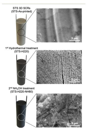
Fig. 2 Photographs and SEM images of STS 3D SCRs before and after each treatment step. The scan speed for the 3D printing process is 1200 mm s<sup>-1</sup>.
