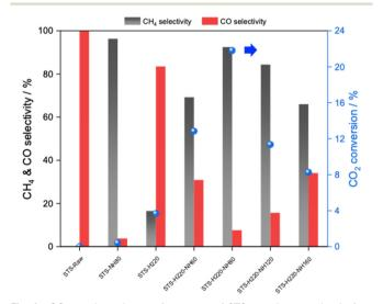
Fig. 1 CO<sub>2</sub> methanation performance of STS powder samples before and after each treatment step. Reaction conditions: T = 300 °C, P = 1bar, flow rate = 20 mL min<sup>-1</sup>, reaction gas =  $H_2/CO_2/N_2 = 64/16/20$ .
