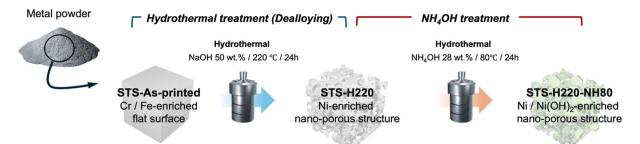
Scheme 1 Two-step surface functionalization method of STS metal powder and 3D SCRs.
