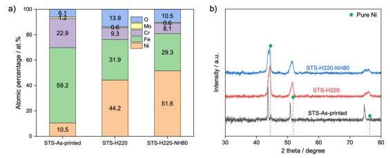
Fig. 3 a) EDS quantification and b) XRD profiles of STS 3D SCRs before and after each treatment step.
