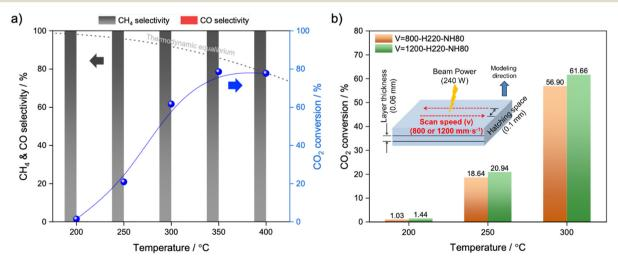
Fig. 4 a) Temperature-dependent  $CO_2$  conversion with v = 1200-H220-NH80 and b)  $CO_2$  methanation performance with different scan speeds. Reaction conditions: P = 1 bar, flow rate = 20 mL min<sup>-1</sup>, reaction gas =  $H_2/CO_2/N_2 = 64/16/20$ .
