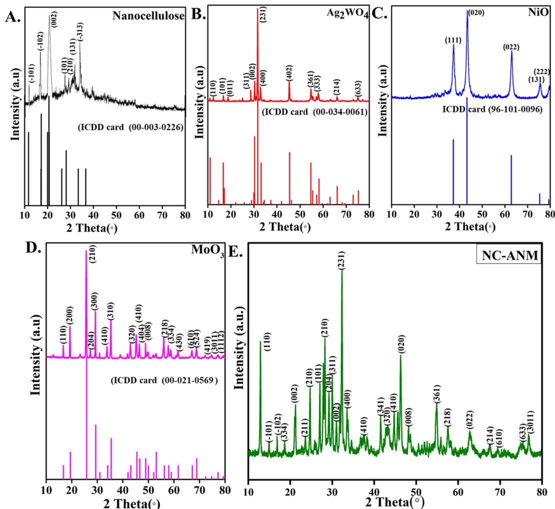
Fig. 2 XRD patterns of (A) nanocellulose, (B)  $\text{Ag}_2\text{WO}_4$ , (C) NiO, and (D)  $\text{MoO}_3$  along with their respective ICDD references, confirming their crystallographic structures and phase purity; (E) XRD pattern of the NC-ANM heterojunction, showing the characteristic peaks of all individual components, indicative of successful heterojunction formation.
