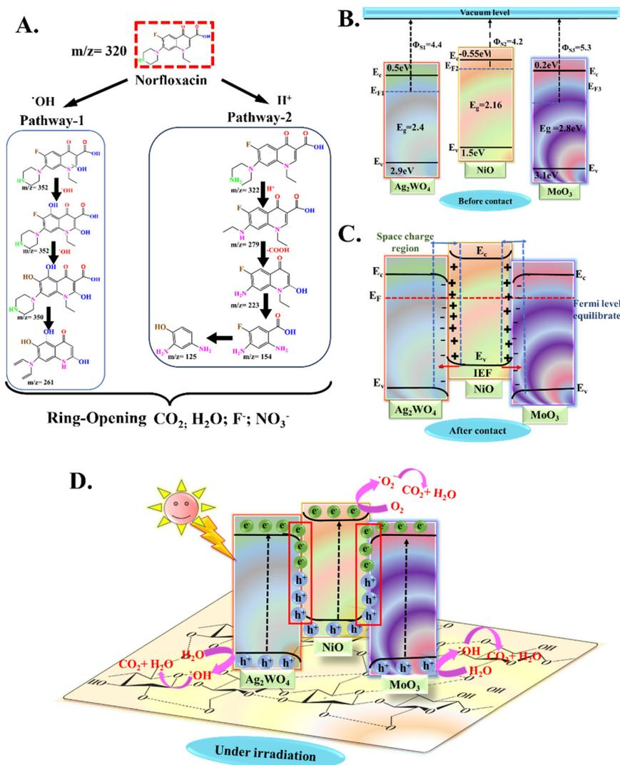
Fig. 7 (A) Proposed photodegradation pathways of NFX involving  $\cdot OH$  radical attack (pathway 1) and  $H^+$  ion attack (pathway 2); (B–D) schematic illustration of the S-scheme charge transfer mechanism in the NC-ANM heterojunction, highlighting the generation of reactive oxygen species ( $\cdot OH$  and  $\cdot O_2^-$ ) and their role in NFX degradation.
