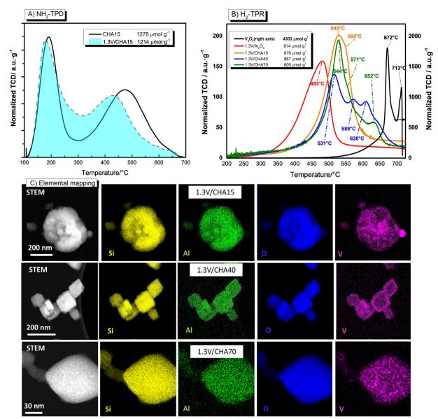
Fig. 1 A)  $NH_3$ -TPD comparison of CHA15 zeolite support before and after the impregnation of 1.3 mmol  $q^{-1}$  vanadium. B)  $H_2$ -TPR profiles for the zeolites (left-hand axis) and for bulk  $V_2O_5$  (right-hand axis). C) STEM images and elemental EDS mapping (Si, Al, O, and V) for 1.3 V/CHA15, 1.3VCHA40, and V.3VCHA70.
