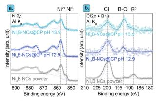
Fig. 5 XPS spectra of the (a) Ni 2p and (b) Cl 2p/B 1s core level regions of Ni<sub>3</sub>B NCs powder (grey), Ni<sub>3</sub>B-NCs@CP after the electrocatalytic test at pH 12.9 (purple), and at pH 13.9 (blue). Data of Ni<sub>3</sub>B NCs powder was reproduced with permission under a Creative Commons CC-BY 4.0 from Hong et al. 62 Copyright 2023 Americal Chemical Society.
