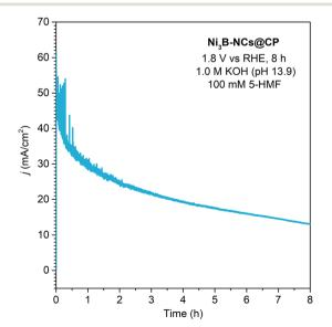
Fig. 11 Chronoamperometry of Ni<sub>3</sub>B-NCs@CP (0.05 mg cm<sup>-2</sup>) conducted at constant potential of 1.8 V vs. RHE for 8 h in the presence of 5-HMF (100 mM) at pH 13.9 (1.0 M KOH).
