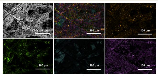
Fig. 13 SEM and EDS analysis of Ni<sub>3</sub>B-NCs@CP (initial loading: 0.05 mg cm<sup>-2</sup>) after 3 runs of 5-HMF electrochemical oxidation at 1.8 V vs. RHE for
