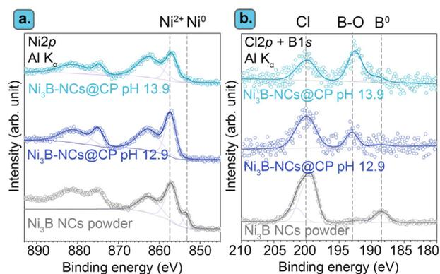
**Fig. 5** XPS spectra of the (a) Ni 2p and (b) Cl 2p/B 1s core level regions of  $\text{Ni}_3\text{B NCs}$  powder (grey),  $\text{Ni}_3\text{B-NCs@CP}$  after the electrocatalytic test at pH 12.9 (purple), and at pH 13.9 (blue). Data of  $\text{Ni}_3\text{B NCs}$  powder was reproduced with permission under a Creative Commons CC-BY 4.0 from Hong *et al.*<sup>62</sup> Copyright 2023 American Chemical Society.
