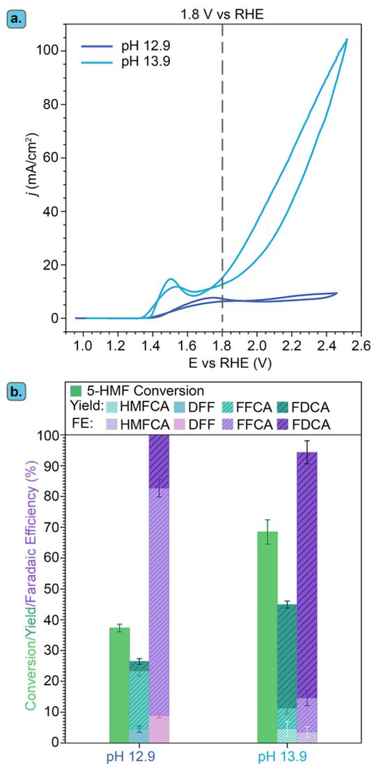
Fig. 6 Effect of pH (12.9 and 13.9) on the electrocatalytic performance of Ni<sub>3</sub>B-NCs@CP. (a) Cyclic voltammetry of Ni<sub>3</sub>B-NCs@CP at pH 12.9 (dark blue) and pH 13.9 (light blue) in the presence of 5-HMF. (b) Conversion, product yields and Faradaic efficiency (FE) obtained after 3 h of electrochemical oxidation of 5-HMF (initial concentration: 100 mM) catalyzed by Ni<sub>3</sub>B-NCs@CP at a constant potential of 1.8 V vs. RHE.
