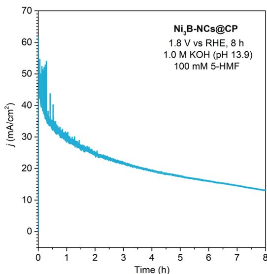
**Fig. 11** Chronoamperometry of  $\text{Ni}_3\text{B-NCs@CP}$  ( $0.05 \text{ mg cm}^{-2}$ ) conducted at constant potential of 1.8 V vs. RHE for 8 h in the presence of 5-HMF (100 mM) at pH 13.9 (1.0 M KOH).
