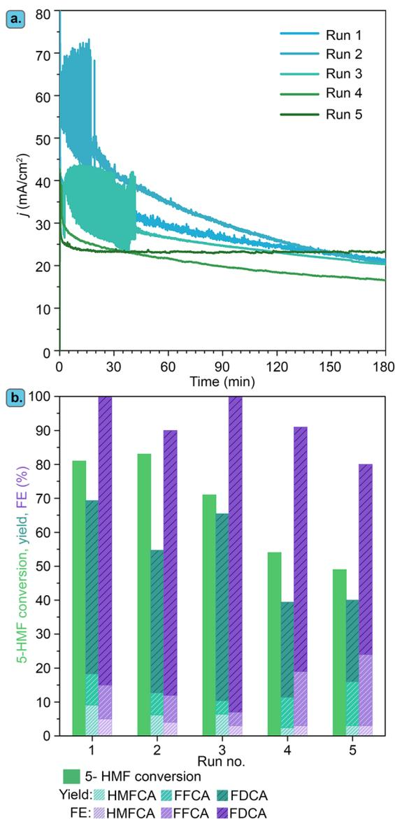
**Fig. 12** (a) Chronoamperometry of  $\text{Ni}_3\text{B-NCs@CP}$  ( $\sim 0.05 \text{ mg cm}^{-2}$ ) in 5 consecutive runs of electrochemical oxidation of 5-HMF (100 mM initial concentration) at constant potential of 1.8 V vs. RHE. (b) 5-HMF conversion, product yields and FE obtained at the end of each run of 5-HMF electrochemical oxidation with  $\text{Ni}_3\text{B-NCs@CP}$  as the electrocatalyst.
