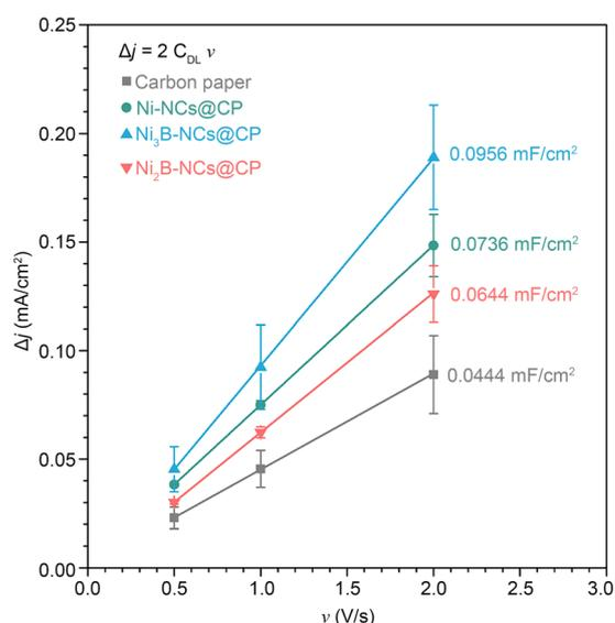
Fig. 10 Difference of anodic to cathodic current density plotted against the scan rate. From the value of slope of the plots ( $2C_{DL}\nu$ ), the double layer capacitance ( $C_{DL}$ ) can be calculated.
