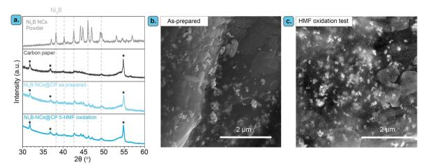
Fig. 4 Characterization of the Ni<sub>3</sub>B-NCs@CP electrocatalyst before and after chronoamperometric test (electrochemical oxidation of 5-HMF at 1.8 V vs. RHE for 3 h, 100 mM 5-HMF). (a) XRD pattern of Ni<sub>3</sub>B-NCs@CP as prepared and Ni<sub>3</sub>B-NCs@CP after the electrocatalytic test at pH 12.9. (b) SEM image of Ni<sub>3</sub>B-NCs@CP as prepared. (c) SEM image of Ni<sub>3</sub>B-NCs@CP after the electrocatalytic test at pH 12.9.
