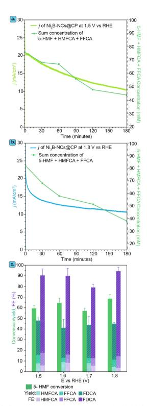
Fig. 8 Electrolysis of 5-HMF at different potentials in pH 13.9. Current density and sum of the concentrations of 5-HMF and reaction intermediates (green), measured during chronoamperometric tests of Ni<sub>3</sub>B-NCs@CP at a constant potential of (a) 1.5 V vs. RHE (light green line) and (b) 1.8 V vs. RHE (blue line). (c) Conversion, product yields and FE in the electrochemical oxidation of 5-HMF catalyzed Ni<sub>3</sub>B-NCs@CP after 3 h at different constant applied potentials.
