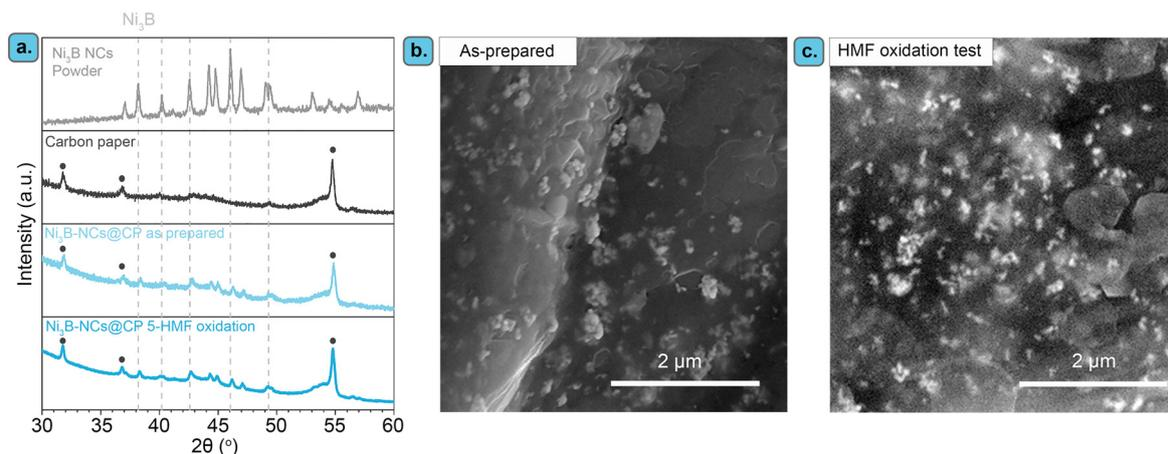
**Fig. 4** Characterization of the  $\text{Ni}_3\text{B-NCs@CP}$  electrocatalyst before and after chronoamperometric test (electrochemical oxidation of 5-HMF at 1.8 V vs. RHE for 3 h, 100 mM 5-HMF). (a) XRD pattern of  $\text{Ni}_3\text{B-NCs@CP}$  as prepared and  $\text{Ni}_3\text{B-NCs@CP}$  after the electrocatalytic test at pH 12.9. (b) SEM image of  $\text{Ni}_3\text{B-NCs@CP}$  as prepared. (c) SEM image of  $\text{Ni}_3\text{B-NCs@CP}$  after the electrocatalytic test at pH 12.9.
