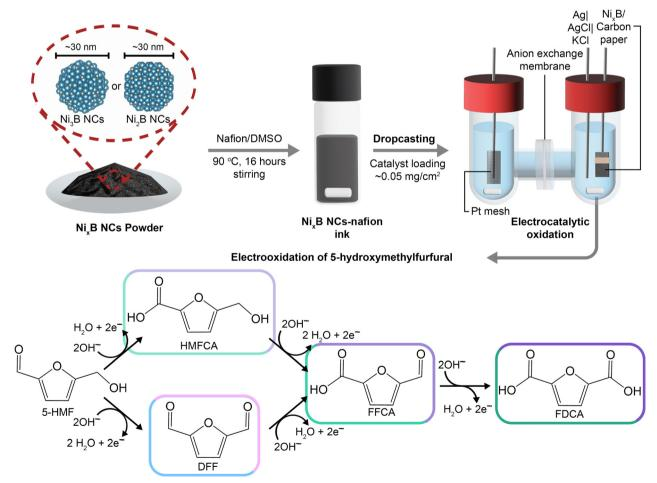
Fig. 1 Top: Schematic representation of the preparation and electrocatalytic testing process of Ni<sub>x</sub>B NCs. Bottom: Possible 5-HMF oxidation pathways towards FDCA. Note that since the reaction is carried out at high pH (12.9 or 13.9), the carboxyl groups will be mainly in their deprotonated form.
