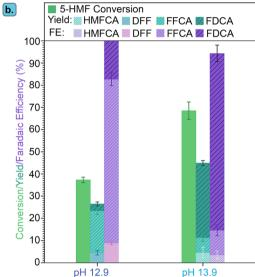
Fig. 6 Effect of pH (12.9 and 13.9) on the electrocatalytic performance of Ni $_3$ B-NCs@CP. (a) Cyclic voltammetry of Ni $_3$ B-NCs@CP at pH 12.9 (dark blue) and pH 13.9 (light blue) in the presence of 5-HMF. (b) Conversion, product yields and Faradaic efficiency (FE) obtained after 3 h of electrochemical oxidation of 5-HMF (initial concentration: 100 mM) catalyzed by Ni $_3$ B-NCs@CP at a constant potential of 1.8 V vs. RHE.
