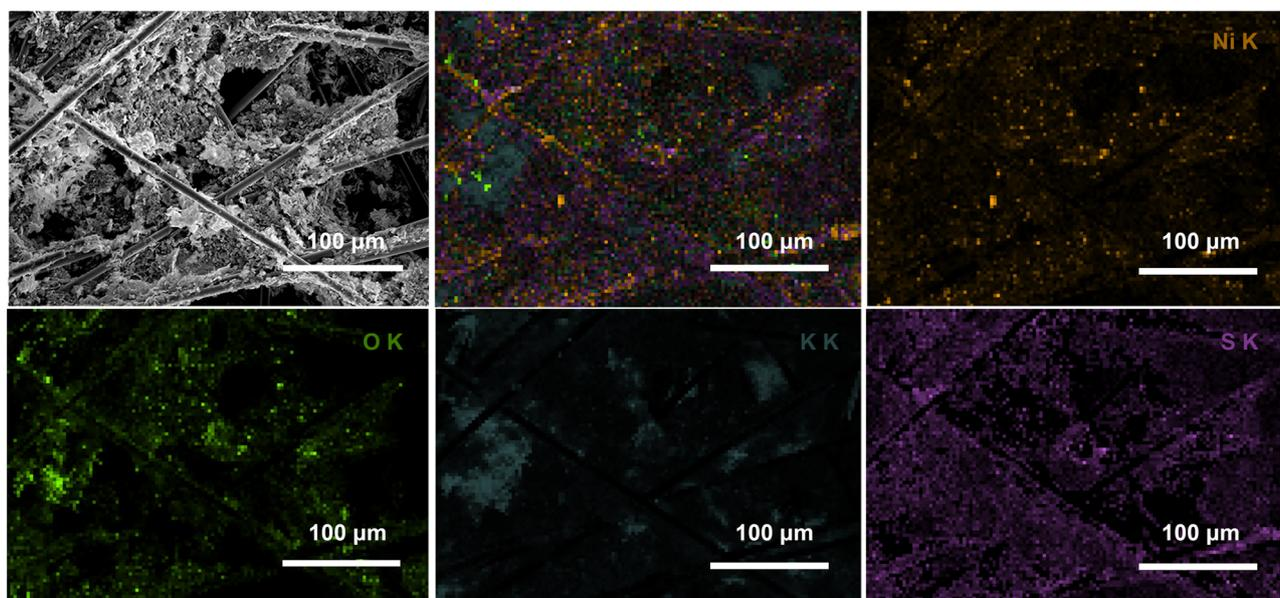
Fig. 13 SEM and EDS analysis of Ni<sub>3</sub>B-NCs@CP (initial loading: 0.05 mg cm<sup>-2</sup>) after 3 runs of 5-HMF electrochemical oxidation at 1.8 V vs. RHE for 3 h.
