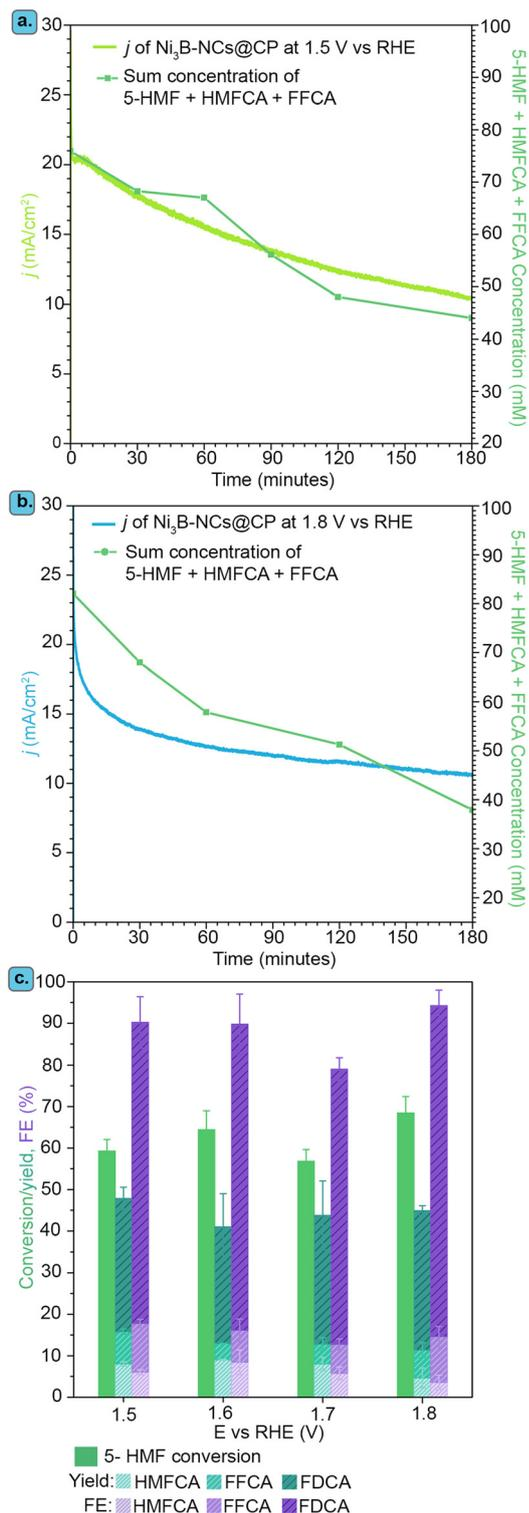
**Fig. 8** Electrolysis of 5-HMF at different potentials in pH 13.9. Current density and sum of the concentrations of 5-HMF and reaction intermediates (green), measured during chronoamperometric tests of Ni<sub>3</sub>B-NCs@CP at a constant potential of (a) 1.5 V vs. RHE (light green line) and (b) 1.8 V vs. RHE (blue line). (c) Conversion, product yields and FE in the electrochemical oxidation of 5-HMF catalyzed by Ni<sub>3</sub>B-NCs@CP after 3 h at different constant applied potentials.
