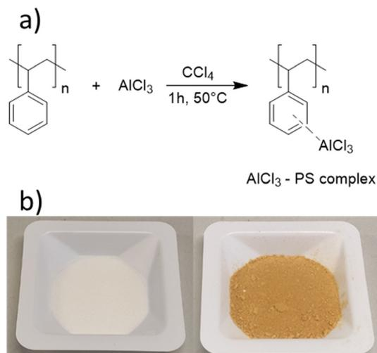
**Scheme 3** a) Reaction scheme for the immobilization of AlCl<sub>3</sub> in a porous polystyrene matrix *via* crosslinking. b) Photograph of the porous polystyrene before (left) and after (right) immobilization of AlCl<sub>3</sub>.
