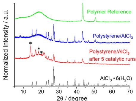
**Fig. 2** Normalized PXRD patterns of the polymer reference (green), the polystyrene/AlCl<sub>3</sub> composite before (blue) and after 5 catalytic runs (red); signals stemming from hydrolysis products Al(OH)<sub>3</sub> and Al(OH)<sub>2</sub>·2(H<sub>2</sub>O) are marked with an asterisk. The diffractogram of AlCl<sub>3</sub>·6(H<sub>2</sub>O) (ICSD-22071) is shown for comparison (black).
