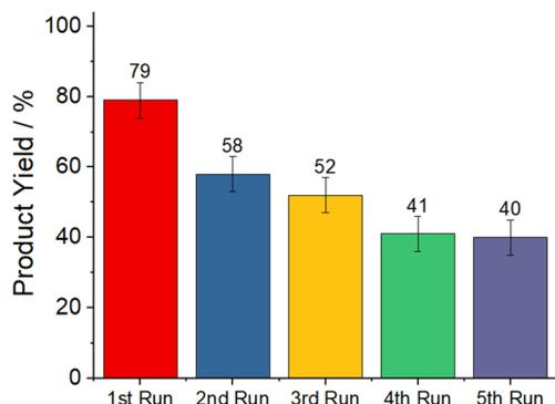
Fig. 4  $^1\text{H-NMR}$  determined yields of 5-phenyltetrazole with (reused) polystyrene-bound  $\text{AlCl}_3$  as heterogeneous catalyst. Conditions:  $160^\circ\text{C}$  for 6 hours, solvent free.
