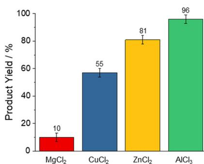
**Fig. 1** Yields of 5-phenyltetrazole with different Lewis acid catalysts at 160 °C for 16 h, as determined by <sup>1</sup>H-NMR spectroscopy.
