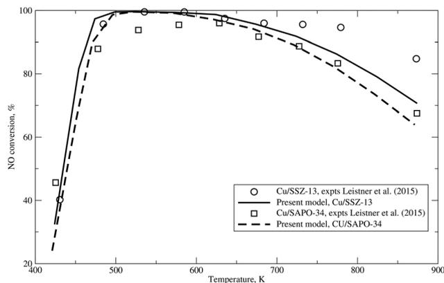
**Fig. 4** NO conversion vs. temperature for two copper-exchanged zeolites for SCR operation. The inlet gas composition is:  $x_{\text{NO}} = x_{\text{NH}_3} = 400$  ppm,  $x_{\text{O}_2} = 8\%$ ,  $x_{\text{H}_2\text{O}} = 5\%$  with the rest being  $\text{N}_2$ . The inlet gas velocity is  $8.4 \text{ cm s}^{-1}$ . Symbols are measurements of Leistner *et al.*<sup>43</sup>
