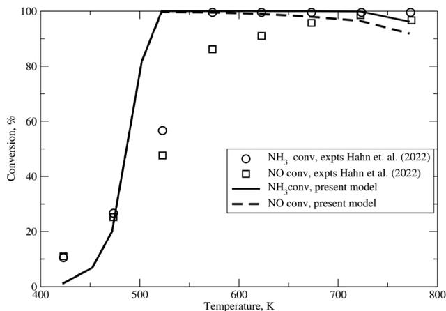
**Fig. 5**  $\text{NH}_3$  and NO conversion vs. temperature for SCR operation with Fe-exchanged HBEA zeolite, Hahn *et al.*<sup>14</sup> The inlet gas composition is:  $x_{\text{NO}} = x_{\text{NH}_3} = 500$  ppm,  $x_{\text{O}_2} = 5\%$ , with the rest being  $\text{N}_2$ . The inlet gas velocity is  $15.3 \text{ cm s}^{-1}$ ,  $\bar{S} = 2.46 \times 10^6 \text{ cm}^2$ , the initial catalyst loading is  $x_{\text{CatO}} = 0.008$ . Symbols are measurements of Hahn *et al.*<sup>14</sup>
