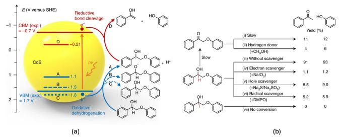
Scheme 2 (a) Proposed electron-hole coupled (EHCO) mechanism for CdS-catalysed C<sub>β</sub>-O bond cleavage of a dimeric β-O-4 lignin model compound through a C<sub>n</sub> radical intermediate: (b) the control experiments with various reactants or additives (this scheme has been reproduced from ref. 22 with permission from Nature Publication Group, copyright 2018).
