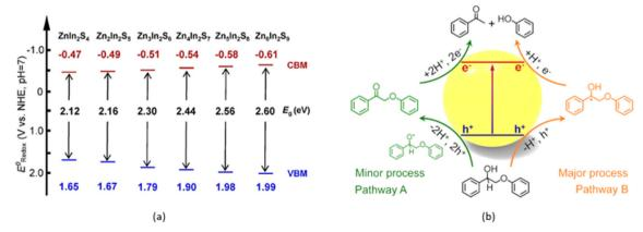
Scheme 4 (a) Band structure diagram of  $Zn_m ln_2 S_{m+3}$  (m = 1-6); (b) proposed photocatalytic mechanism for  $\beta$ -O-4 bond cleavage in 2-phenoxy-1phenylethanol over the  $Zn_4In_2S_7$  catalyst (this scheme has been reproduced from ref. 16 with permission from Wiley-VCH, copyright 2019).
