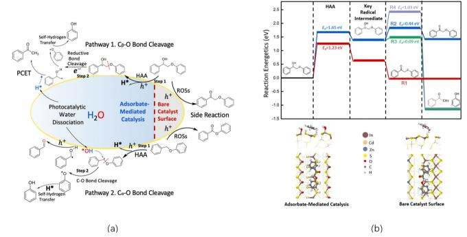
Scheme 5 (a) Proposed reaction mechanism for photocatalytic fragmentation of aryl ether C-O bonds in lignin model compounds over quaternary cadmium zinc indium sulphide photocatalysts; (b) the calculated reaction profiles of four different PP-ol conversion pathways in two different catalytic microenvironments (this scheme has been reproduced from ref. 68 with permission from Elsevier, copyright 2024).
