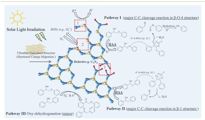
Scheme 13 Proposed mechanism of multi-defective  $g-C_3N_4$  photocatalysed cleavage of C-C bonds in  $\beta$ -O-4 and  $\beta$ -1 structures; the marked area 1, 2 and 3 represent the -C≡N, N vacancy and C vacancy, respectively (this scheme has been reproduced from ref. 90 with permission from Elsevier, copyright 2024).
