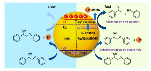
Scheme 3 Schematic representation comparing the fragmentation of the β-O-4 bond in Aq<sub>2</sub>S@CdS (yellow) with CdS (blue) (this figure has been reproduced from ref. 17 with permission from American Chemical Society, copyright 2020).
