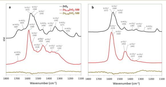
Fig. 6 DRIFT spectra of (a) CO<sub>2</sub> adsorption at 325 °C and 10 bar on  $ZrO_2$ ,  $ZrO_2$ -500, and  $ZrO_3$ -500 after 40 minutes under 2 ml min<sup>-1</sup> CO<sub>2</sub> and 16 ml min<sup>-1</sup> Ar and (b) after 40 minutes evacuation at 325 °C and 10 bar under 16 ml min<sup>-1</sup> Ar (m: monodentate, b: bidentate, wi: weakly interacting, and p: polydentate species).
