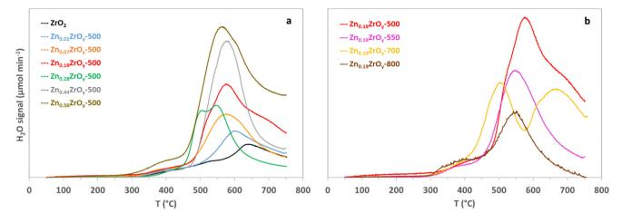
Fig. 4 Temperature-programmed H<sub>2</sub> reduction of (a) Zn<sub>x</sub>ZrO<sub>v</sub>-500 catalysts and (b) Zn<sub>0.19</sub>ZrO<sub>v</sub>-T calcined at 500, 550, 700, and 800 °C.
