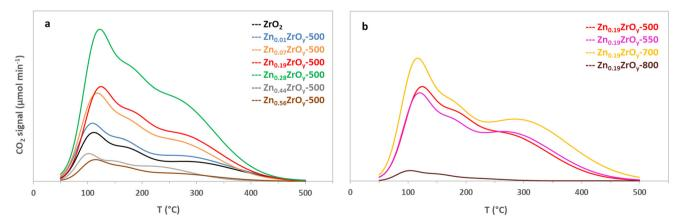
Fig. 5 Temperature-programmed CO<sub>2</sub> desorption of (a) Zn<sub>x</sub>ZrO<sub>y</sub>-500 catalysts and (b) Zn<sub>0.19</sub>ZrO<sub>y</sub>-T calcined at 500, 550, 700, and 800 °C.
