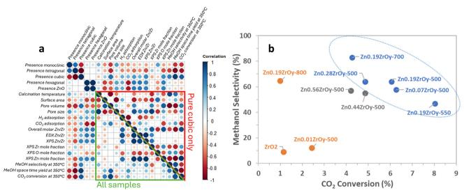
Fig. 9 (a) Surface property correlations and CTM catalysis within all samples and (b) methanol selectivity versus CO2 conversion at 350 °C, 45 bar,  $H_2: CO_2: Ar = 3:1:1$ , and GHSV = 21 000 Nml  $g_{cat}^{-1} h^{-1}$  (blue colour: pure cubic-phase, grey colour: cubic-phase + h-ZnO, and orange colour: the rest of the samples).
