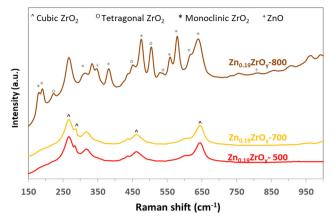
Fig. 2 Raman spectra of Zn<sub>0.19</sub>ZrO<sub>v</sub>-T calcined at 500, 700, and 800 °C.
