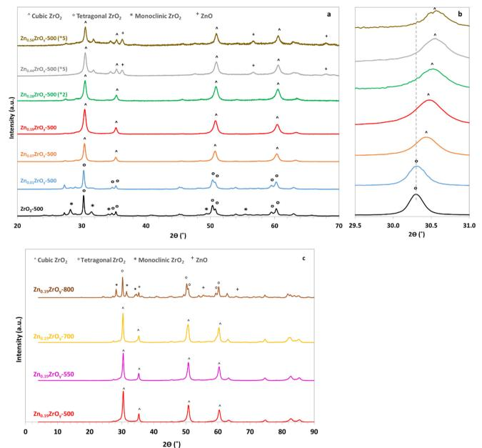
Fig. 1 (a) XRD patterns of  $Zn_xZrO_y$ -500 catalysts, (b) enlarged XRD patterns of  $Zn_xZrO_y$ -500 catalysts in the  $2\theta$  range of 29.5–31.0°, and (c) XRD patterns of Zn<sub>0.19</sub>ZrO<sub>v</sub>-T calcined at 500, 550, 700, and 800 °C (m-ZrO<sub>2</sub>: PDF card 81.1314, t-ZrO<sub>2</sub>: PDF card 50-1089, c-ZrO<sub>2</sub>: PDF card 65-0461, and h-ZnO: PDF card 05-0664).
