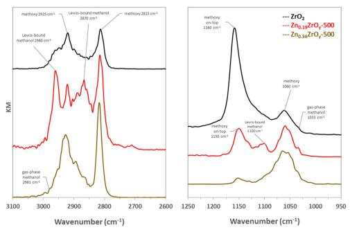
Fig. 7 DRIFT spectra of methanol adsorption at 200 °C and 10 bar on ZrO<sub>2</sub>, Zn<sub>0.19</sub>ZrO<sub>y</sub>-500, and Zn<sub>0.56</sub>ZrO<sub>y</sub>-500 (the spectra were recorded after evacuation of physically adsorbed species under a flow of 130 ml min<sup>-1</sup> Ar).
