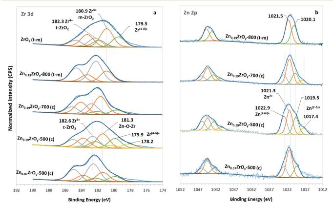
Fig. 3 XPS spectra of (a) Zr 3d in ZrO<sub>2</sub>, Zn<sub>0.07</sub>ZrO<sub>y</sub>-500, Zn<sub>0.19</sub>ZrO<sub>y</sub>-500, Zn<sub>0.19</sub>ZrO<sub>y</sub>-700, and Zn<sub>0.19</sub>ZrO<sub>y</sub>-800 and (b) Zn 2p in Zn<sub>0.07</sub>ZrO<sub>y</sub>-500, Zn<sub>0.19</sub>ZrO<sub>y</sub>-500, Zn  $Zn_{0.19}ZrO_{v}$ -500,  $Zn_{0.19}ZrO_{v}$ -700, and  $Zn_{0.19}ZrO_{v}$ -800.
