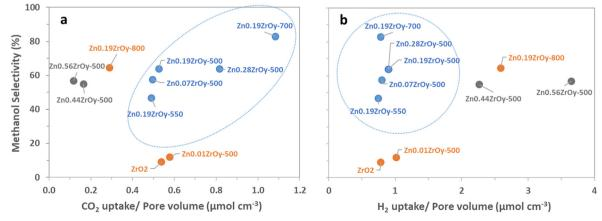
Fig. 10 Effect of pore-volume normalized (a) CO<sub>2</sub> uptake and (b) H<sub>2</sub> uptake on methanol selectivity at 350 °C, 45 bar, H<sub>2</sub>: CO<sub>2</sub>: Ar = 3:1:1, and GHSV = 21000 Nml  $g_{cat}^{-1}$  h<sup>-1</sup> (blue colour: pure cubic-phase, grey colour: cubic-phase + h-ZnO, and orange colour: the rest of the samples).
