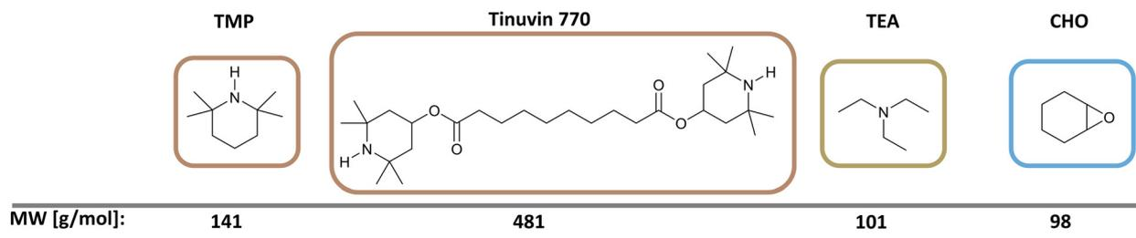
**Fig. 2** Three different stabilizers studied for their stabilizing effect on Biphephos. 2,2,6,6-Tetramethylpiperidine (TMP) and Tinuvin® 770 are sterically hindered secondary amines, Et<sub>3</sub>N (TEA), and cyclohexene oxide (CHO).
