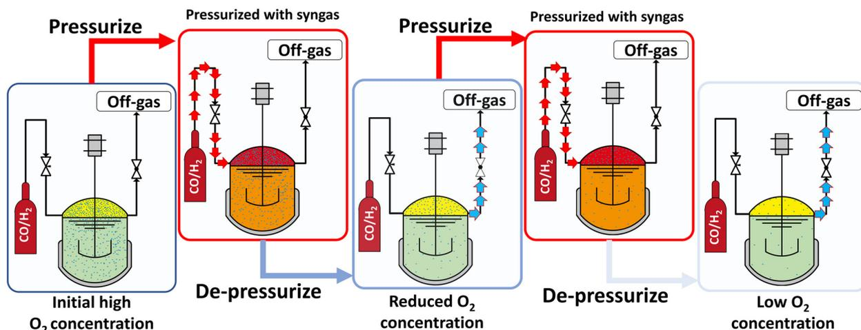
Fig. 7 A schematic representation of how a “pressure-de-pressurize” cycle helps to reduce the concentration of  $O_2$  present within the autoclave reactor after being charged with all the reaction mass.
