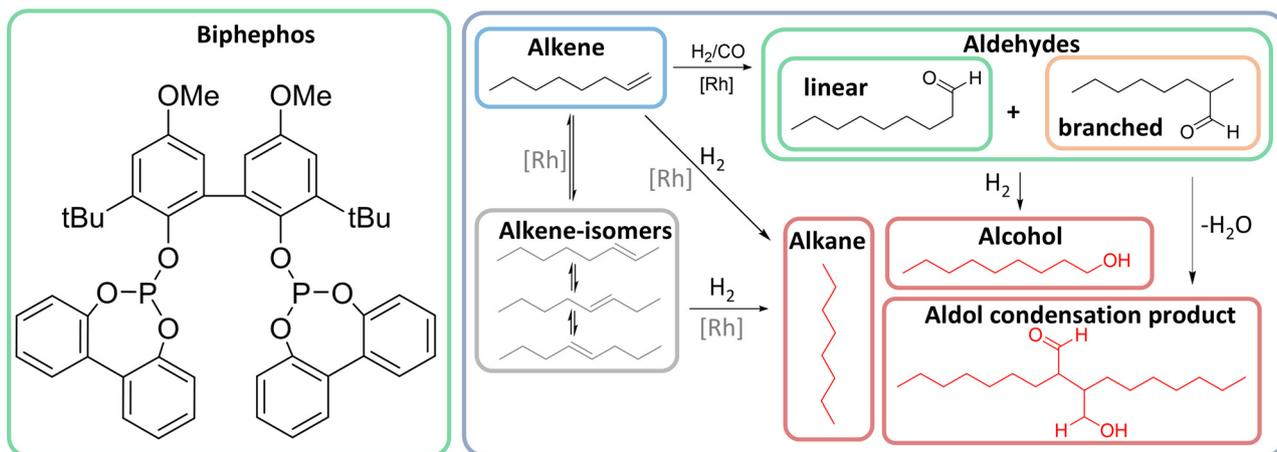
**Fig. 1** On the left side: the ligands Biphephos; on the right side: a reaction overview of Rh-catalyzed hydroformylation of a terminal alkene where the most desired product is the linear aldehyde. Hydrogenation products such as alkane and alcohols can be produced. Aldol condensation products from aldehydes can be formed.
