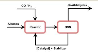
Fig. 9 Basic scheme of the nanofiltration membrane reactor miniplant. The catalyst complex remains in the reaction system.
