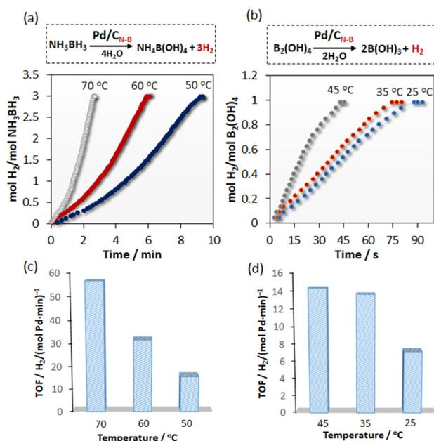
Fig. 3 Time plot of H<sub>2</sub> evolution from the hydrolysis of NH<sub>3</sub>BH<sub>3</sub> (a) and B<sub>2</sub>(OH)<sub>4</sub> (b), TOF values for 10% substrate conversion catalyzed by Pd/C<sub>N-B</sub> (c and d).
