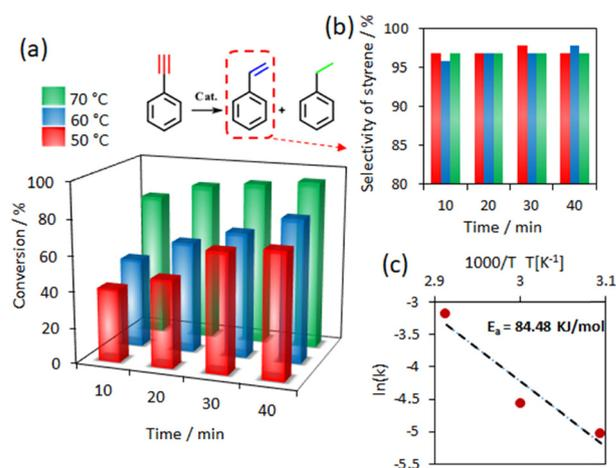
Fig. 4 The time profiles of conversion of phenylacetylene catalyzed by Pd/C<sub>N-B</sub>. Reaction conditions: 0.91 mmol of phenylacetylene, catalyst (1 mol% Pd), Pd : NH<sub>3</sub>BH<sub>3</sub> = 0.0091, 2 mL of H<sub>2</sub>O (a). Effect of reaction time on the selectivity of styrene (b) and Arrhenius plot of ln(*k*) versus 1000/*T* (c).
