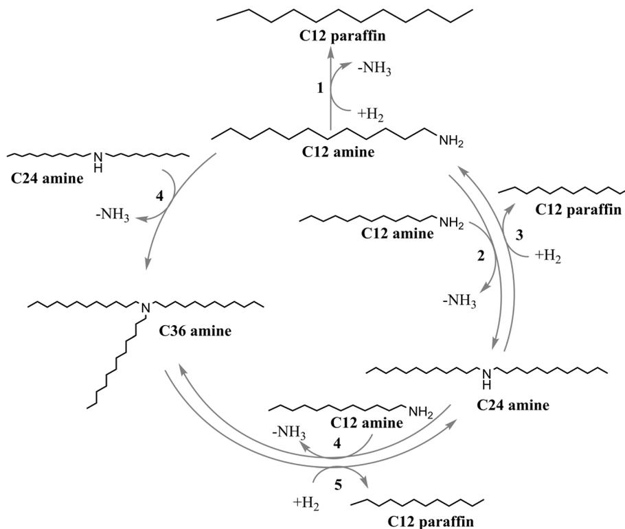
**Fig. 3** Reaction network for the hydrotreatment of primary amine (dodecylamine, C12 amine), secondary amine (didodecylamine, C24 amine) and tertiary amine (tridodecylamine, C36 amine) over Pt/ZrO<sub>2</sub>. The hydrotreatment of all three amines produces dodecane (C12 paraffin) as the final product. Reactions: 1 direct HDN of primary amine, 2 condensation of primary amine, 3 hydrogenolysis of secondary amine, 4 condensation of secondary amine, and 5 hydrogenolysis of tertiary amine.
