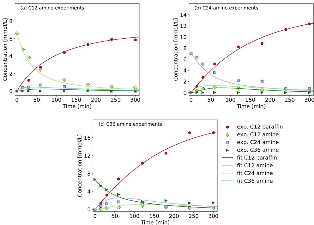
**Fig. 4** Experimental (exp.) data and simulated fit as concentration ( $\text{mmol L}^{-1}$ ) vs. reaction time (min) for (a) the primary amine experiments, (b) the secondary amine experiments, and (c) the tridodecylamine experiments. Experimental conditions: 300 °C, 80 bar  $\text{H}_2$ , 20 mg catalyst and 100 ppm initial nitrogen concentration.
