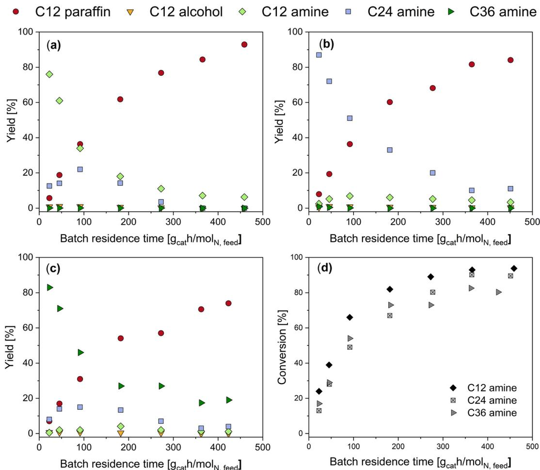
**Fig. 1** Carbon-based yields as a function of batch residence time ( $\text{g}_{\text{cat}} \text{h mol}_{\text{N, feed}}^{-1}$ ) for: (a) dodecylamine HDN experiments, (b) didodecylamine HDN experiments, (c) tri-dodecylamine HDN experiments, as well as conversion (%) as a function of batch residence time (d). Experimental conditions: 300 °C, 80 bar  $\text{H}_2$ , 20 mg catalyst and 100 ppm initial nitrogen concentration.
