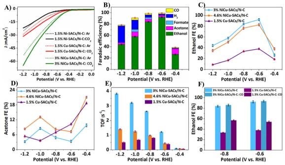
Fig. 26 (A) LSV curves of 3% NiCu-SACs/N in 0.5 M KHCO<sub>3</sub>. (B) FE% & product distribution on 3% NiCu-SACs/N-C. (C) FE% of ethanol, (D) FE% of acetone, and (E) TOF of ethanol over NiCu-SACs/N-C hybrids with different metal loadings at different applied potentials. (F) FE% of ethanol over 3% NiCu-SACs/N-C and 1.5% Cu-SACs/N-C. Reproduced with permission.<sup>236</sup> ©2024, Elsevier B.V.
