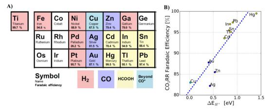
Fig. 5 (A) Major product classification of metal catalysts for ECR of CO2 obtained from other experimental data. (B) FE% of ECR of CO2 as a function of  $\Delta E_{H^*}$  (binding energy of H\*). Reproduced with permission.<sup>109</sup> ©John Wiley and Sons.
