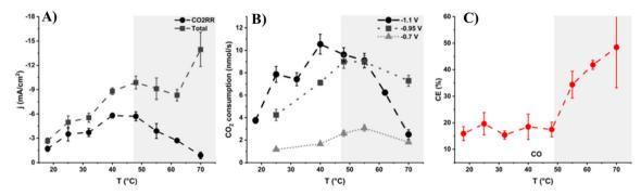
Fig. 17 (A) Total current density and current density toward ECR of CO<sub>2</sub> at -1.1 V vs. RHE, (B) total consumption of CO<sub>2</sub> during the reduction at different reaction temperatures in 0.1 M KHCO<sub>3</sub> at -1.1, -0.9, and -0.7 V vs. RHE, and (C) carbon efficiency toward CO at -1.1 V vs. RHE.
