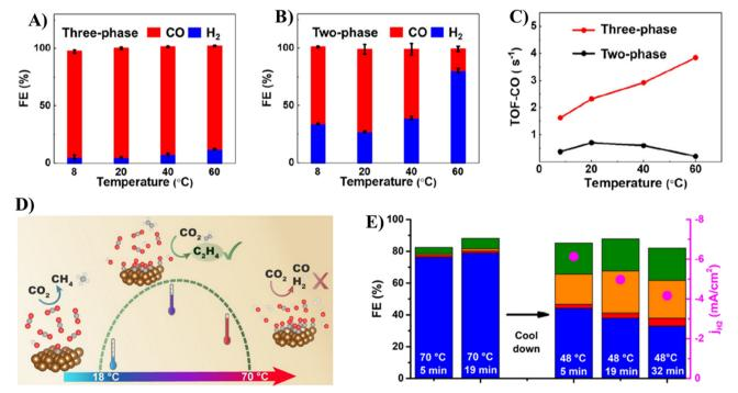
Fig. 20 (A and B) % FE for ECR of CO<sub>2</sub> evaluated at a potential of -0.7 V and different temperatures. (C) TOFs of CO production at a potential of -0.7 V. (D) Mechanisms for the selective changes in temperature-dependent products. (E) Comparison of the gaseous product % FE in ECR of CO<sub>2</sub> at 1.1 V with RHE at 70 °C after 5 and 19 min, and after cooling at 48 °C for 5, 19, and 32 min. The current density of the HER is indicated by the red dots (at 70 °C).51,204
