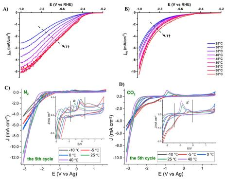
Fig. 18 Partial current density towards CO formation (A) and H<sub>2</sub> (B) at different temperatures in 0.1 M NaHCO<sub>3</sub> on a gold RRDE at 2500 rpm and 20 mV s<sup>-1,205</sup> Curves (the fifth cycle) of Pt in N<sub>2</sub> (C) and CO<sub>2</sub>-saturated, a (-2 to 2 V), (D) ionic liquid in the potential range of -3.1 to 1.7 V vs. Ag/ AgCl, a' (-2.5 to 2 V). Reproduced with permission. 206 ©2020, the American Chemical Society.
