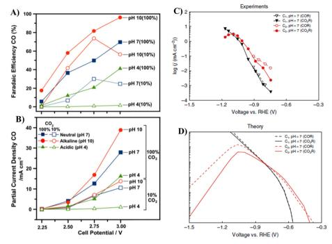
Fig. 15 (A) Faradaic efficiency for CO and (B) partial current density of CO as a function of cell potential for 3 different pH levels and two different CO<sub>2</sub> concentrations (10 and 100%). Comparison of ECR of CO<sub>2</sub> and CO at pH 7: (C) measured CO and CO<sub>2</sub> reduction activities toward C<sub>1</sub> and C<sub>2</sub> at pH = 7 and (D) theoretically predicted polarization curves of ECR of CO<sub>2</sub> and CO on Cu(211) at pH = 7.197
