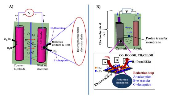
Fig. 1 (A) Principles of ECR of CO2 on the surface of heterogeneous electrocatalysts. (B) Detailed scheme showing the role of the anode and cathode in the reduction process.
