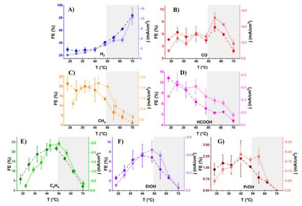
Fig. 16 Faradaic efficiency (in dark circles) and partial current density (in light squares) during ECR of CO<sub>2</sub> at different reaction temperatures in 0.1 M KHCO<sub>3</sub> at -1.1 V vs. RHE for (A) hydrogen, (B) CO, (C) methane, (D) formic acid, (E) ethylene, (F) ethanol, and (G) 1-propanol. The error bars are determined from at least 3 separate experiments. The gray background indicates the second regime, and the dotted lines are a guide to the eye.205
