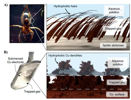
Fig. 13 (A) Diving bell spider for subaquatic breathing in and (B) on a hydrophobic dendritic cu surface for aqueous CO<sub>2</sub> reduction.<sup>178</sup>
