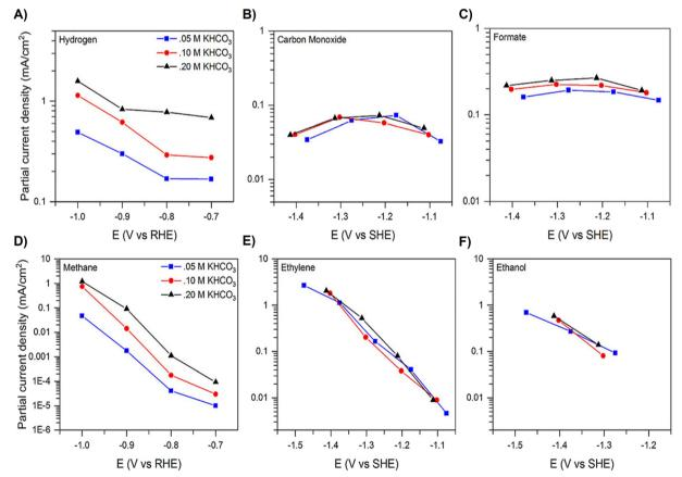
Fig. 8 (A-F) Impact of HCO<sub>3</sub><sup>-</sup> buffer concentration on the production of main products and generation of partial current for each of major products in ECR of CO<sub>2</sub> on Cu(100). The current density for each product is represented as a function of the bicarbonate buffer concentration in the electrolyte solution in the range of -0.7 and -1.0 V vs. RHE. Reproduced with permission. ©2018, Wiley-VCH Verlag GmbH & Co. KGaA,
