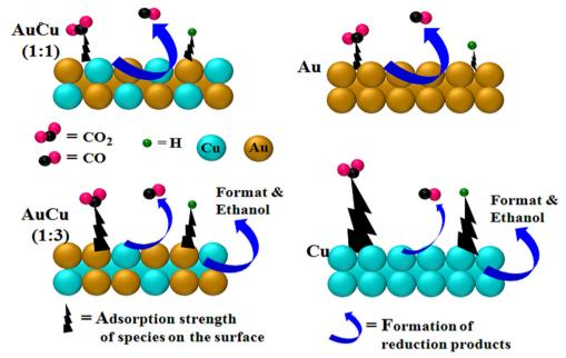
Fig. 31 Role of surface composition and type of electrocatalyst in reactivity and selectivity of ECR of CO<sub>2</sub>.
