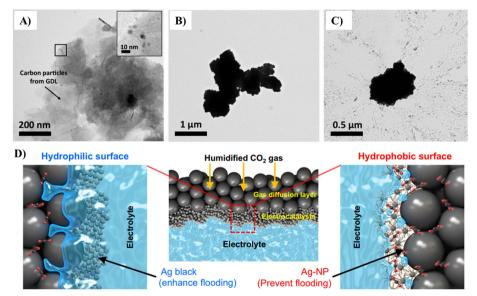
Fig. 12 Low-magnification TEM image of (A) Ag-NP, (B) Ag black, (C) and Ag-PTFE catalysts after the durability test at 3.4 V vs. RHE. (D) Schematic (low and high magnifications) of the triple-phase boundary for the hydrophilic Ag black and hydrophobic Ag-NP catalysts in the CO2 electrolyzer.176
