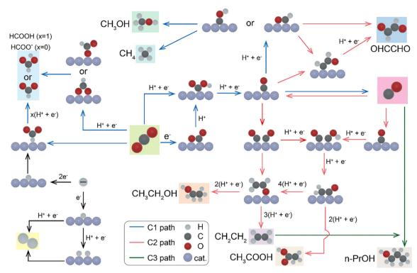
Fig. 2 Possible carbon dioxide reduction reaction pathways for C1 and C2 products. 69 ©Elsevier
