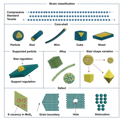
Fig. 28 Schematic of formation mechanisms and types of strains. 303
