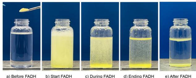
**Fig. 6** Photographs during the FA dehydrogenation with the release-and-catch catalytic system (Cp\*Ir-HMDAbpy@PAA). a) Before FA dehydrogenation, b) starting FA dehydrogenation, Cp\*Ir complex is released from cross-linked PAA support into the solution, c) during FA dehydrogenation, d) ending FA dehydrogenation by consuming almost FA, Cp\*Ir complex is caught by cross-linked PAA support, e) after FA dehydrogenation, Cp\*Ir complex is completely caught by cross-linked PAA support.
